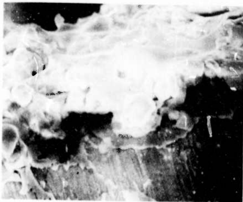
Fig. 4(a) 300 X Side View Showing Rare Earth Oxide Coating (Above) Flame Sprayed Onto Niobium Substrate.
