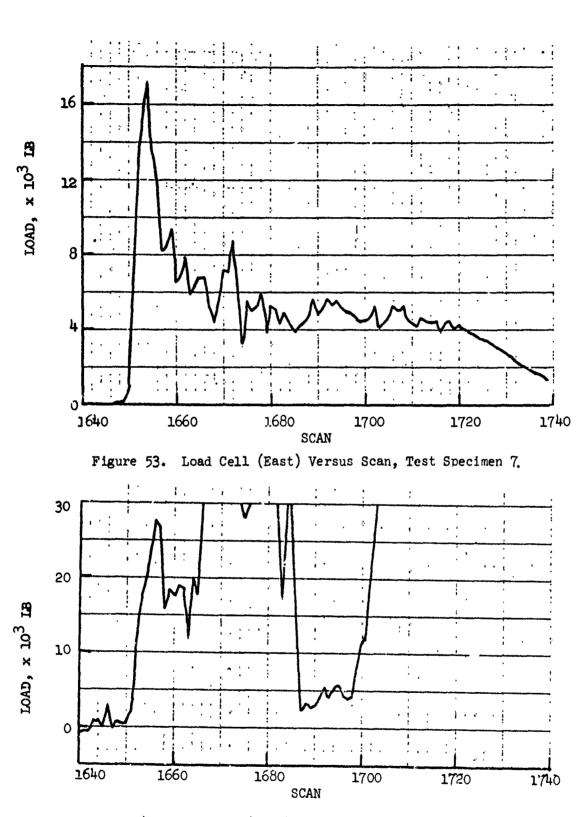
Figure 54. Load Cell (West) Versus Scan, Test Specimen 7.
