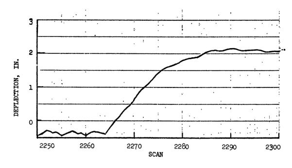
Figure 63. Deflection Versus Scan, Test Specimen 8.
