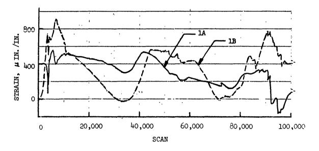
Figure 74. Strain Gages 1A and 1B Versus Scan, Test Specimen 10.
