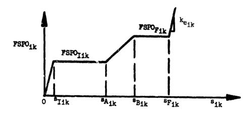
This table is defined by six parameters S<sub>Iik</sub>, S<sub>Aik</sub>, S<sub>Bik</sub>, S<sub>Fik</sub>, FSPO<sub>Iik</sub>, and FSPO<sub>Fik</sub>, which are input on cards 0801 through 080p.
