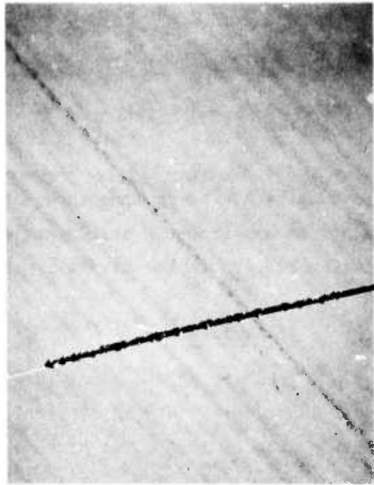
(b) Heavy growth of precipitates and bubbles along a stria. (80X)
