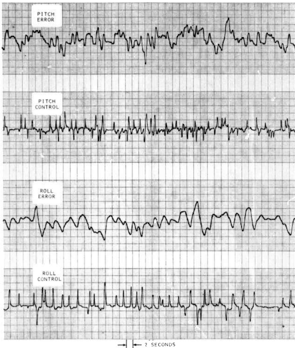
Figure 3.6 Time Histories of Error and Control Signals. Subject RF; Task = Pitch+Roll Relative Input Amplitude = 0.25
