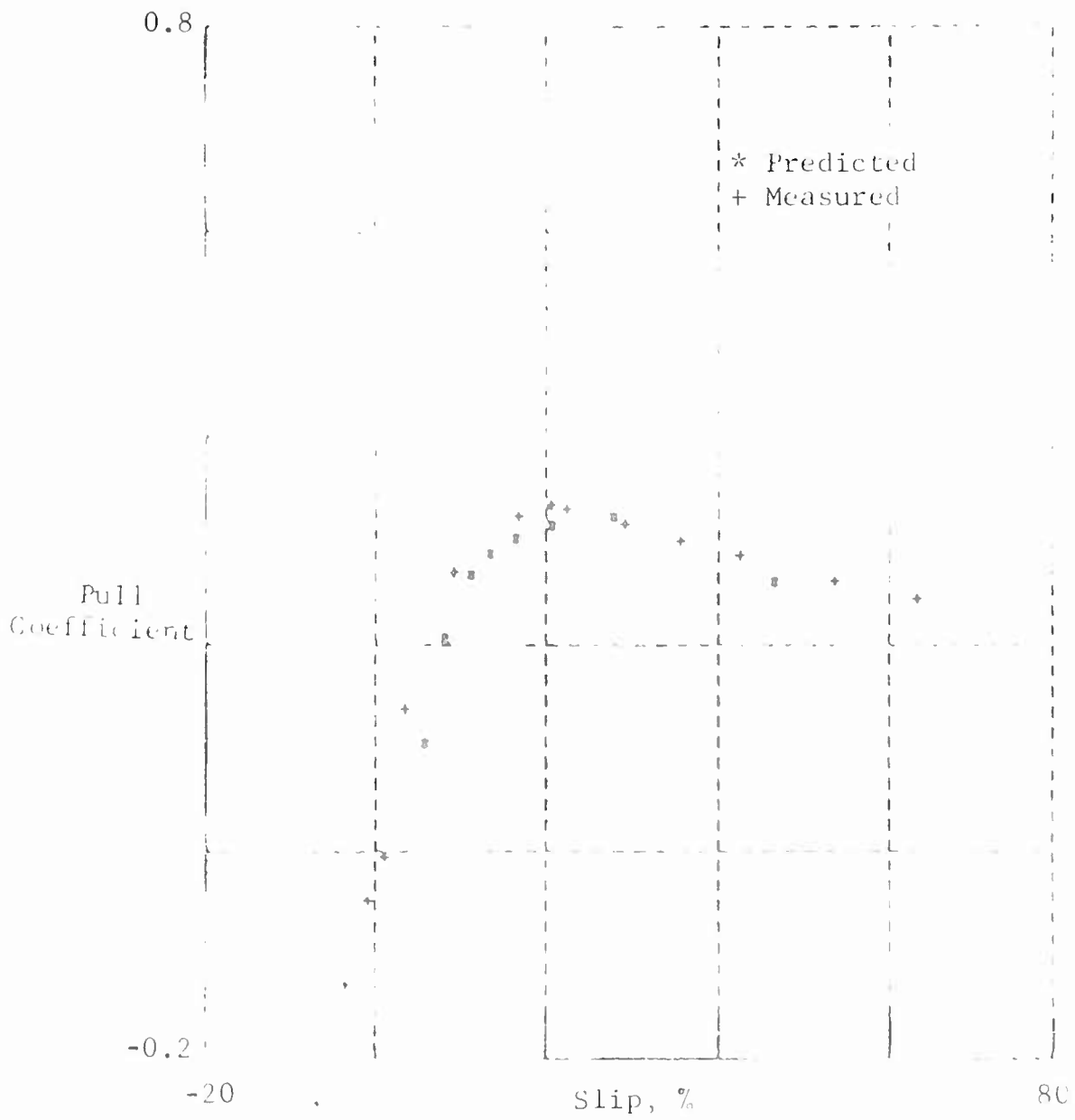
Fig. 29 Pull Coefficient Versus Slip - Test 20 Yuma Sand, CGR = 16.4 Tire: 4.00-20, Load: 440 lb
