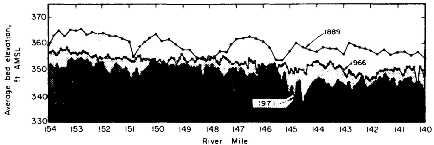
FIGURE 4 BED ELEVATIONS MILES 140 TO 154
