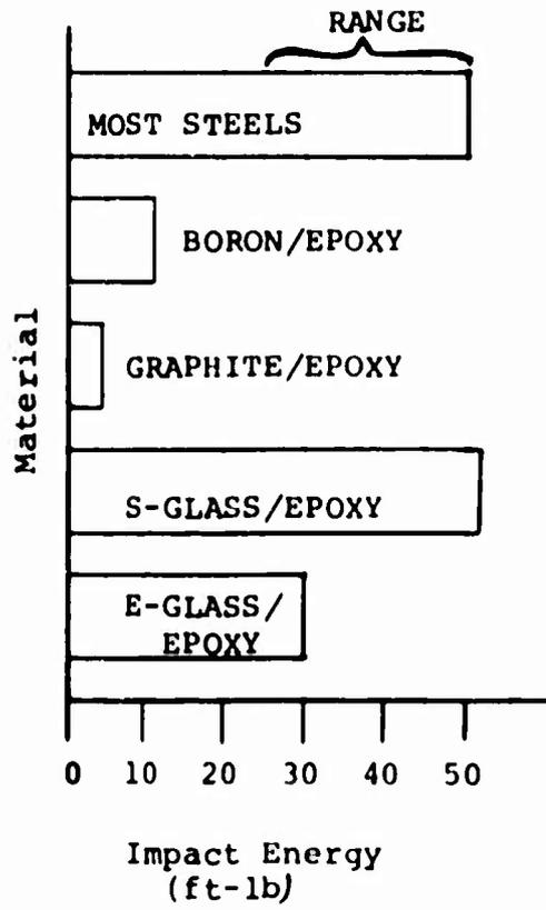
Figure 20. Fracture Toughness (Reference 5).
