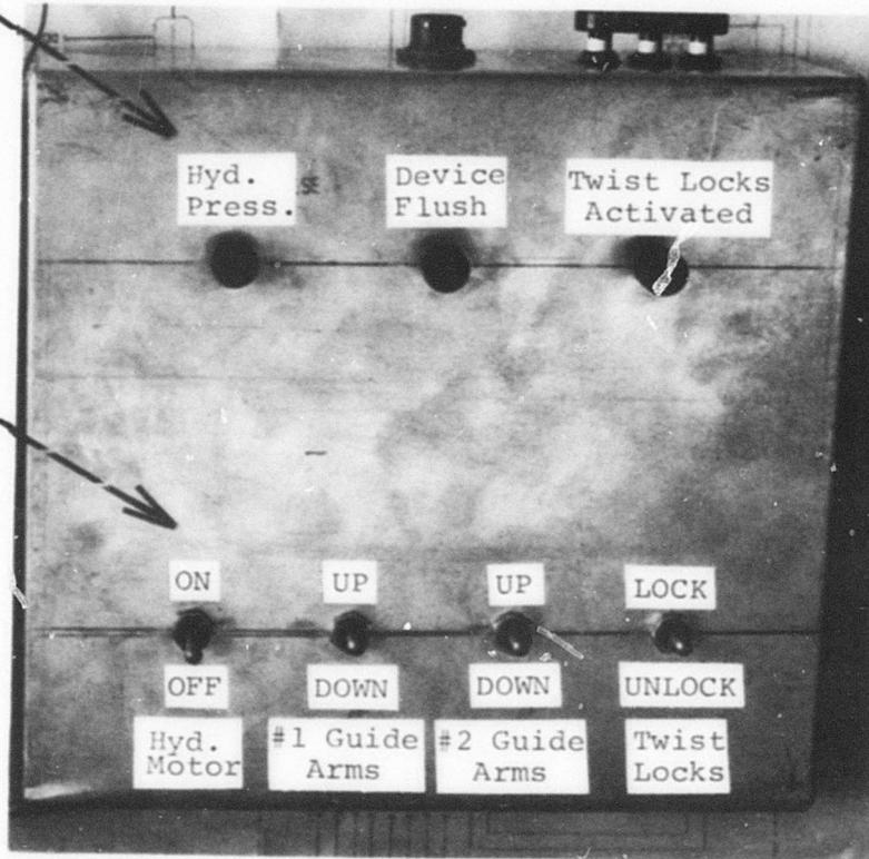
Figure 9. Helicopter Control Box.
