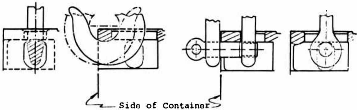
Figure 23. Hook and Shackle Attachments Protruding Beyond Side of Container.
