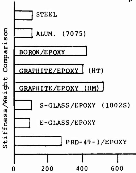
Specific Tensile Modulus,  $\frac{E_T}{\rho} - \frac{\text{PSI}}{\text{LB/CU IN.}} \times 10^6$
