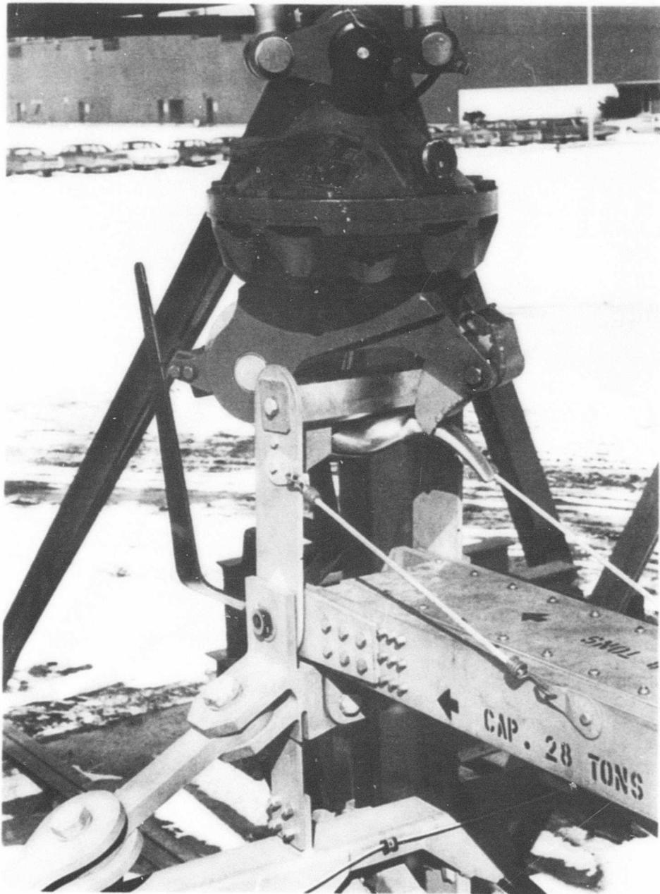
Figure 12. Closeup of HLH Cargo Coupling Attached to Dual-Mode Shackle.
