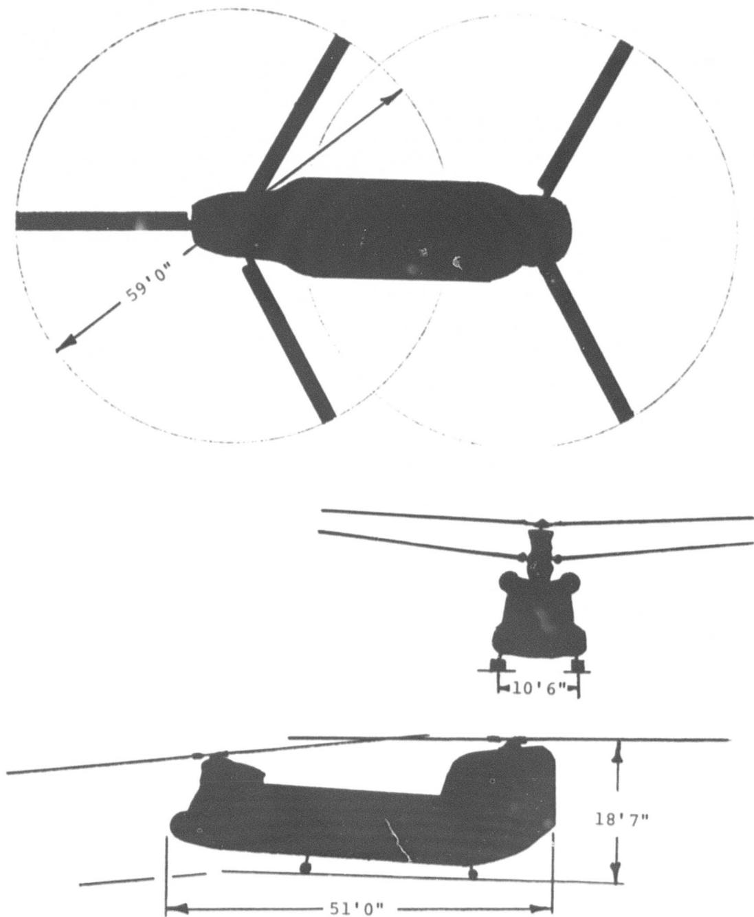
Figure 29. Container Handling Device Compatibility with CH-47.
