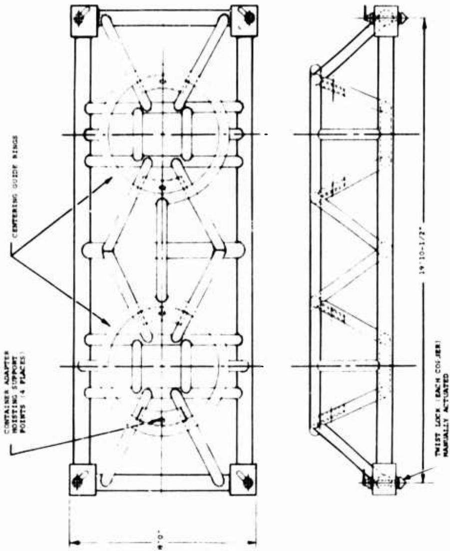
Figure 38. Container Handling Device - Cooperative Container Adapter.
