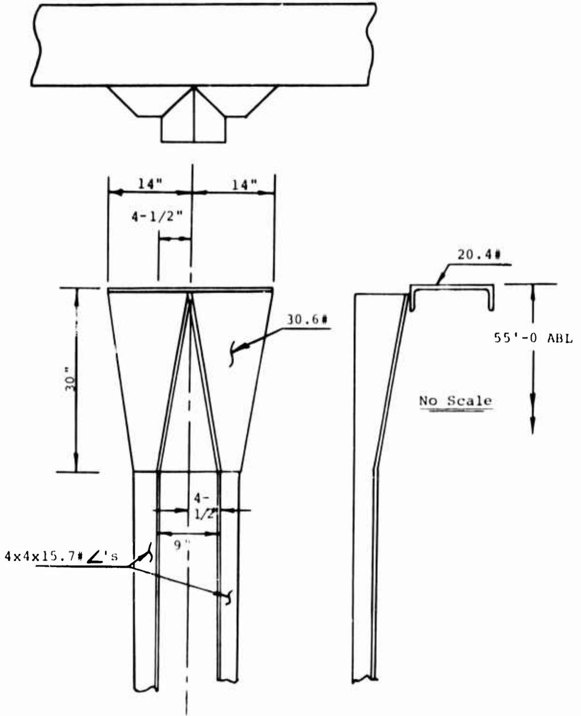
Figure 26. Existing Cell Guide Taper (Reference 3).
