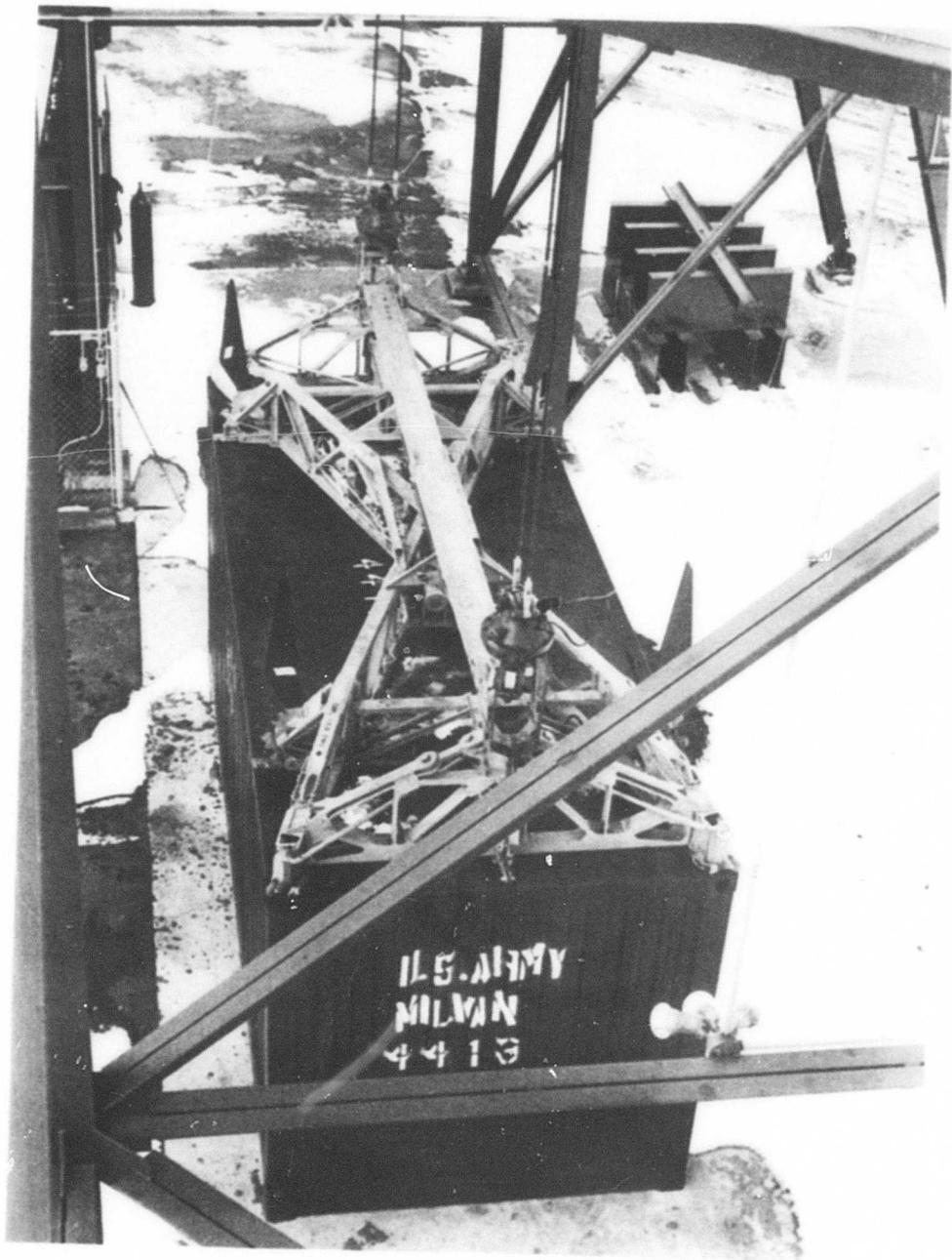
Figure 11. Container Device During HLH Compatibility Testing.
