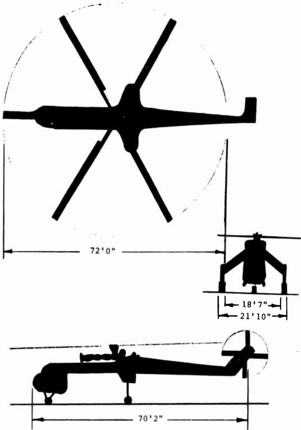
Figure 30. Container Handling Device Compatibility with CH-54.
