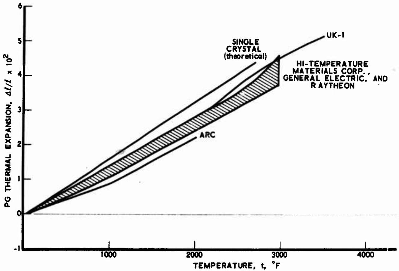
Fig. 34. C Axis Thermal Expansion vs Temperature
