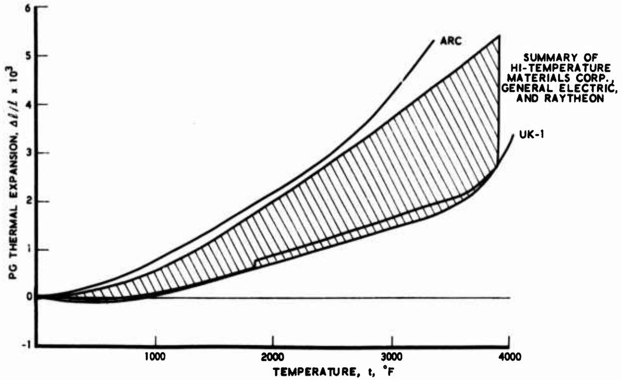
Fig. 33. Thermal Expansion of a-b Plane vs Temperature
