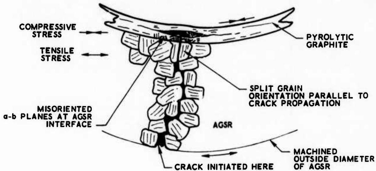
Fig. 12. Schematic of Insert Failure Region
