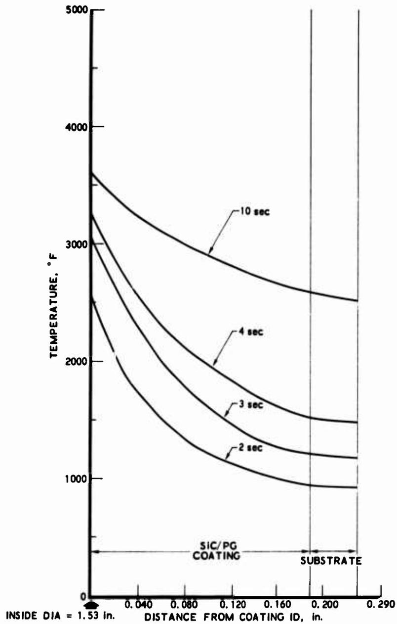
Fig. 41. Temperature Profile on C<sub>0</sub> Specimen No. 8
