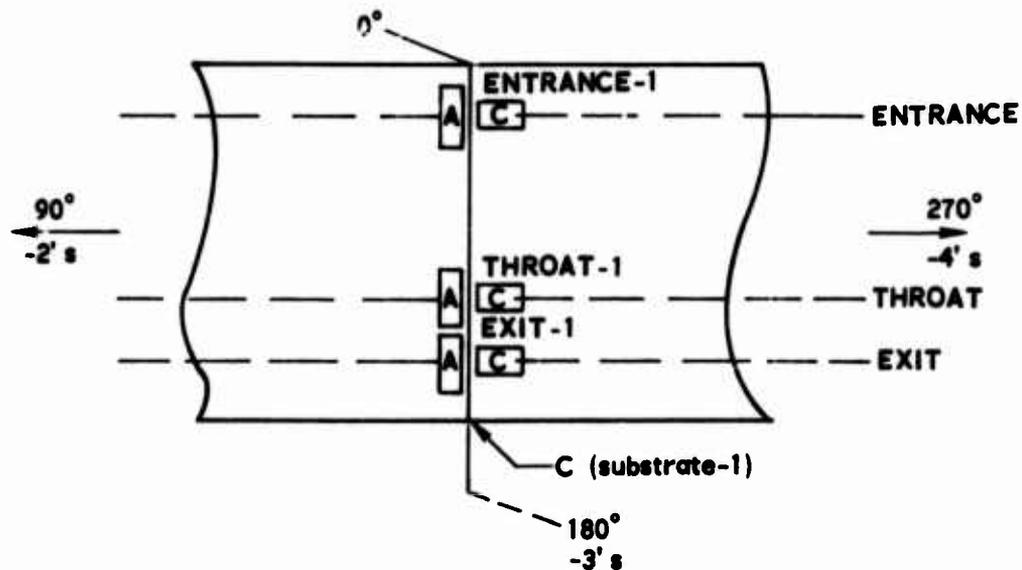
Fig. 2. Front View of Throat Insert for a Pyrolytic Graphite Coated Nozzle Showing Strain Gage Positions
