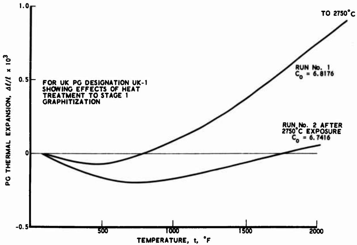
Fig. 35. Thermal Expansion of a-b Plane vs Temperature for As-Deposited and Stage I Graphitized UK PG
