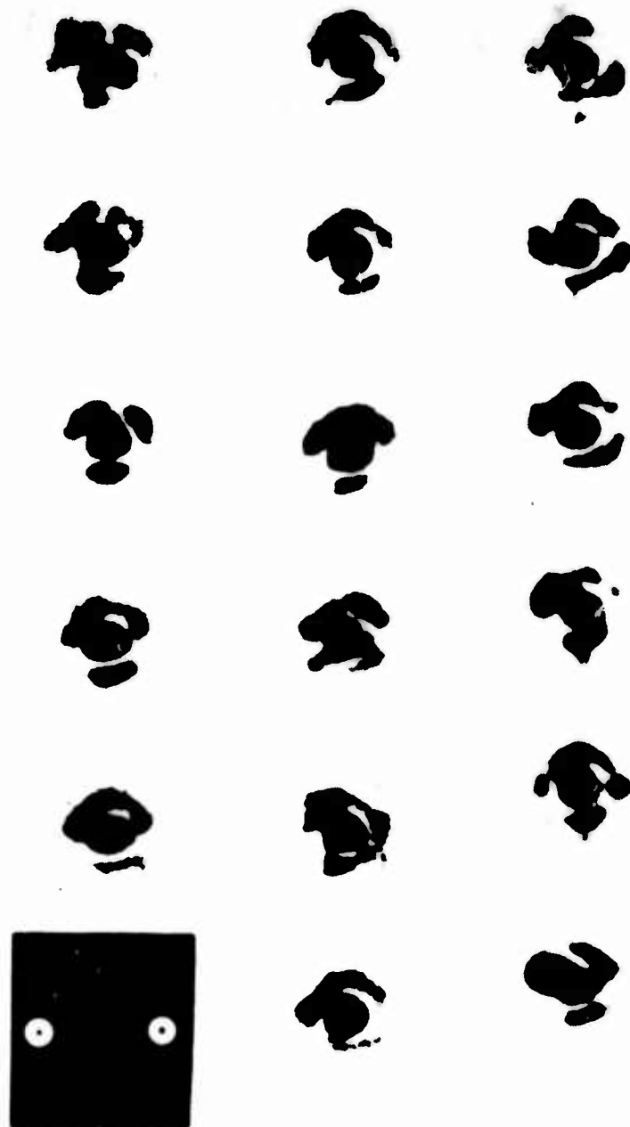
Characteristic received beam for a focused, near-field transmitter in moderate turbulence. The duration of each frame was 4 ms; the time between adjacent frames was 21 ms. The frame sequence is downward in each column, and the scale marks represent 2.5 cm. \lambda = 4880 \text{ \AA} , L = 1.4 \text{ km} , D_T = 15 \text{ cm} , \alpha_1 L = 0.09 .
