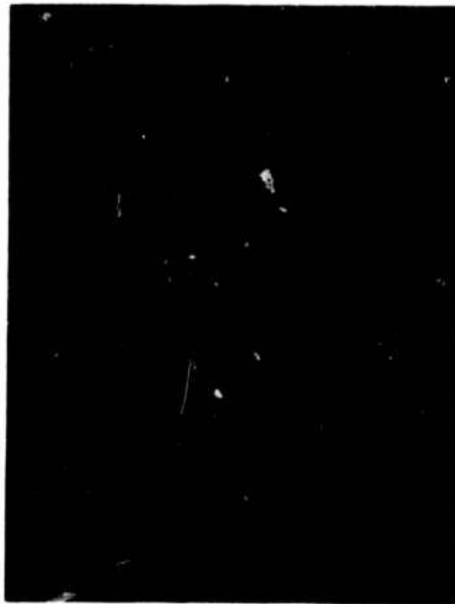
Received beam for the focused, near field transmitter of Fig. 1 in strong turbulence. Individual patches have the same nominal size as the central spot in Fig. 1.
