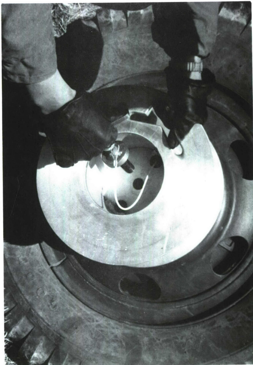
Figure 4. Installing Capstan on M35.
