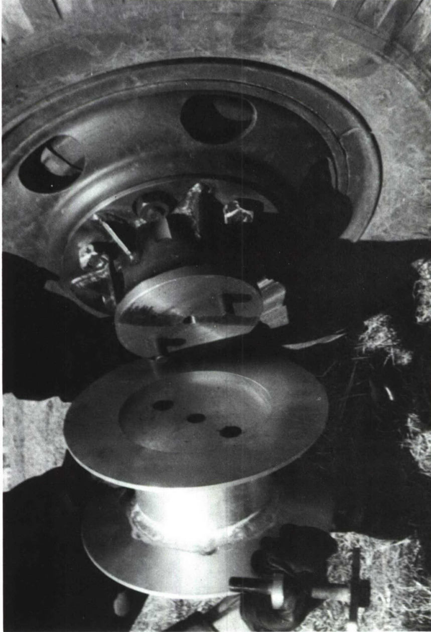
Figure 3. Wheel Adaptor (front) and Capstan for M35 Truck
