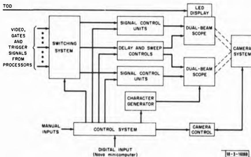
Fig. IV-17. Simplified block diagram of photorecording system.
