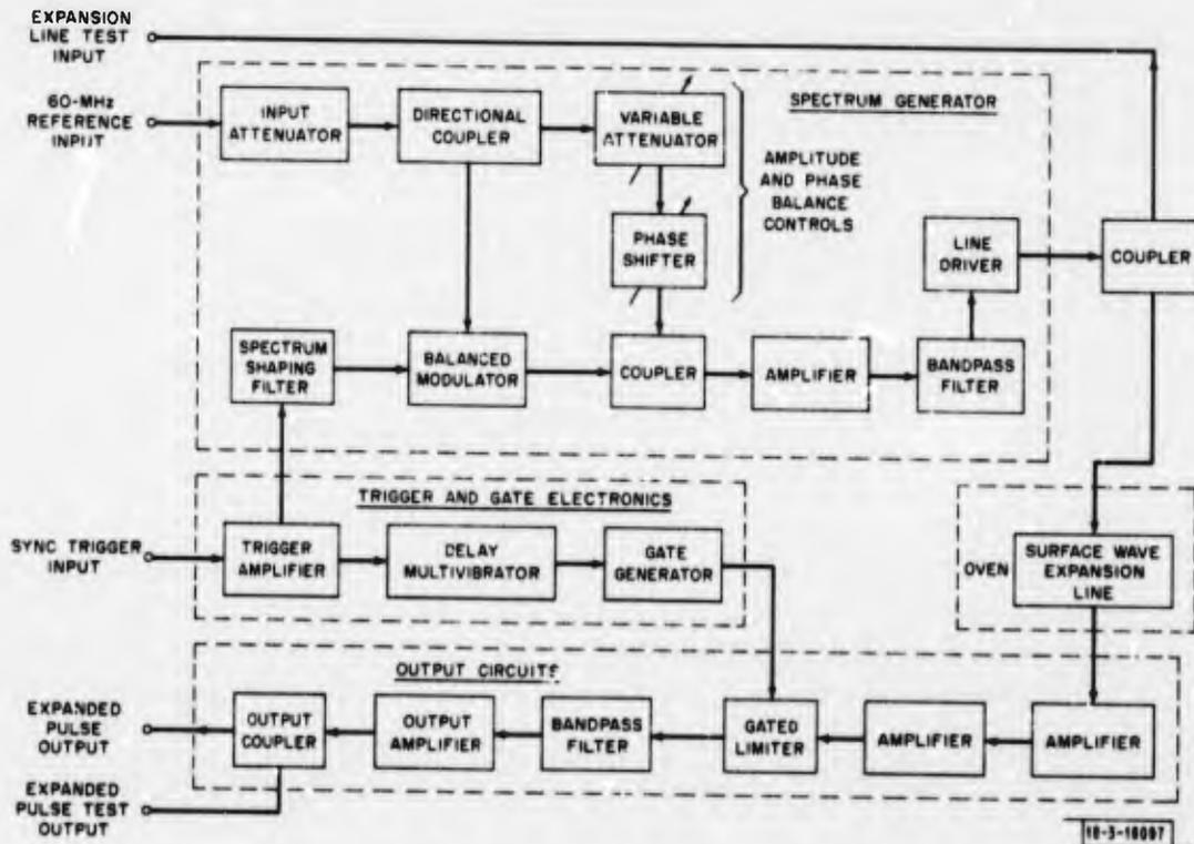
Fig. IV-27. Expansion Unit block diagram.
