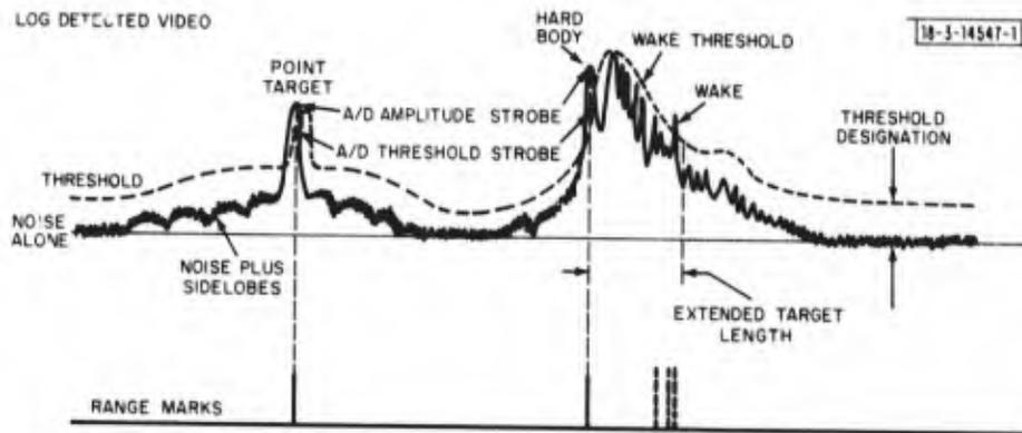
Fig. IV-4. Typical BATS received signals and measurements.
