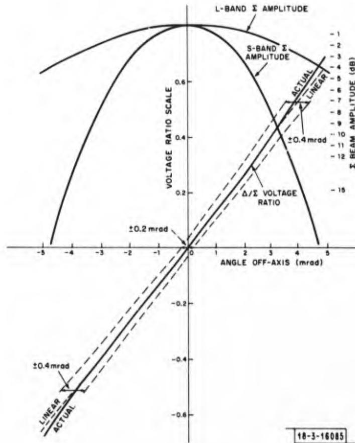
Fig. IV-13. TRADEX antenna beams and monopulse outputs.
