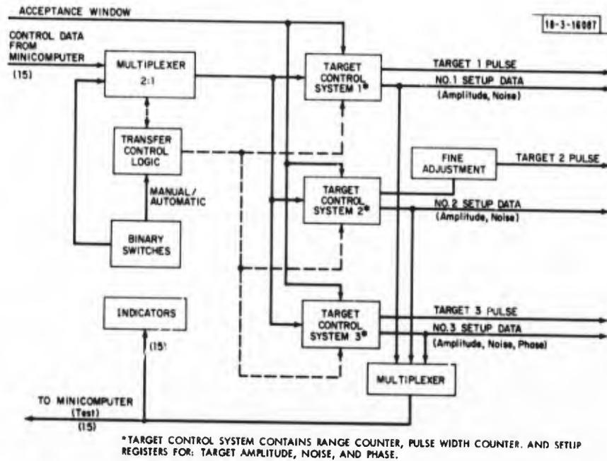
Fig. 1V-15. ATG control logic.
