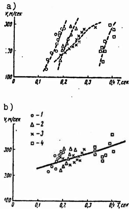
Fig. 16. Dispersive curves of the group velocities of Rayleigh's surface wave: a) not allowing for the size of the source; b) taking into account the size of the source: 1 -  $q = 20$  kg; 2 -  $q = 160$  kg; 3 -  $q = 1$  t; 4 -  $q = 10$  t.
