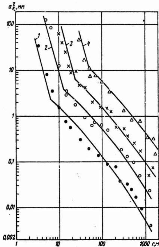
Fig. 18. Curves of dependence  $a = f(r)$  for wave R during explosions in loess deposits using charges of different force: 1 -  $q = 20 \text{ kg}$ ; 2 -  $q = 160 \text{ kg}$ ; 3 -  $q = 1 \text{ t}$ ; 4 -  $q = 10 \text{ t}$ .
