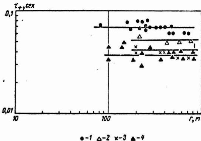
Fig. 33. Curve of the dependence of the rise time  $\tau_+$  in wave  $p$ , on the distance during explosions in loess deposits: 1 -  $q = 5000$  kg; 2 -  $q = 1000$  kg; 3 -  $q = 200$  kg; 4 -  $q = 100$  kg.
