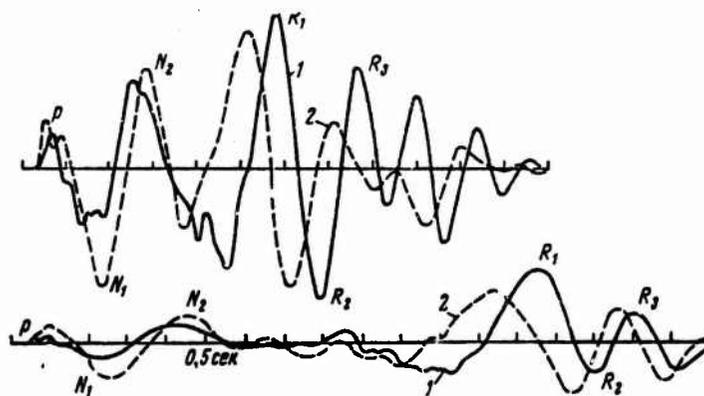
Fig. 4. Typical wave picture for two points during explosions in the media, close to a half-space: 1, 2 - vertical and horizontal (radial) components of motion; p, N, R - phases of the different waves.
