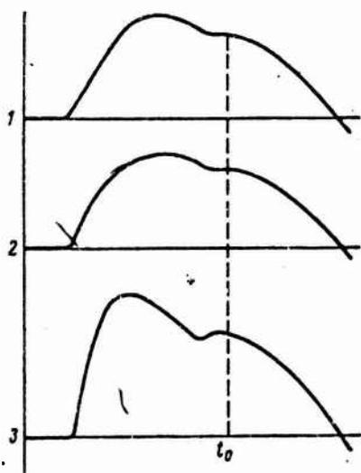
Fig. 1. Typical seismograms of the motion of the soil in the epicentral zone: 1 - at the epicenter; 2 -  $r = 0.5 h_3$ ; 3 -  $r = h_3$ .
