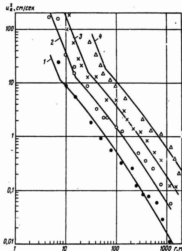
Fig. 20. Curves of dependence  $u_R = \psi(r)$  during explosions in loess deposits using charges of different force: 1 -  $q = 20$  kg; 2 -  $q = 160$  kg; 3 -  $q = 1$  t; 4 -  $q = 10$  t.
