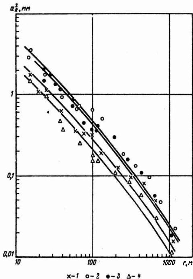
Fig. 21. Curves of the dependence of displacement into wave R, on the placement depth of the charge of 160 kg during explosions in loess deposits: 1 -  $h_3 = 1.25$  m; 2 -  $h_3 = 3.75$  m; 3 -  $h_3 = 10.4$  m; 4 -  $h_3 = 22.5$  m.
