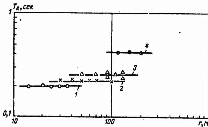
Fig. 27. Curves of dependence  $T = f(r)$  in wave R during explosions in water-saturated sands using charges of different weight: 1 -  $q = 5 \text{ kg}$ ; 2 -  $q = 10 \text{ kg}$ ; 3 -  $q = 40 \text{ kg}$ ; 4 -  $q = 320 \text{ kg}$ .
