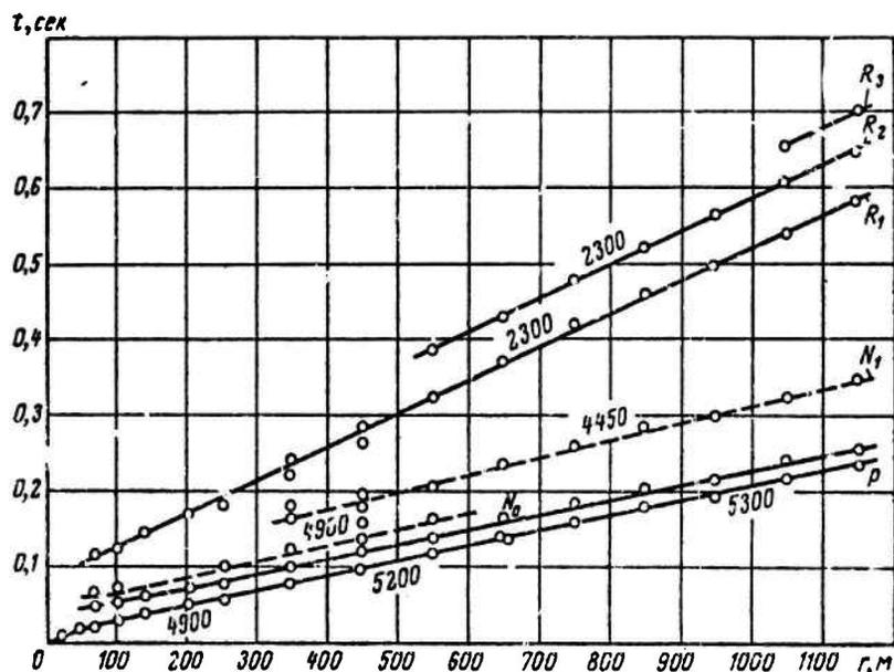
Fig. 5. Hodographs of waves during explosions in granite.
