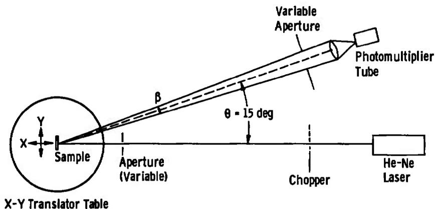
Figure 4. Schematic of uniformity-measuring apparatus.
