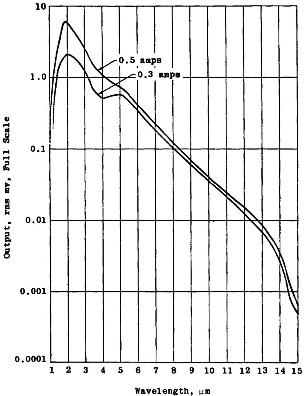
Figure 2. Spectral output of Nernst glower.
