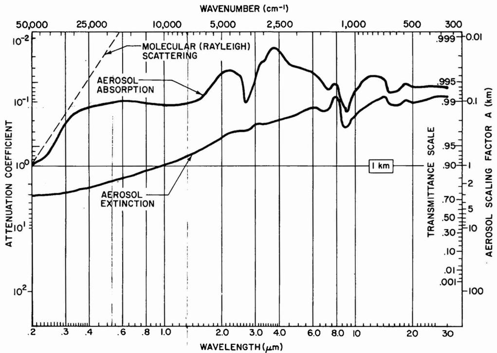
Figure 2. Attenuation Coefficients for Aerosol Transmittance (Absorption and Total Extinction)
