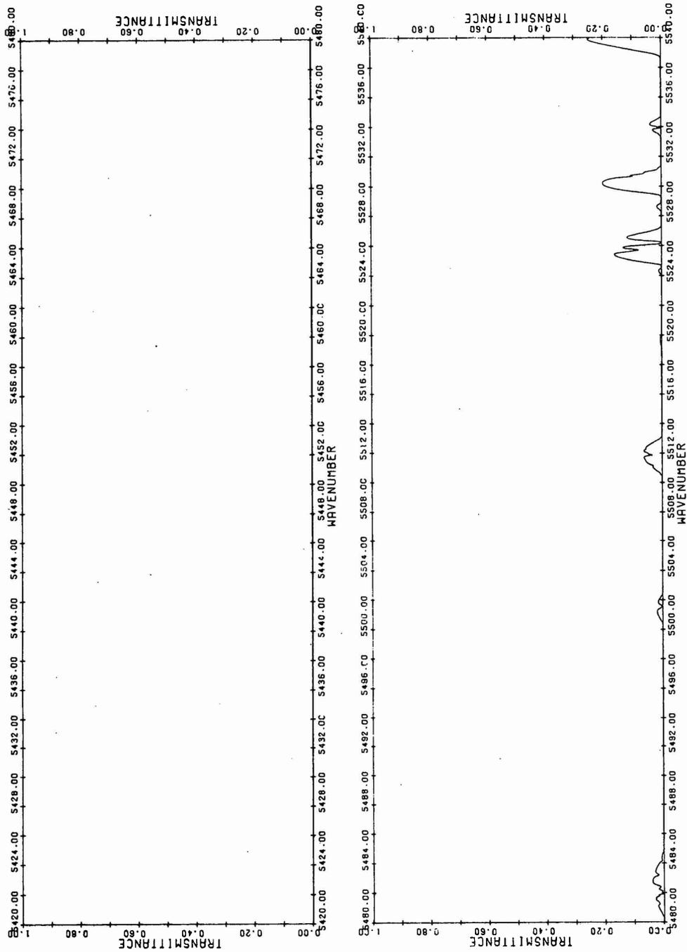
Figure 4ar. Atmospheric Transmittance due to Molecular Absorption Through a 10-km Horizontal Path at Sea Level
