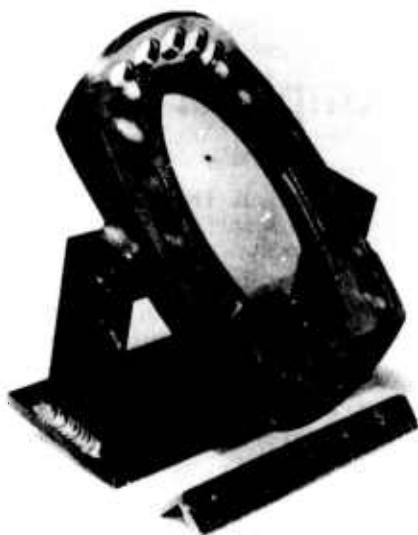
Fig. 1. Individual disk-lamp holder (scale is in inches). The disk-amplifier assembly consists of eleven of these holders placed end to end in a zigzag pattern. Twenty-two lamps each 60-in long are slid through the disk holders to completely surround the disks. Separate top and bottom reflectors are placed around the disk holders. All of the metal surfaces are gold-plated.
