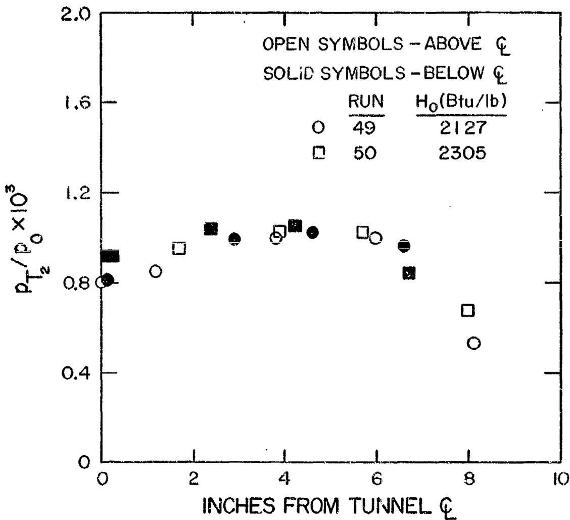
Figure 14. Pitot Pressure Surveys at Run Condition 3;
