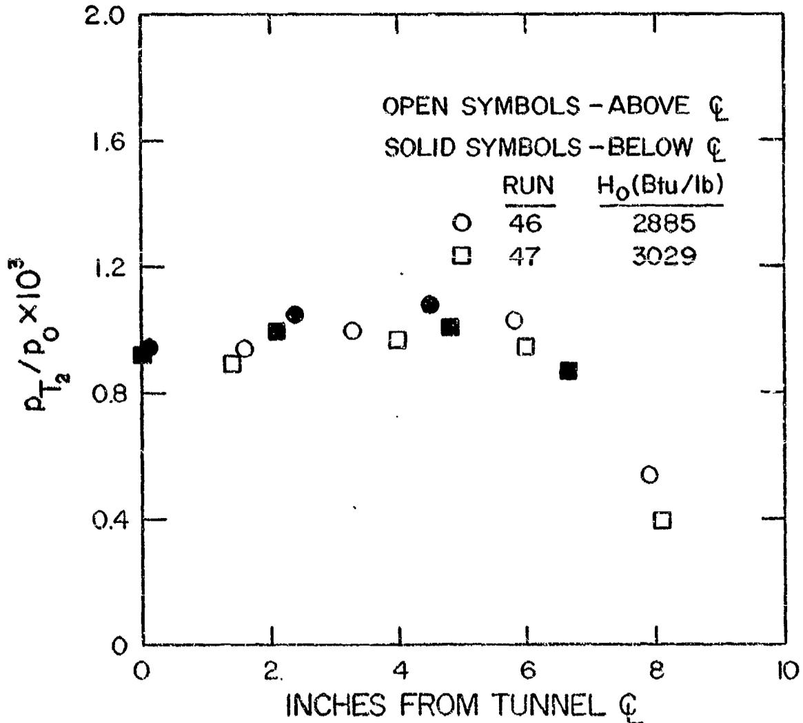
Figure 13. Pitot Pressure Surveys at Run Condition 2;
