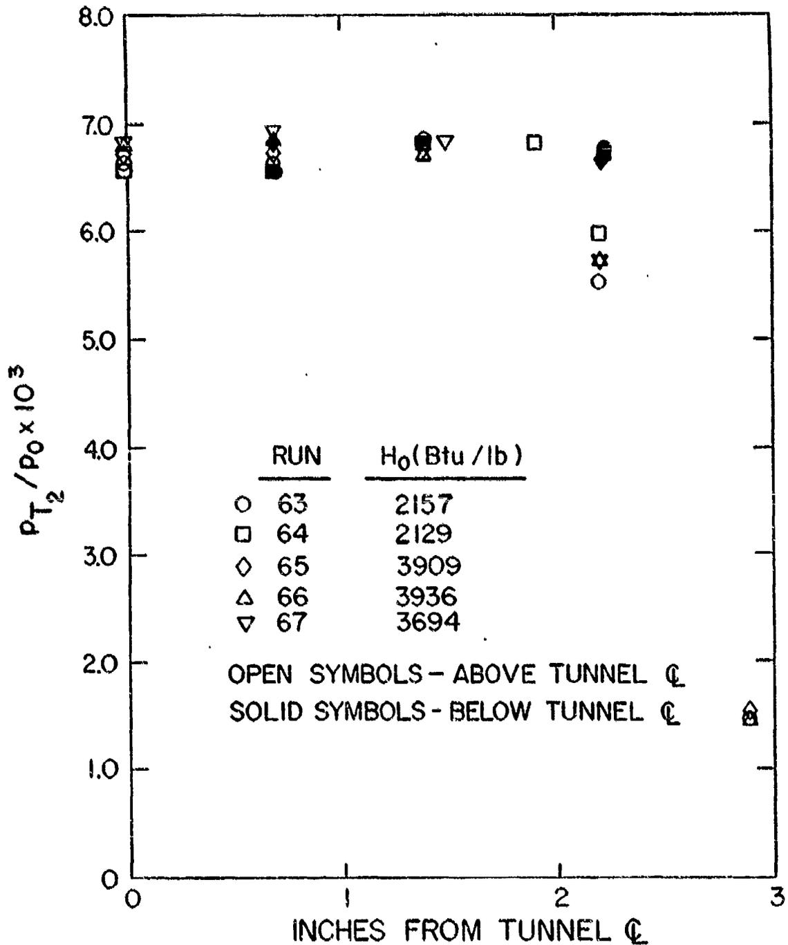
Figure 17. Pitot Pressure Surveys at Run Condition 3;
