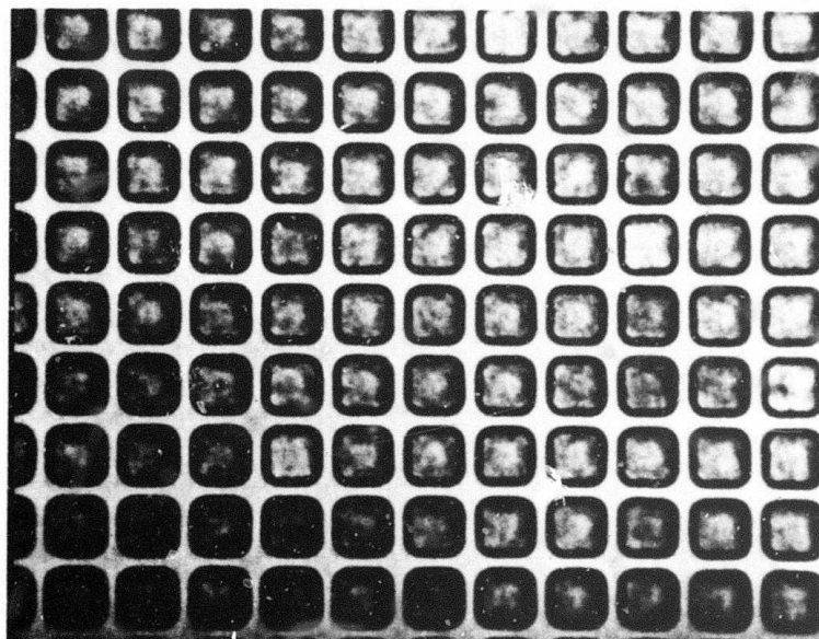
Figure 7A. Metal-Silicon Schottky Barrier Diode Array Infrared Vidicon Retina. Pd Thickness 500 Å, Magnification X1000
