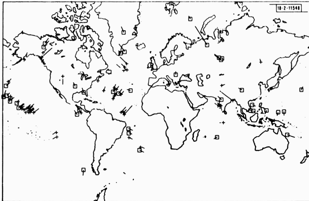
Fig. IV-10. Regional anomalies in P-wave travel times for distance range of 80^{\circ} to 90^{\circ} . Symbols are plotted at midpoint of great circle path. Crosses represent late arrivals, and squares indicate early arrivals. Straight lines are in direction of source to station azimuth, their length being proportional to travel-time anomalies. Smallest length in this figure represents an absolute value of 0.5 sec, and largest is an absolute value of 3 sec.
