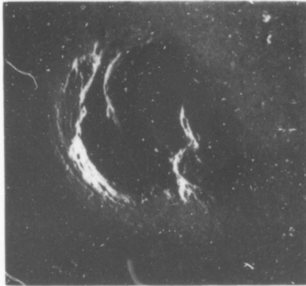
Spall morphology on a Silicon Nitride ball run in a five-ball tester. 100X
