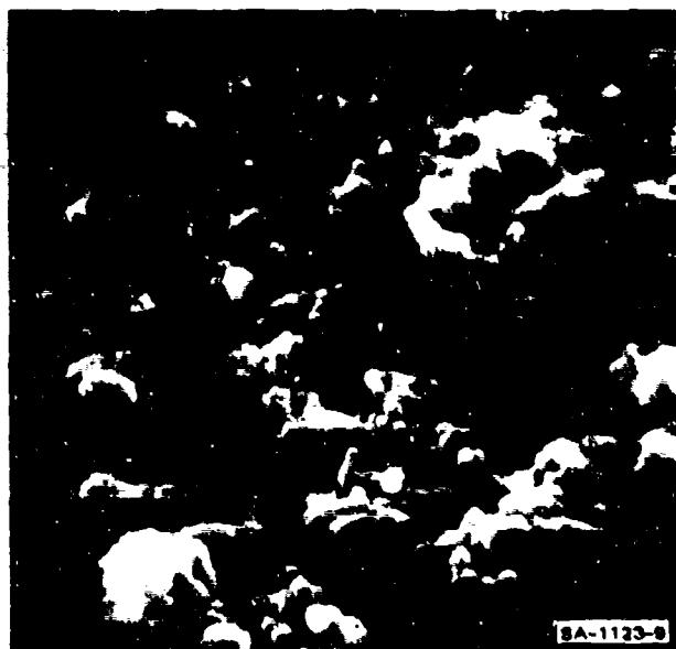
FIGURE 5 SCANNING ELECTRON MICROGRAPH OF MgAl_2O_4 POWDER OBTAINED BY CALCINING A MIXTURE OF HYDRATED AMMONIUM ALUMINUM SULFATE AND HYDRATED MAGNESIUM NITRATE SALES (X20,000)
