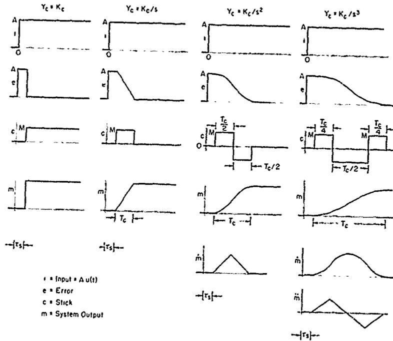
Figure 45. Ideal Time-Optimal Response Characteristics
