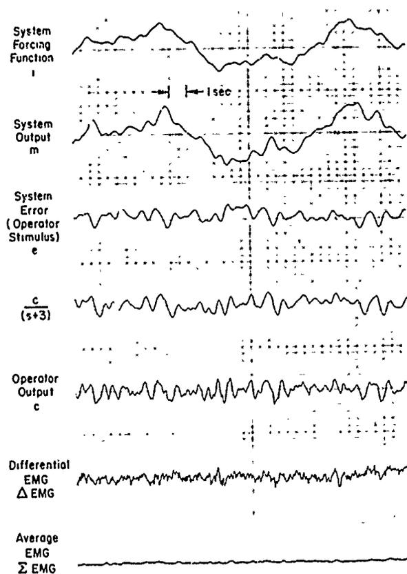
Figure 7. Man/Machine System Response Time Histories;  $Y_C = K_C/[s(s/3 + 1)]$
