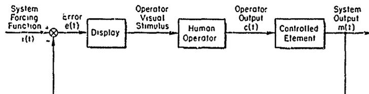
Figure 1. Display and Functional Block Diagram of
