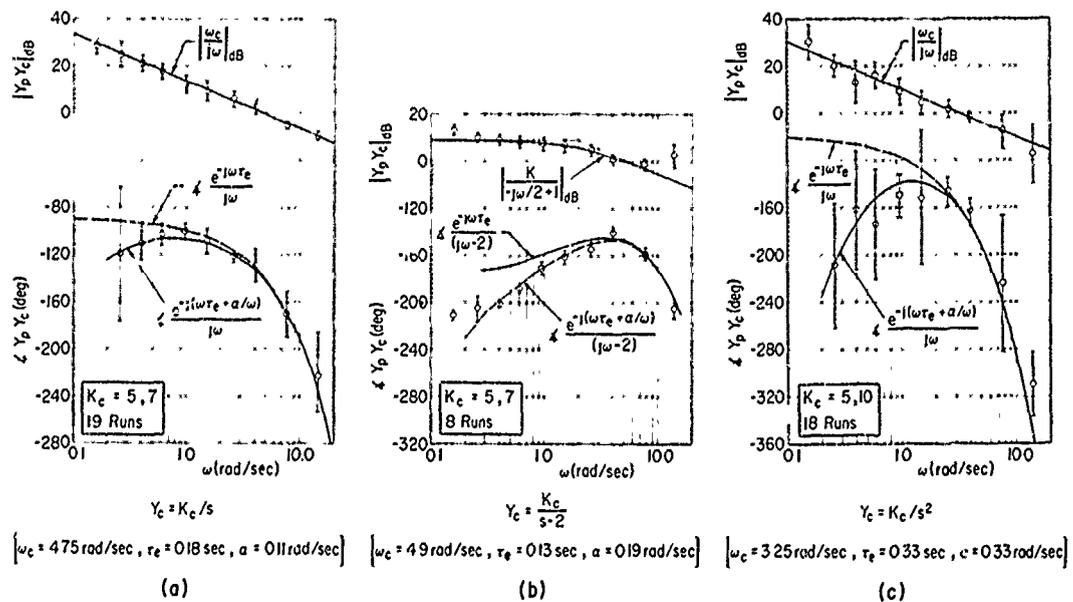
Figure 18. Data, Simple Crossover Models, and  $\alpha$  Crossover Models for Elementary Controlled Elements;  $\omega_1 = 2.5 \text{ rad/sec}$  (Ref. 56)
