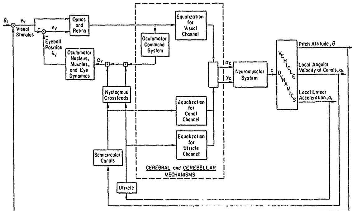
Figure 3<sup>h</sup>. Pilot/Vehicle System for Head-Fixed, Pressure-Manipulator, Attitude Control Tasks
