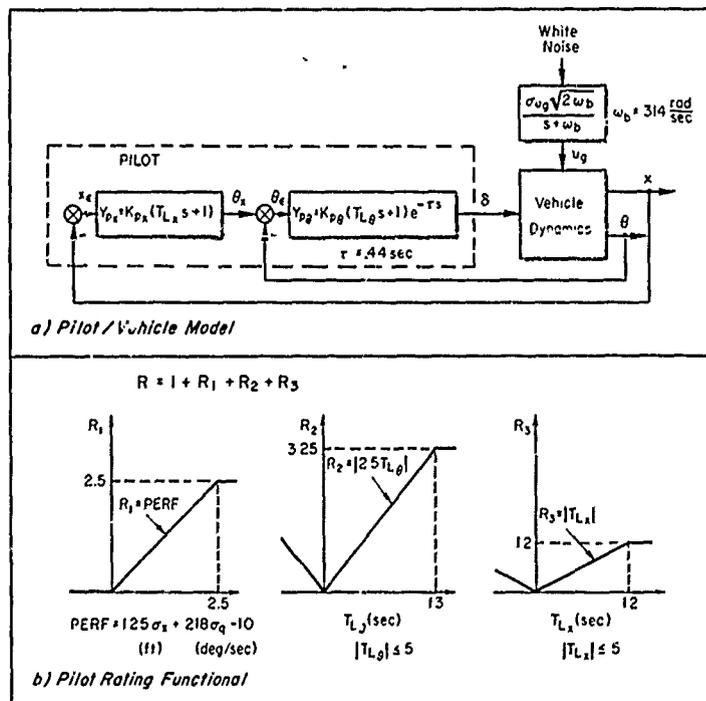
Figure 26. Typical Pilot/Vehicle Model and Form of Pilot Rating Functional (Specific Values for Hover Task, Refs. 96-97) (Refs. 5-6)
