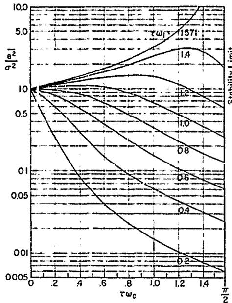
Figure 12. Crossover Model Steady-State Performance for Inputs with Rectangular Spectral Densities
