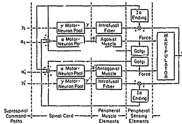
Figure 16. Functional Diagram of Elemental Agonist/Antagonist Neuromuscular System Elements Involved in Tracking
