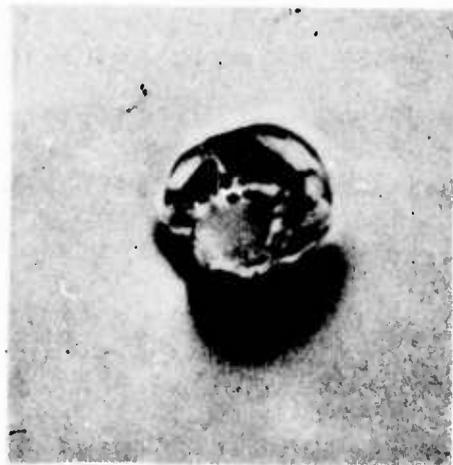
**Fig. 11d.** X-ray topograph of fracture cone corresponding to Fig. 11b (approx. 10X).
