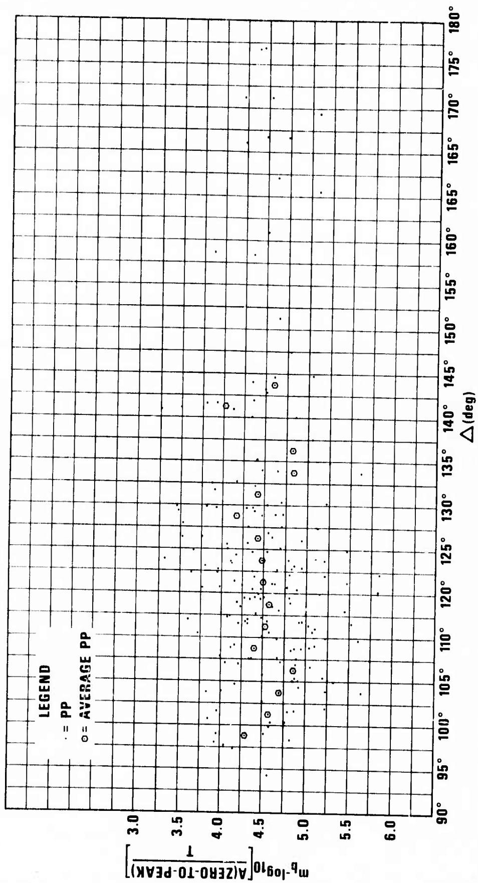
Figure 8. Individual amplitude versus distance values for PP from Observatory and LRSM readings ( $0^\circ$ - $180^\circ$ ) 18 July 1963 - 31 October 1968.
