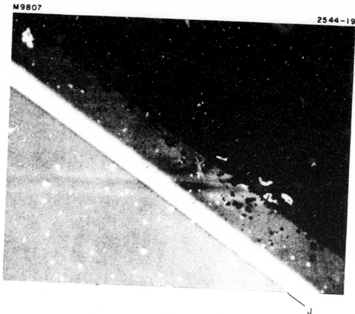
Fig. 18(a). SEM photograph of cleaved cross section of A 4 . Magni- fication 500x.
