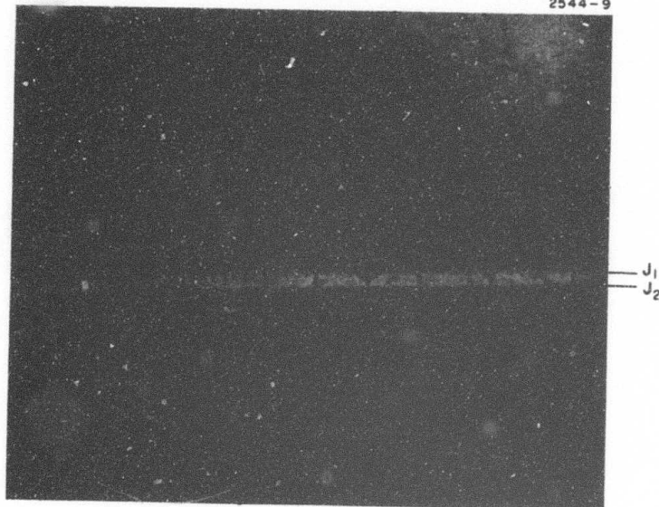
Fig. 9. Ga 0.95 Al 0.05 As layer on GaAs. Note the regrowth region J 1 J 2 . Scale: 2.3 μm/div.
