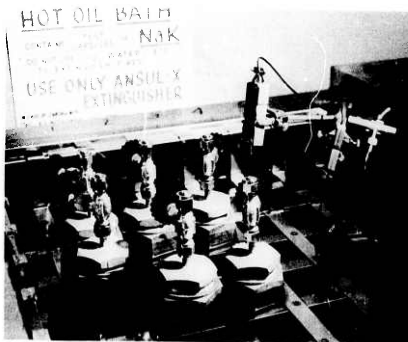
(b) View of material test canisters in oil bath
