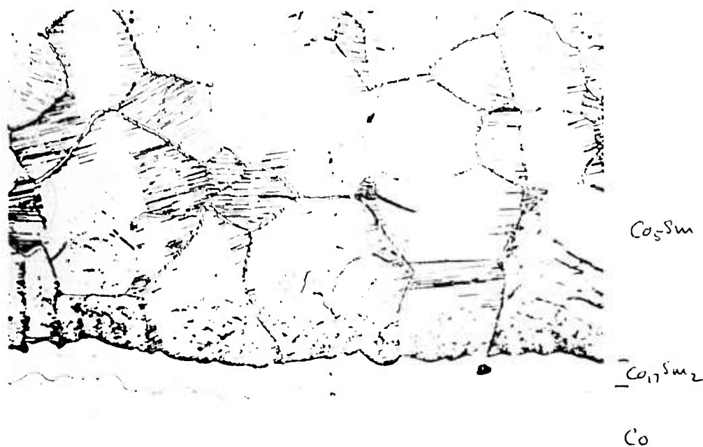
Figure 15 Cobalt + 60 wt % Sm alloy diffused 15 hours at 1120°C and then heat treated for 206 hours at 700°C. 228X
