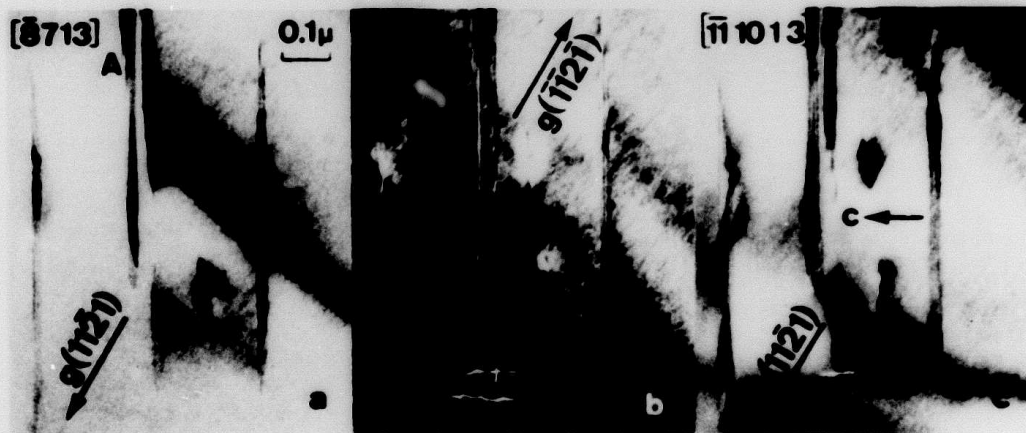
Fig. 1 Bright (a and c) and dark field (b) images of \text{Co}_5\text{Sm} showing the existence of basal stacking faults.
