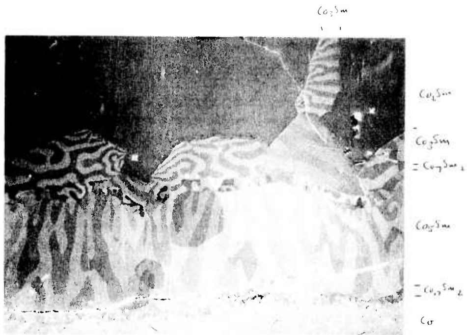
Figure 14 Cobalt + 60 wt % Sm alloy diffused 1 hour at 1120°C. Polarized light. 525X
