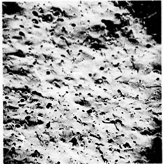
Fig. 7 Sample A showing intergranular fracture. 500X
