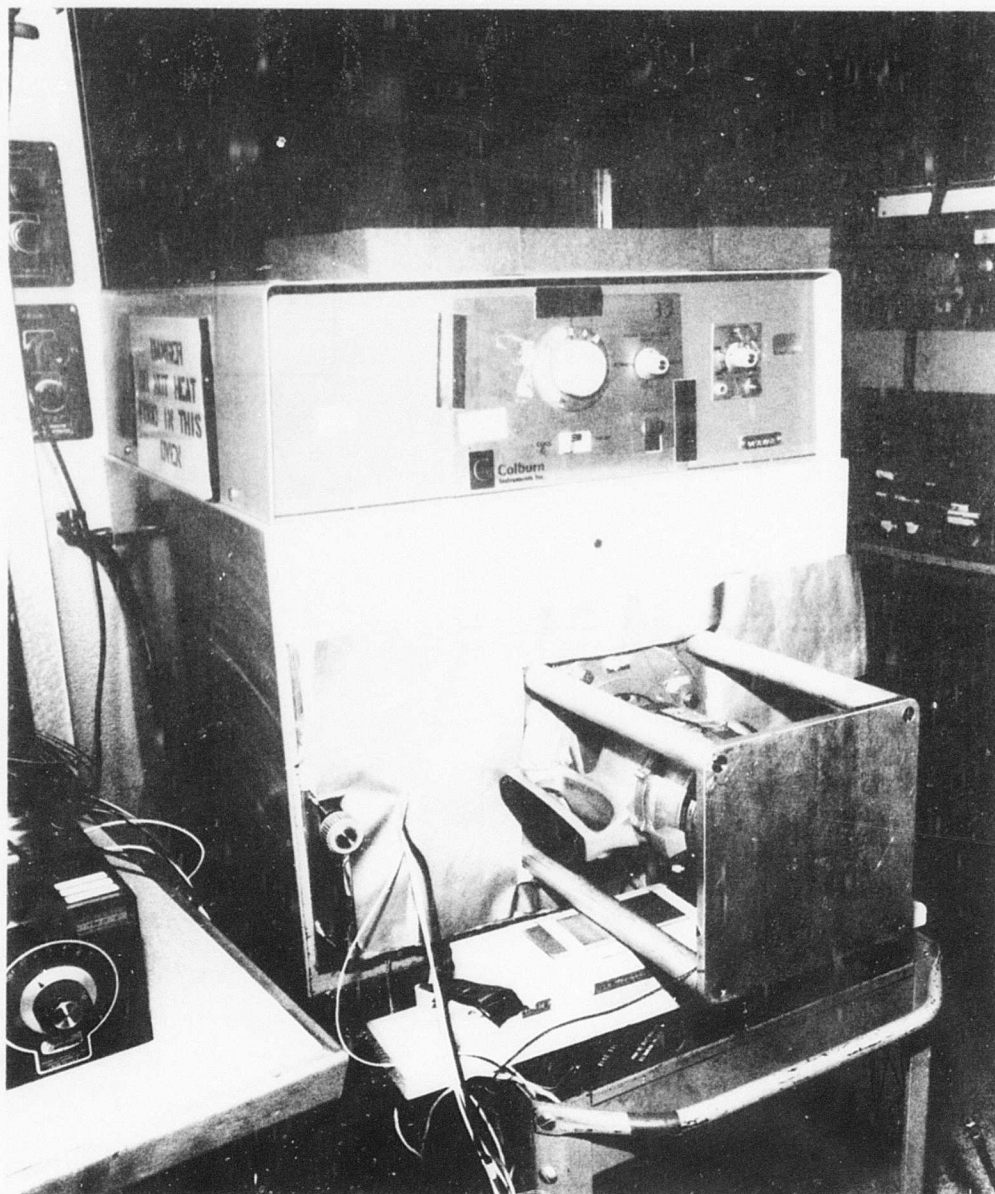
Figure 72. Installation of Test Sensing Unit in Colburn Oven.
