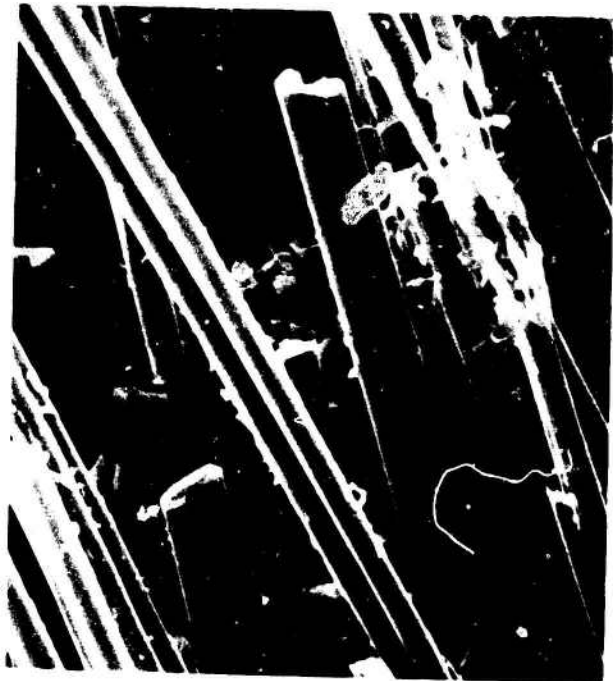
Figure 6. AZ91C Mg-Graphite fiber composite, good area (fractured)
