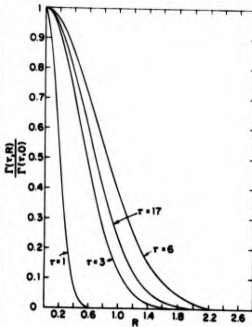
Figure 3. Normalized Mutual Coherence Function for a Beam With  $C_s = 100$ ,  $C_F = -\infty$ ,  $\lambda = 0.001$
