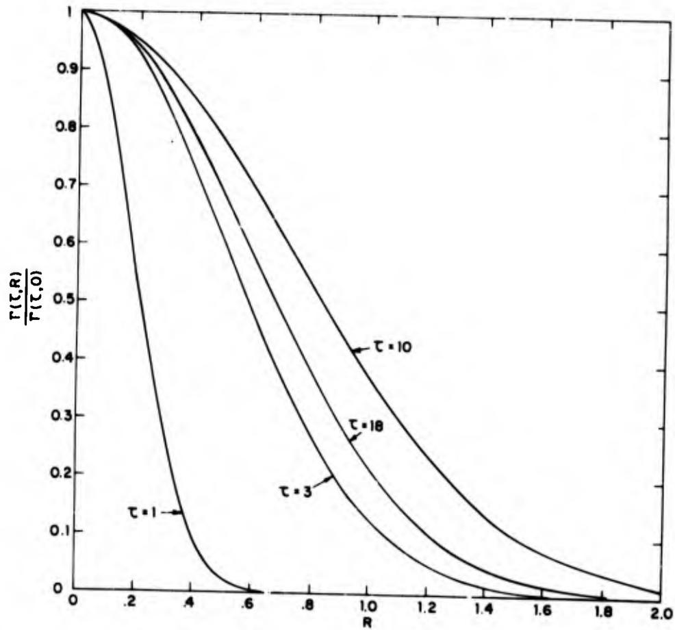
Figure 4. Normalized Mutual Coherence Function for a Beam With  $C_S = 100$ ,  $\lambda = 0.01$ ,  $C_F = -\infty$
