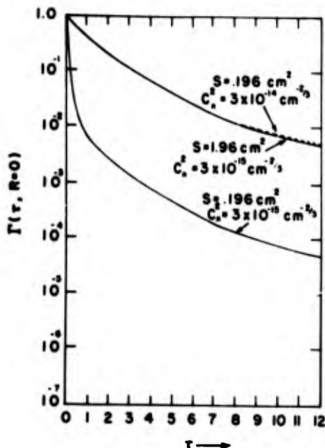
Figure 8. Axial Intensity for a Laser Beam Propagating in Turbulence Having a von Karman Spectrum, Assuming  $k_0 = 6280 \text{ cm}^{-1}$  and  $F = -\infty$
