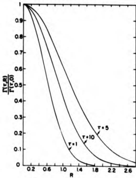
Figure 2. Normalized Mutual Coherence Function for a Beam With  $C_s = 10$ ,  $C_F = -\infty$ ,  $\lambda = 0.001$
