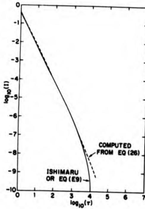
Figure E1. Comparison of Axial Intensity for a von Karman Spectrum Assuming  $k_0 = 6280 \text{ cm}^{-1}$ ,  $C_n^2 = 3 \times 10^{-14} \text{ cm}^{-2/3}$ ,  $S = 0.196 \text{ cm}^2$ , and  $F = -\infty$
