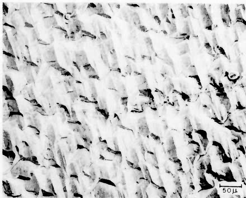
Figure 4.19 Typical faceted surface developed in GaN grown on (1\bar{1}02) -sapphire.
