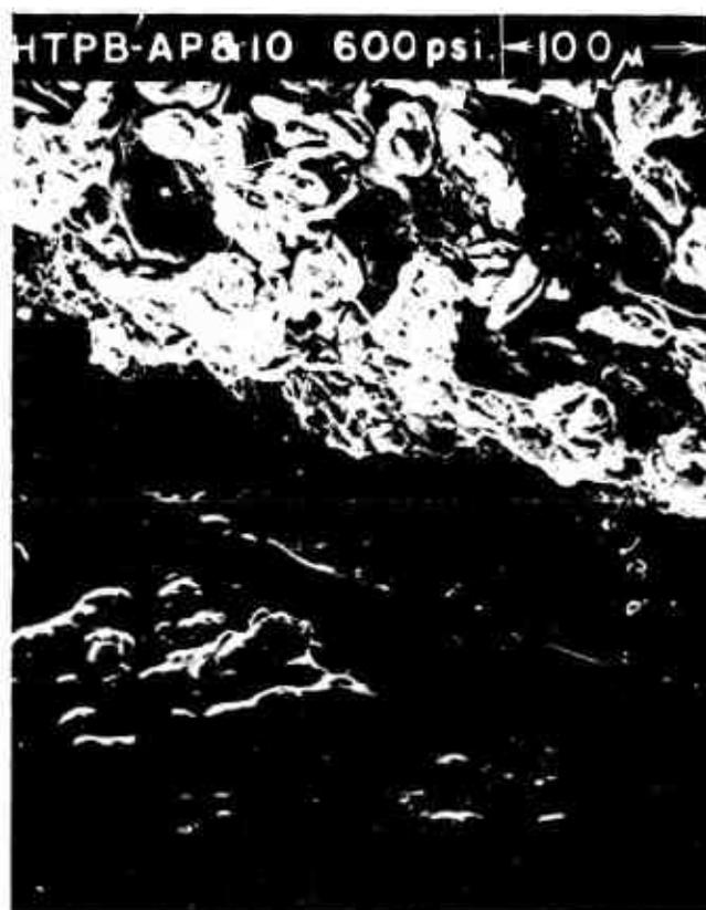
Figure III-24. HTPB-AP and Ferric Oxide (IO) 600 psia (x260).
