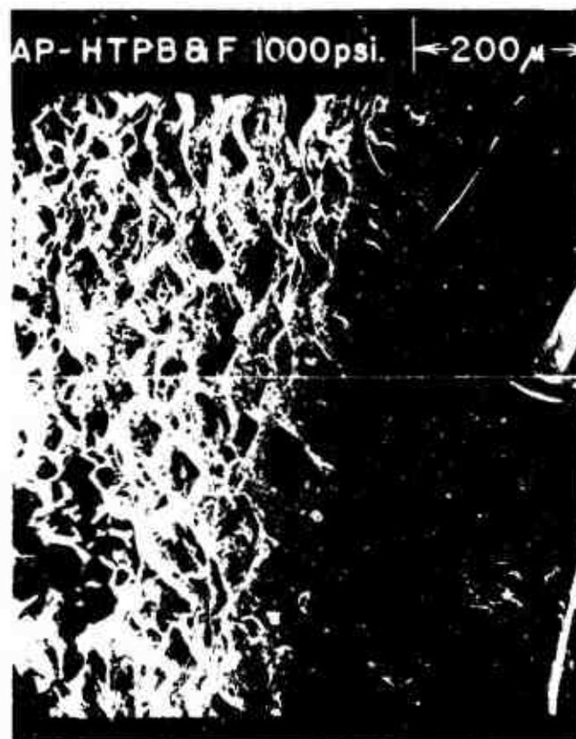
Figure III-72. AP-HTPB and Ferrocene (F) 1000 psia (x140).
