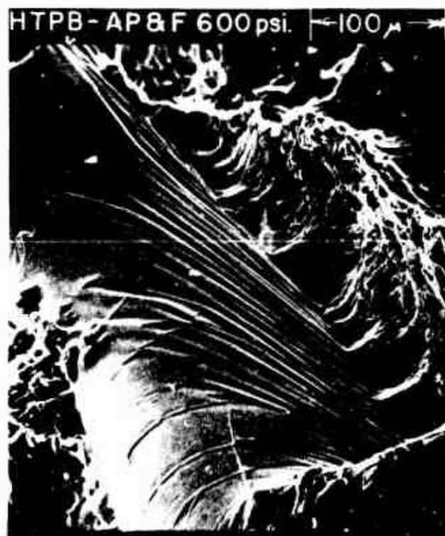
Figure III-36. HTPB-AP and Ferrocene (F) 600 psia (x262).
