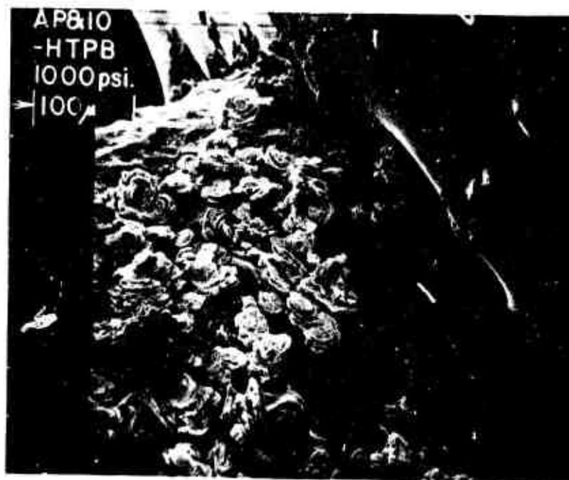
Figure III-27. AP and Ferric Oxide (IO)-HTPB 1000 psia (x204).
