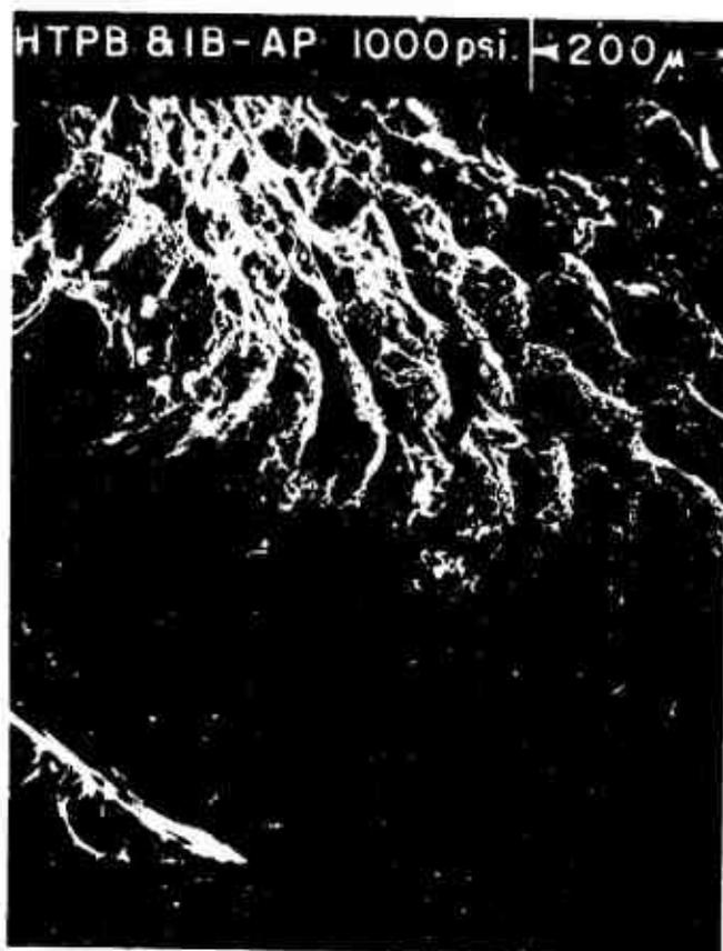
Figure III-73. HTPB and Iron Blue (IB)-AP 1000 psia (x130).
