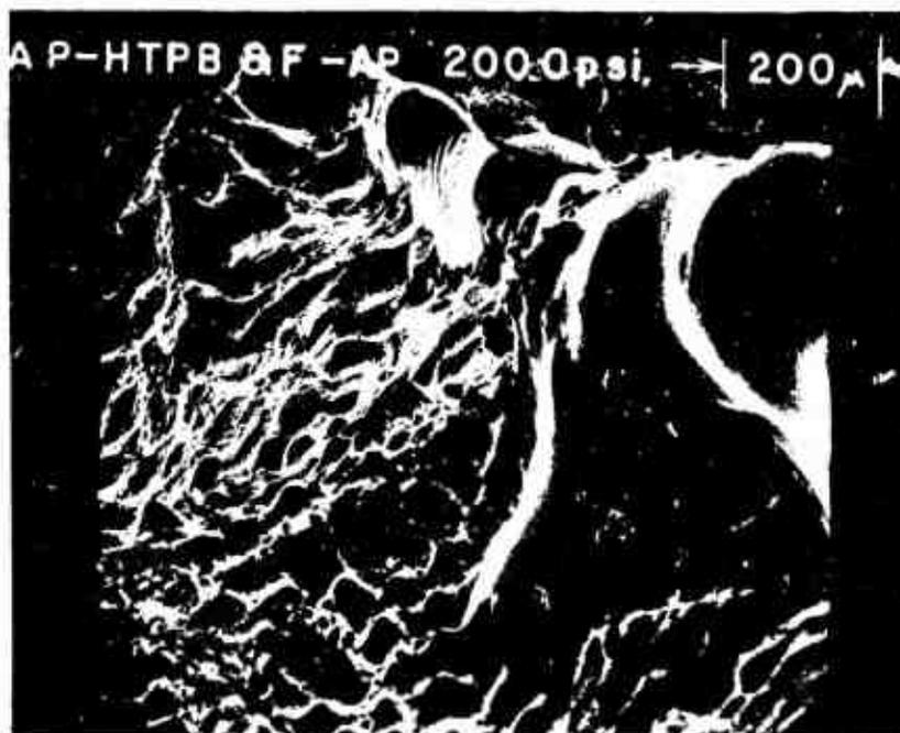
Figure III-78. AP-HTPB and Ferrocene 2000 psia (x98).
