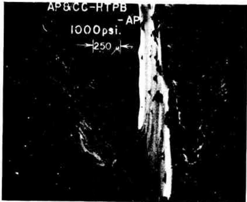
Figure III-18. AP and CuO<sub>2</sub> (CC)-HTPB-AP 1000 psia (x49.3).
