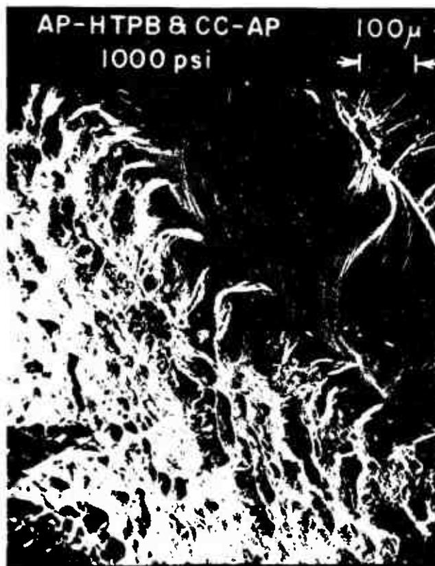
Figure III-57. AP-HTPB and CuO<sub>2</sub>O<sub>2</sub> (CC)-AP 1000 psia (x116).
