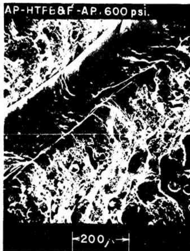
Figure III-66. AP-HTPB and Ferrocene (F)-AP 600 psia (x135).
