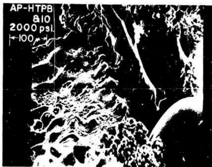
Figure III-64. AP-HTPB and Ferric Oxide (IO) 2000 psia (x200).
