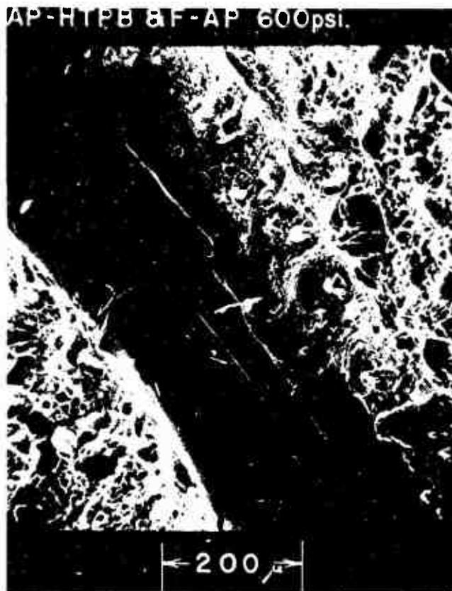
Figure III-67. AP-HTPB and Ferrocene (F)-AP 600 psia (x136).
