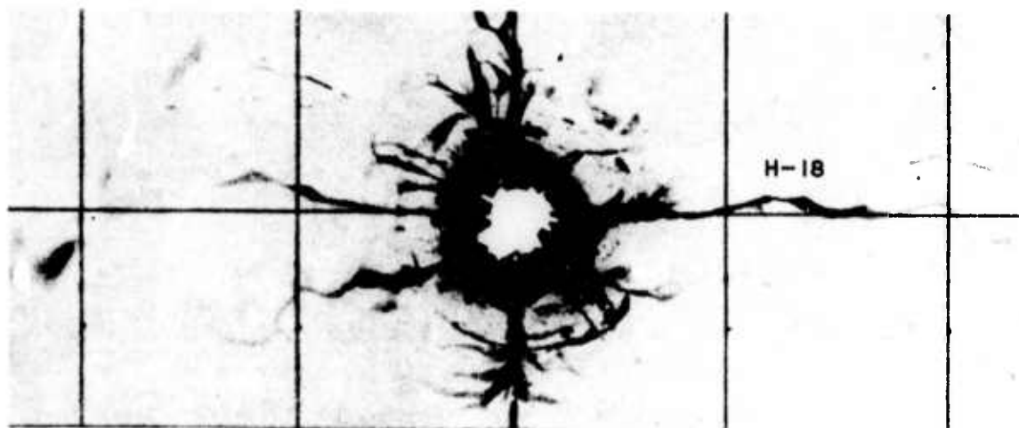
Fig. 6.1 Crack Patterns Existing Before Detonation for Models H-8, H-9 and H-18
