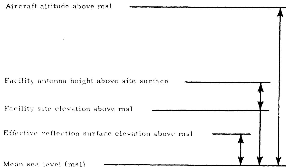
*Figure 1. Antenna heights and surface elevations.*
