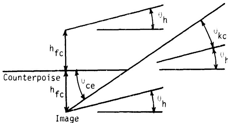
Figure 18. Geometry for determination of counterpoise reflection diffraction parameter,  $v_c$ , associated with the limited reflecting surface of the counterpoise.
