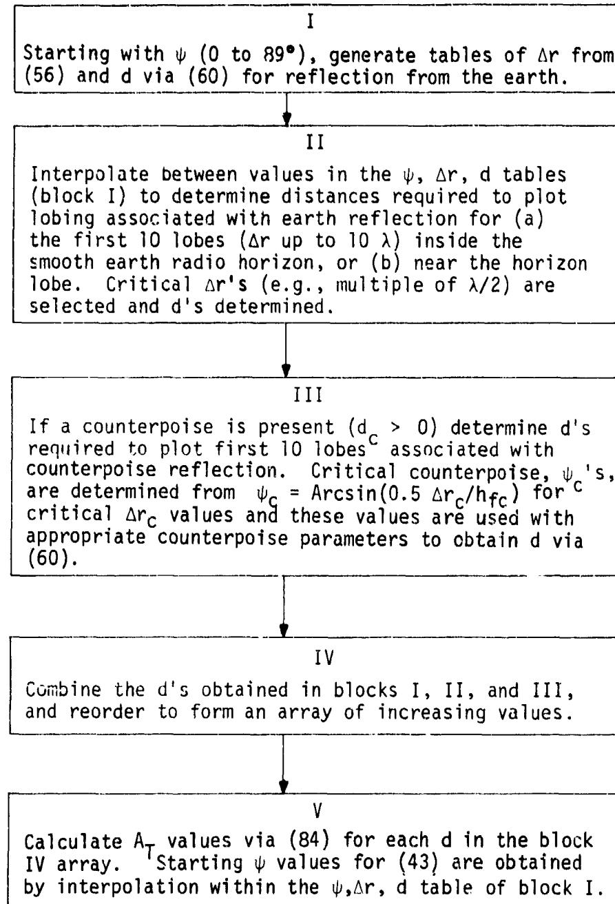
Figure 19. Block diagram of procedure used in line-of-sight calculations.
