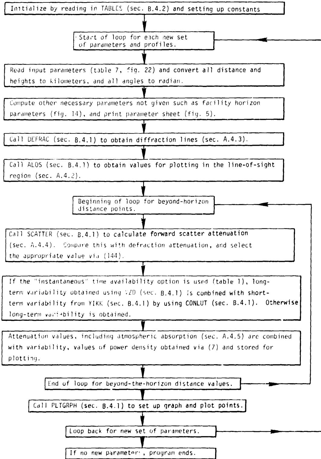
Figure 25. Block diagram for power density program, POWAV.
