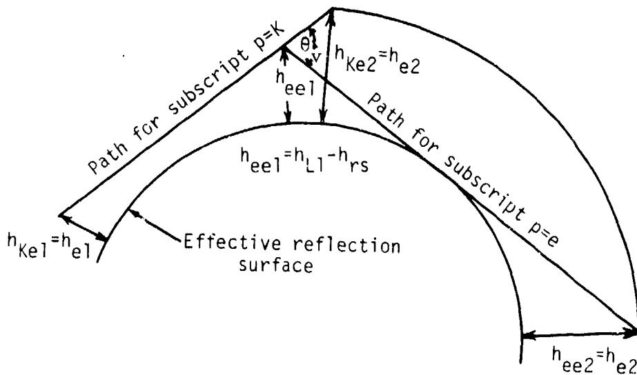
Figure 20. Paths used to determine diffraction loss (not drawn to scale). Rounded earth diffraction is calculated for the  $h_{Ke1}$  to  $h_{Ke2}$  and  $h_{ee1}$  to  $h_{ee2}$  paths. Knife-edge diffraction is calculated for the  $h_{e1}$  to  $h_{Ke2}$  and  $h_{e1}$  to  $h_{ee1}$  paths.
