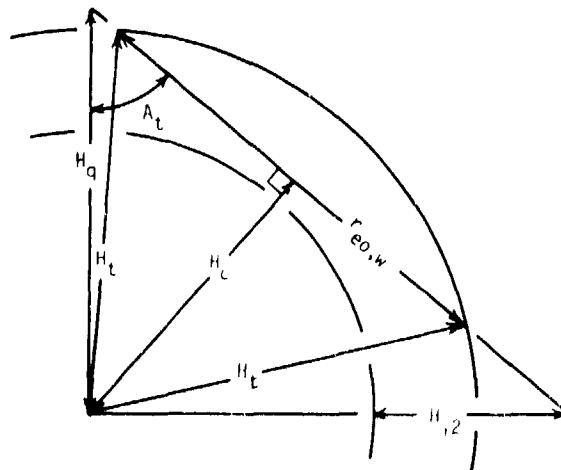
Figure 21. Geometry associated with atmospheric absorption calculations. Values of  $T_{eo,w}$  for oxygen and water vapor are taken as 3.25 and 1.36 km [13, table A.2], respectively (not drawn to scale).
