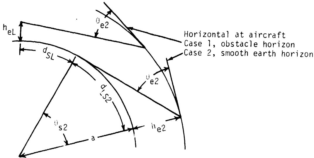
Figure 15. Geometry for aircraft radio horizon
