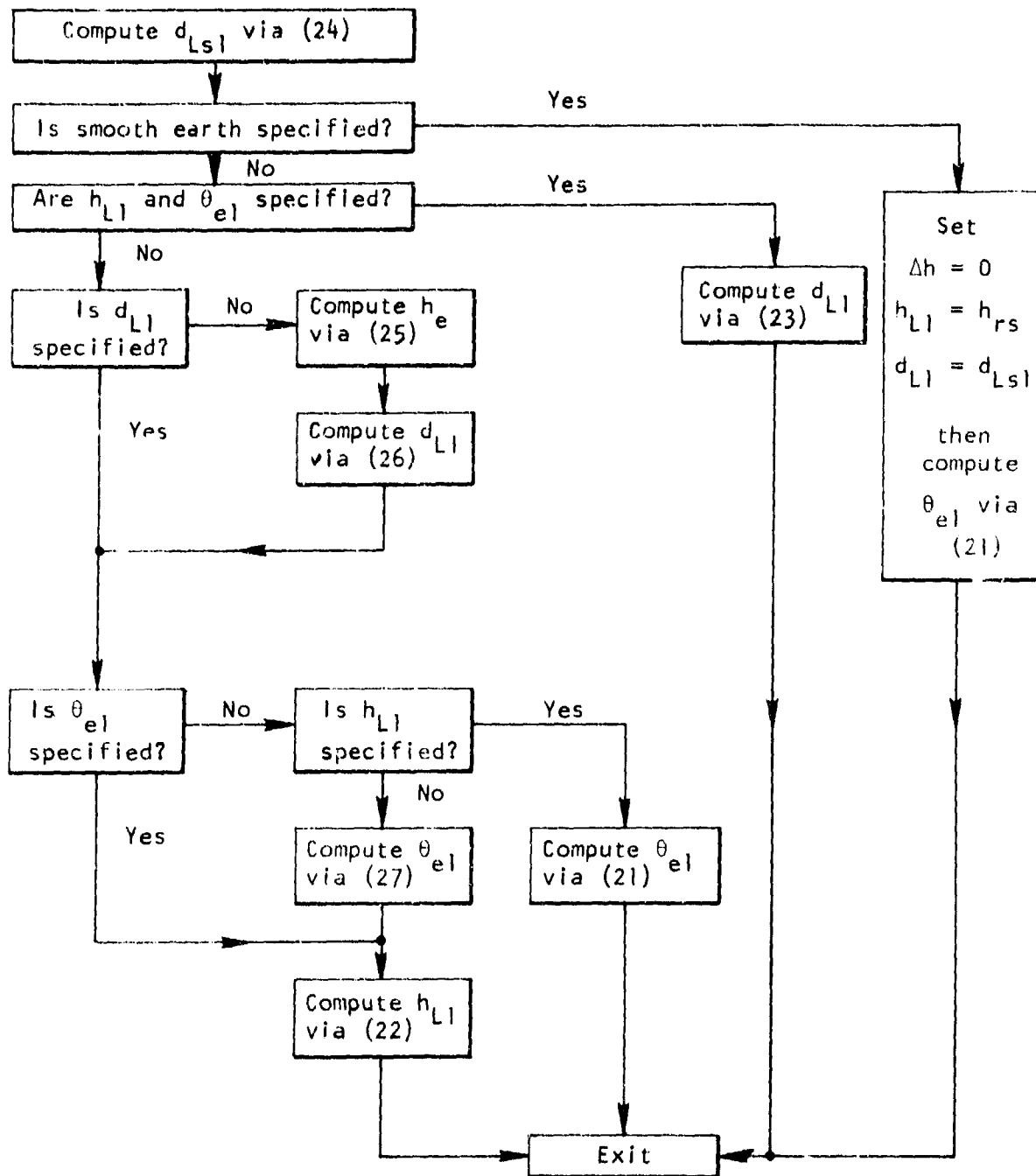
Figure 14. Logic for facility horizon determination.
