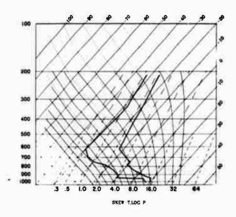
Figure I. A computer-generated SKEW-T background with a hypothetical profile of temperature and dewpoint temperature. Horizontal lines are pressure. Positive sloped lines are temperature (solid) and mixing ratio (dashed). Negative sloped curves are dry adiabat (dashed) and saturated adiabat (solid).
