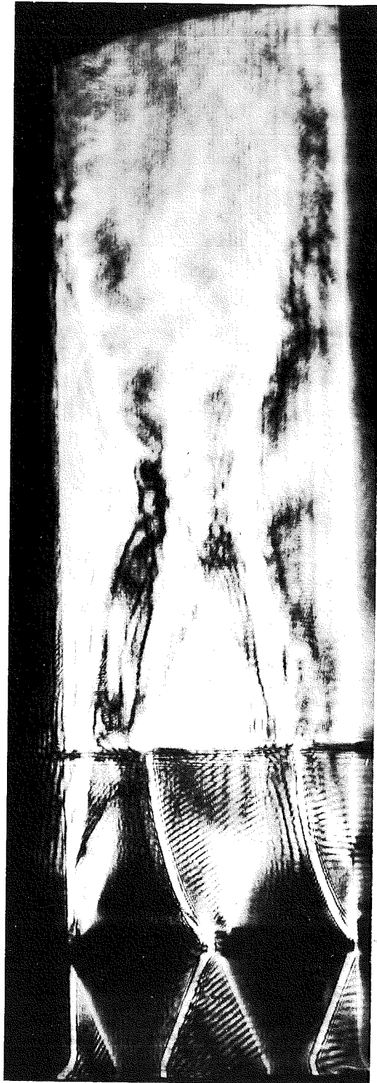
Figure 15. Schlieren of run 21, condition 12 with knife edge set vertically.
