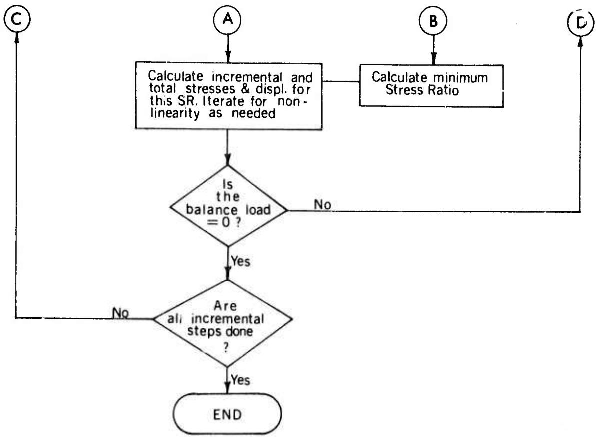
FIG. II-1. Flow Chart for Progressive Failure of Elastic-Plastic Incremental System
