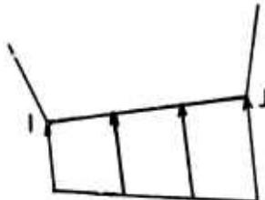
As shown in the sketch, the boundary of the element must be on the left hand side as one progresses from I to J. Surface tensile force is input as a negative pressure.
