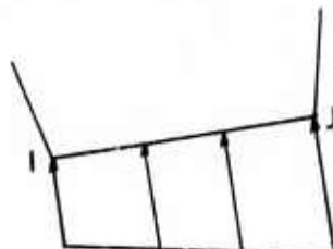
As shown in the sketch, the boundary element must be on the left as one progresses from I to J. Surface tensile force is input as a negative pressure.
