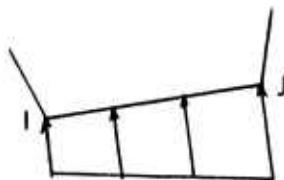
As shown in the sketch, the boundary element must be on the left as one progresses counter-clockwise from I to J. Surface tensile force is input as a negative pressure.
