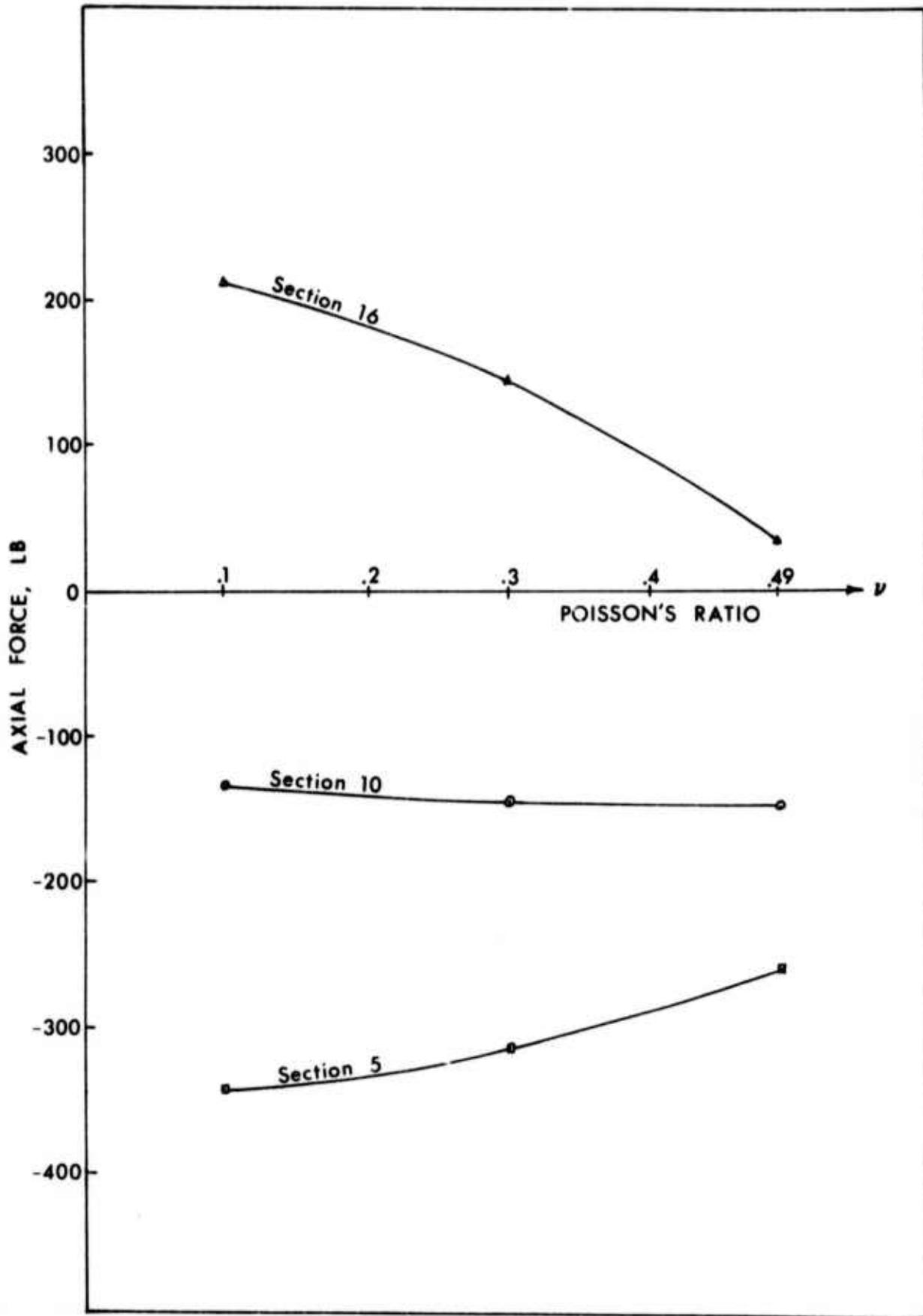
FIG. VI-20. Influence of Poisson's Ratio on Axial Force
