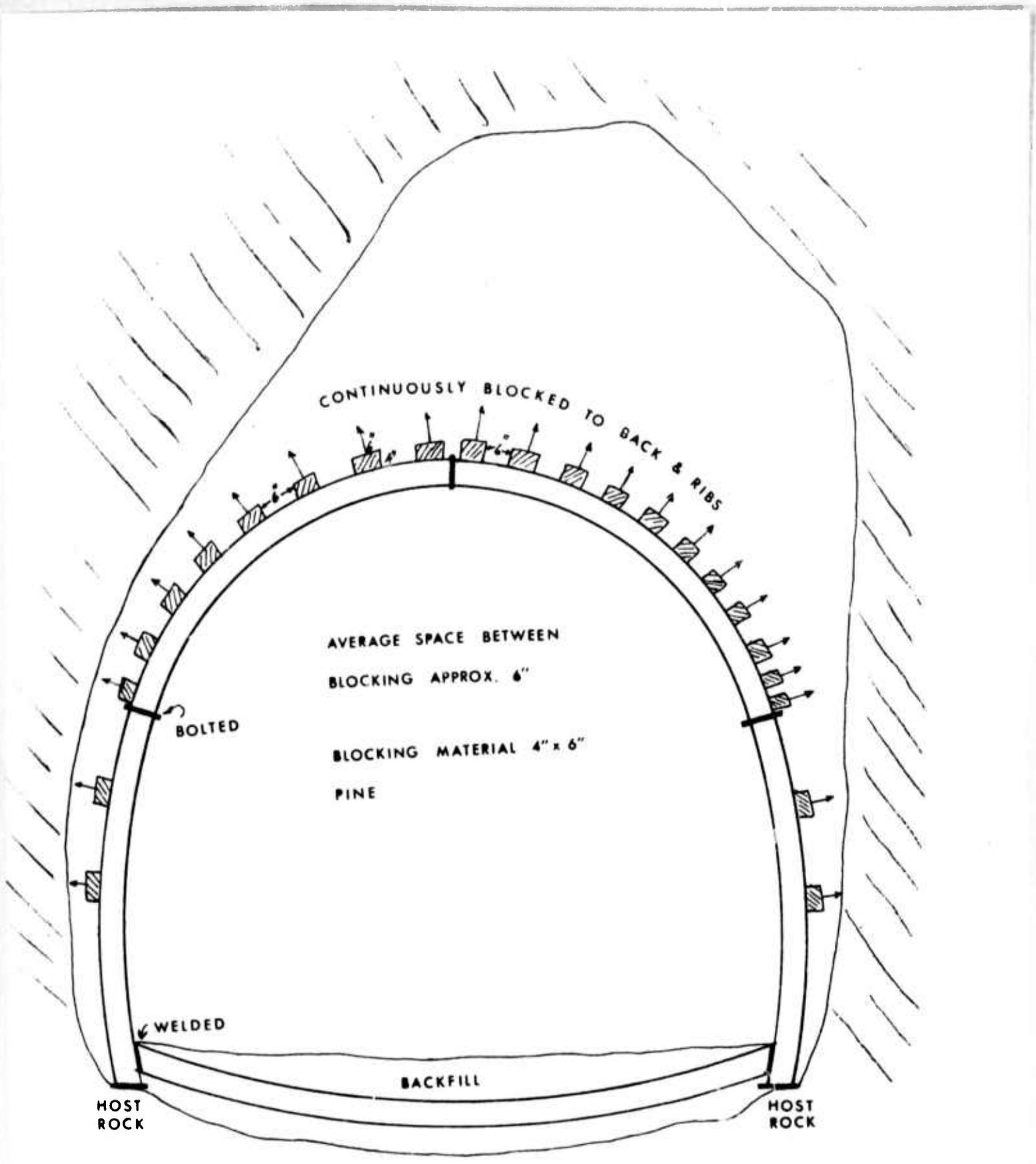
FIG. VI-3. Tunnel Excavation and Supports
