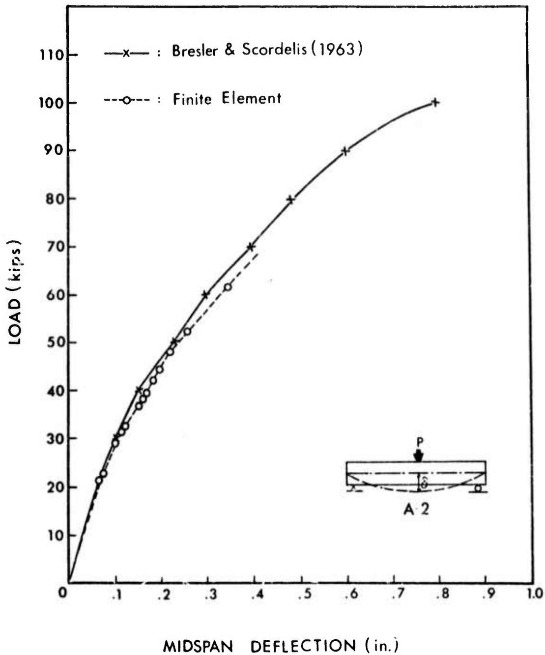
FIG.V-12. Load-Deflection Curve for Beam A-2
