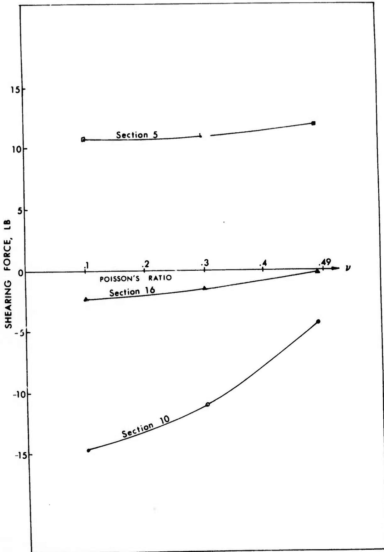
FIG. VI-21. Influence of Poisson's Ratio on Shearing Force
