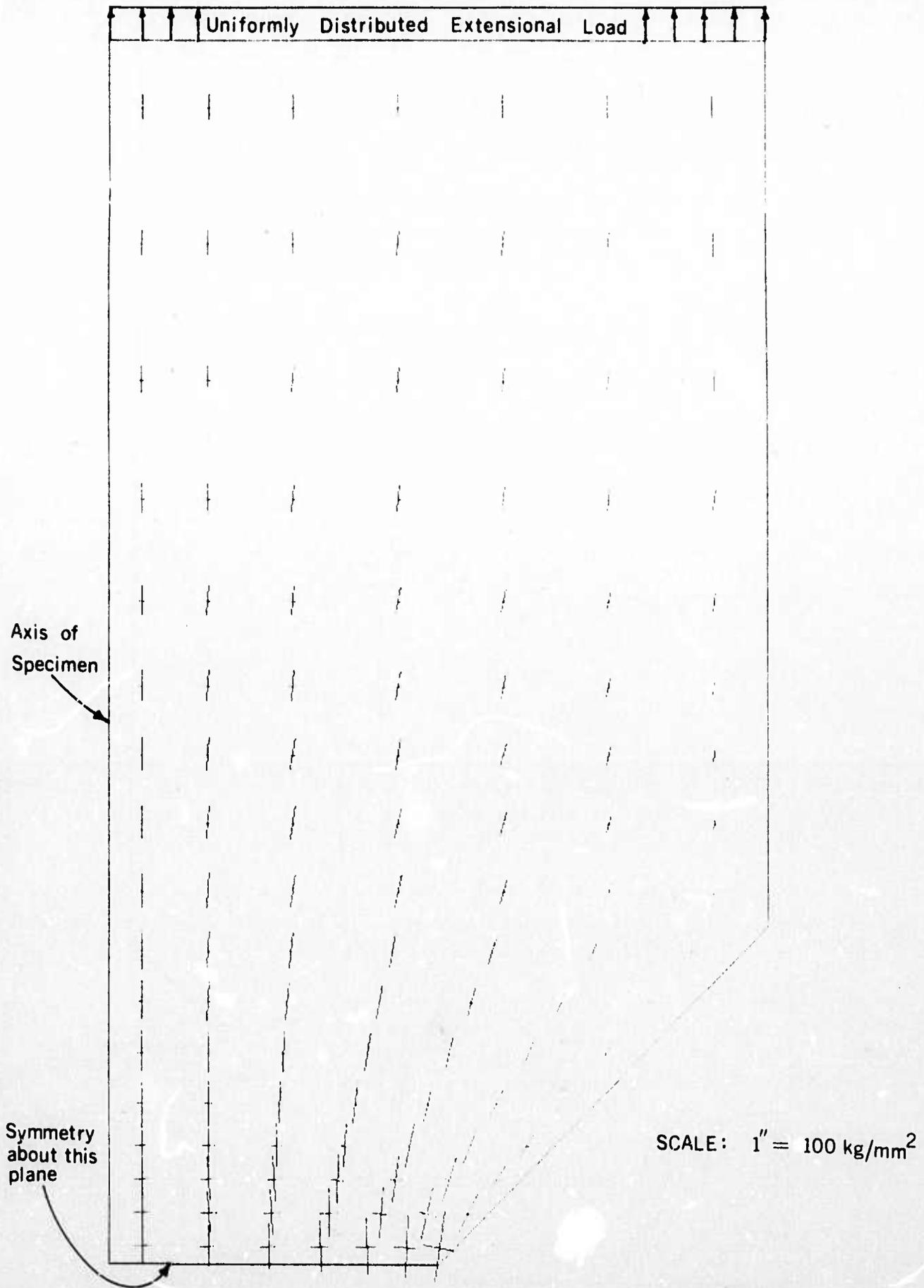
FIG. IV-9. Notched Specimen (One Quarter) - Elastic-Plastic Stress Distribution Under Uniform Load of  $19.2 \text{ kg./mm.}^2$  Applied at Ends
