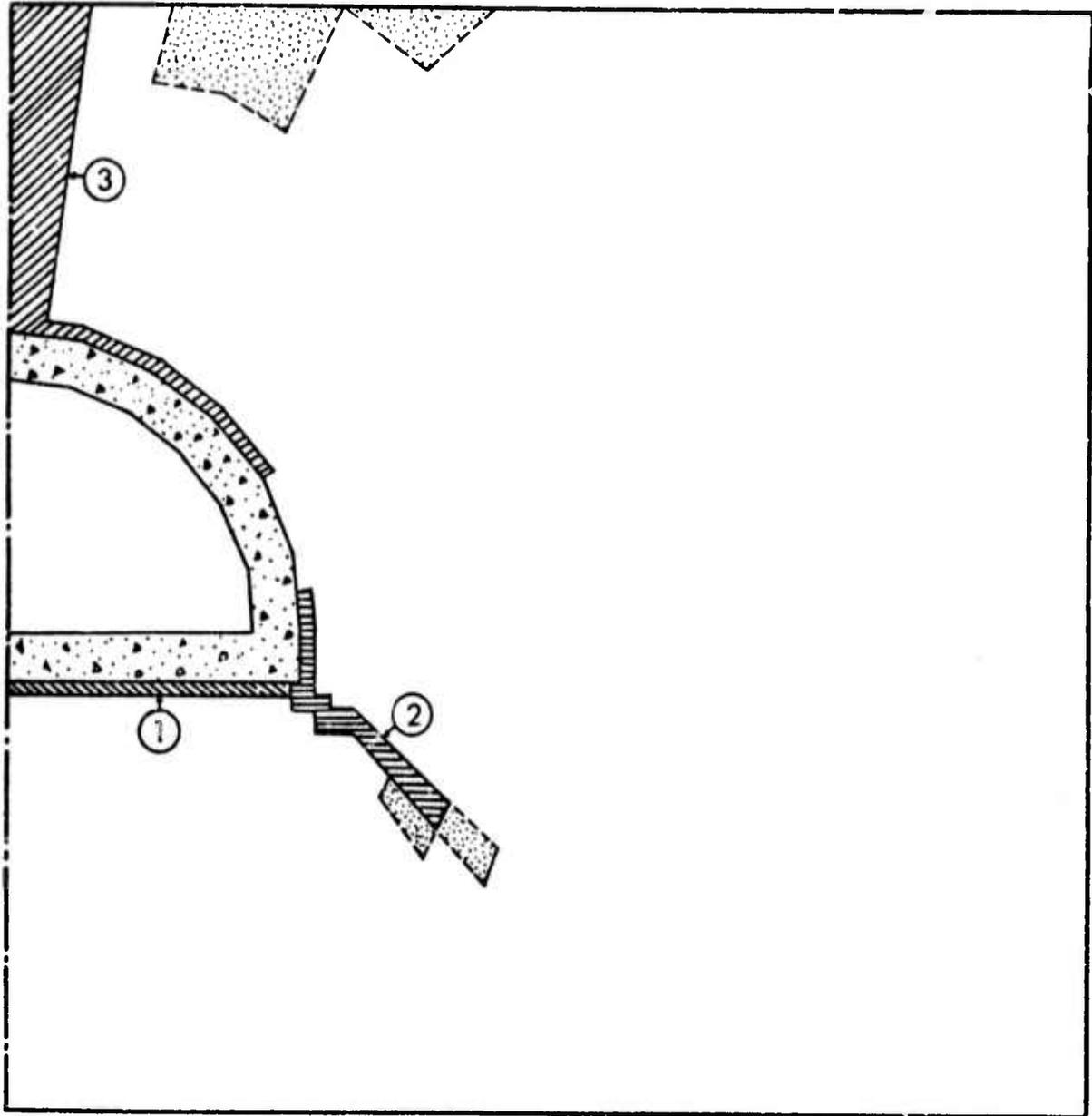
FIG. V-16 Sequence of Cracking and Final Tensile Zones in Rock
