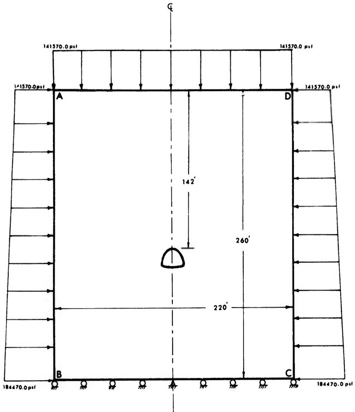
FIG. VI-7. Boundary Conditions on the Finite Element Model
