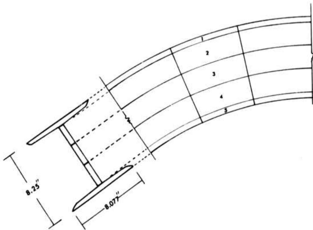
FIG. VI-9. Finite Element Representation of the Cross-Section of Steel Rib
