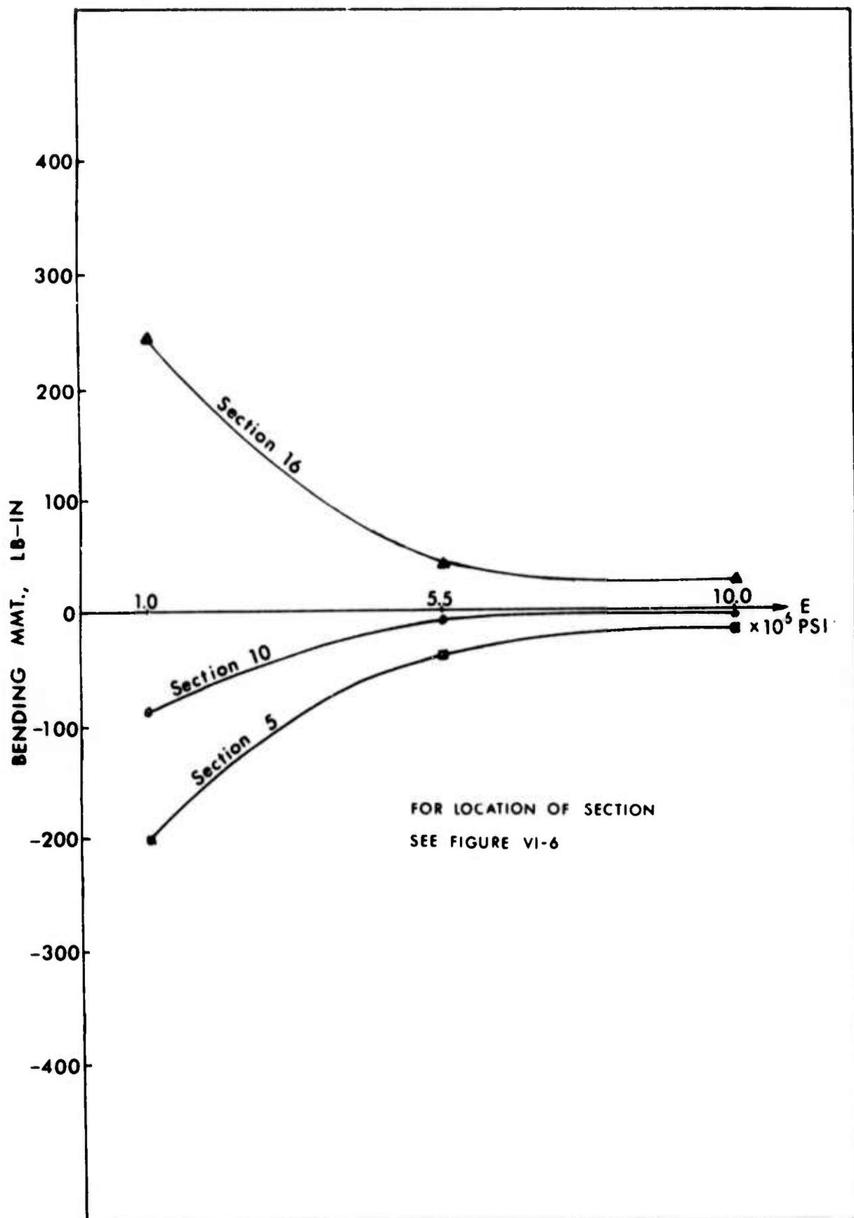
FIG. VI-16. Influence of Elastic Modulus on Bending Moments
