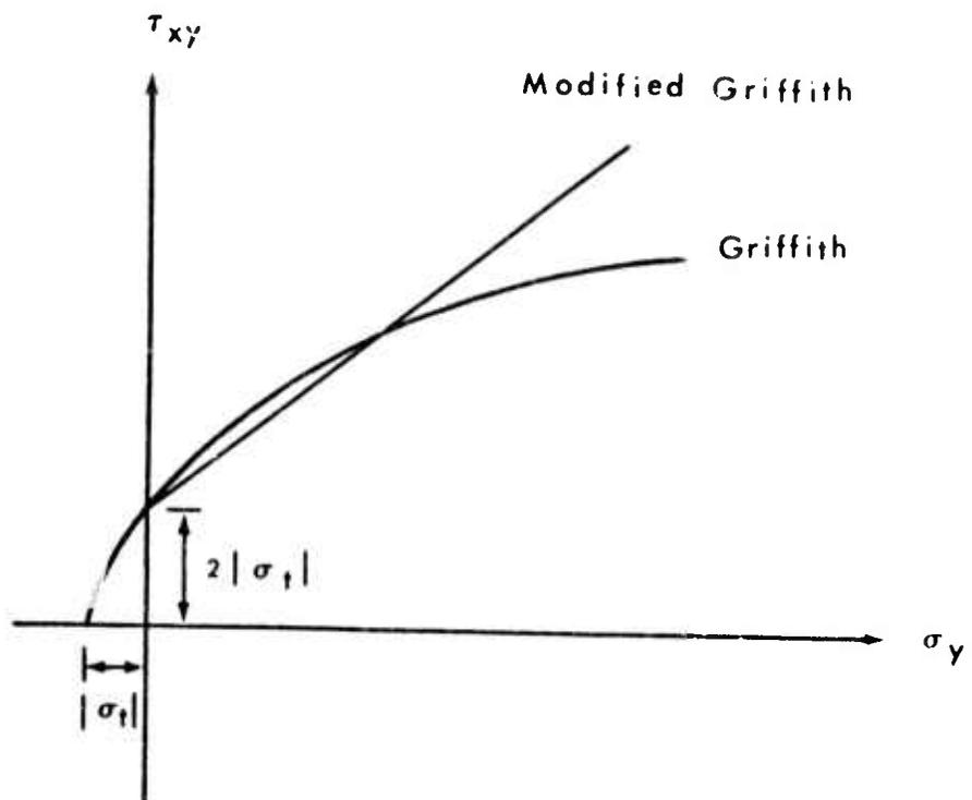
Fig. A-3 Mohr's Diagram for Griffith and Modified Griffith Criteria
