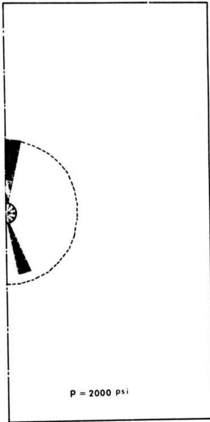
FIG. V-22. Sequential Cracking Due to Internal Pressure on Tunnel Surface - 2000 psi
