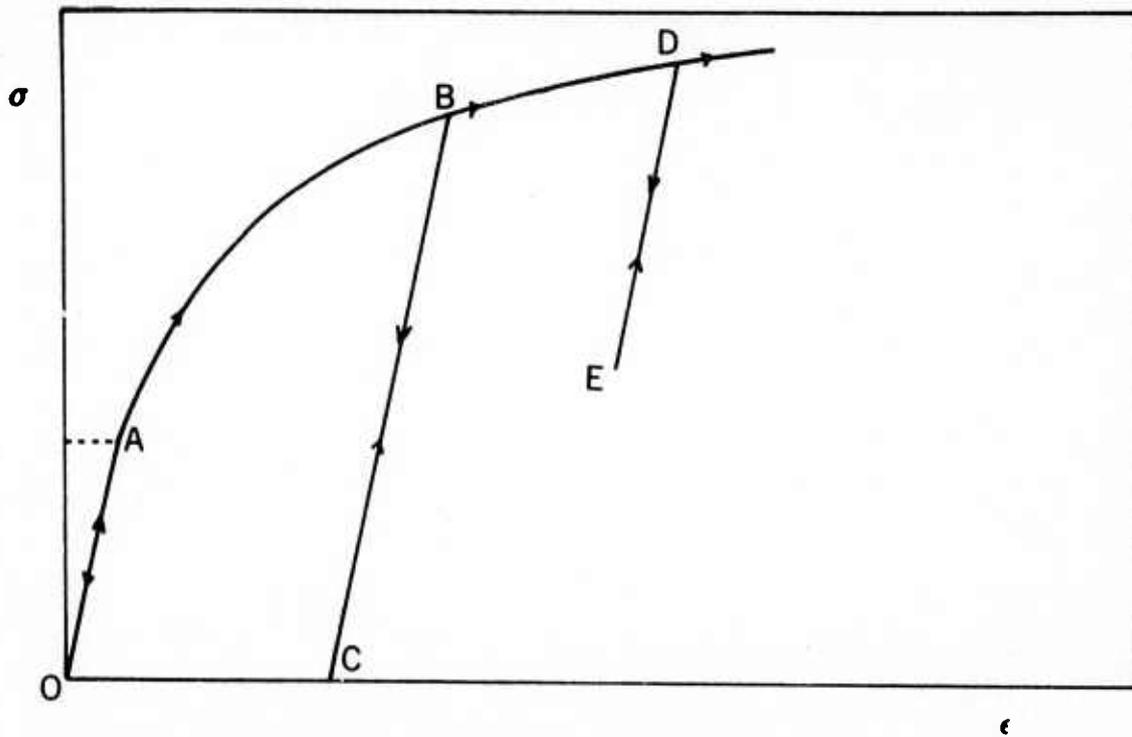
FIG. II-3. Idealization of Elastic-Plastic Stress-Strain Behavior for Rocks
