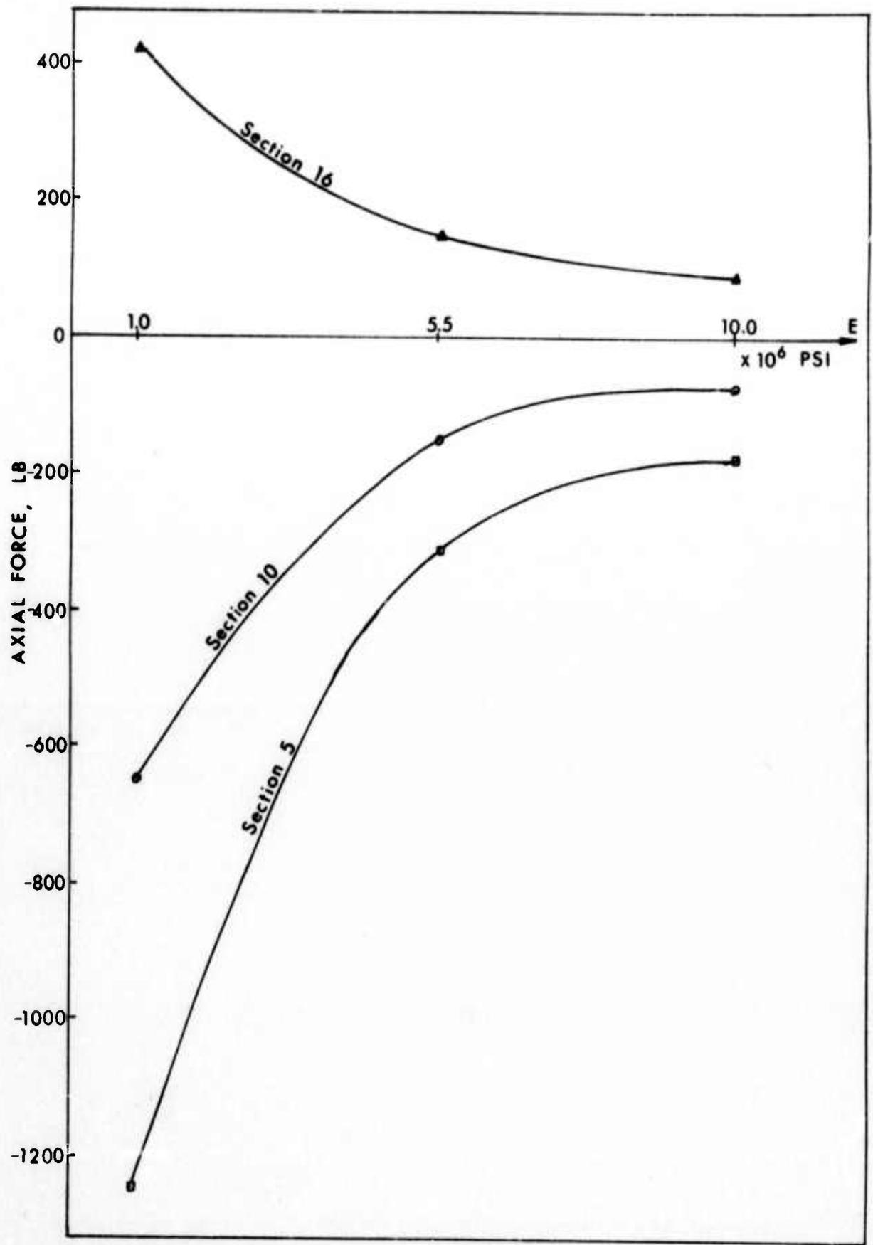
FIG. VI-17. Influence of Elastic Modulus on Axial Force
