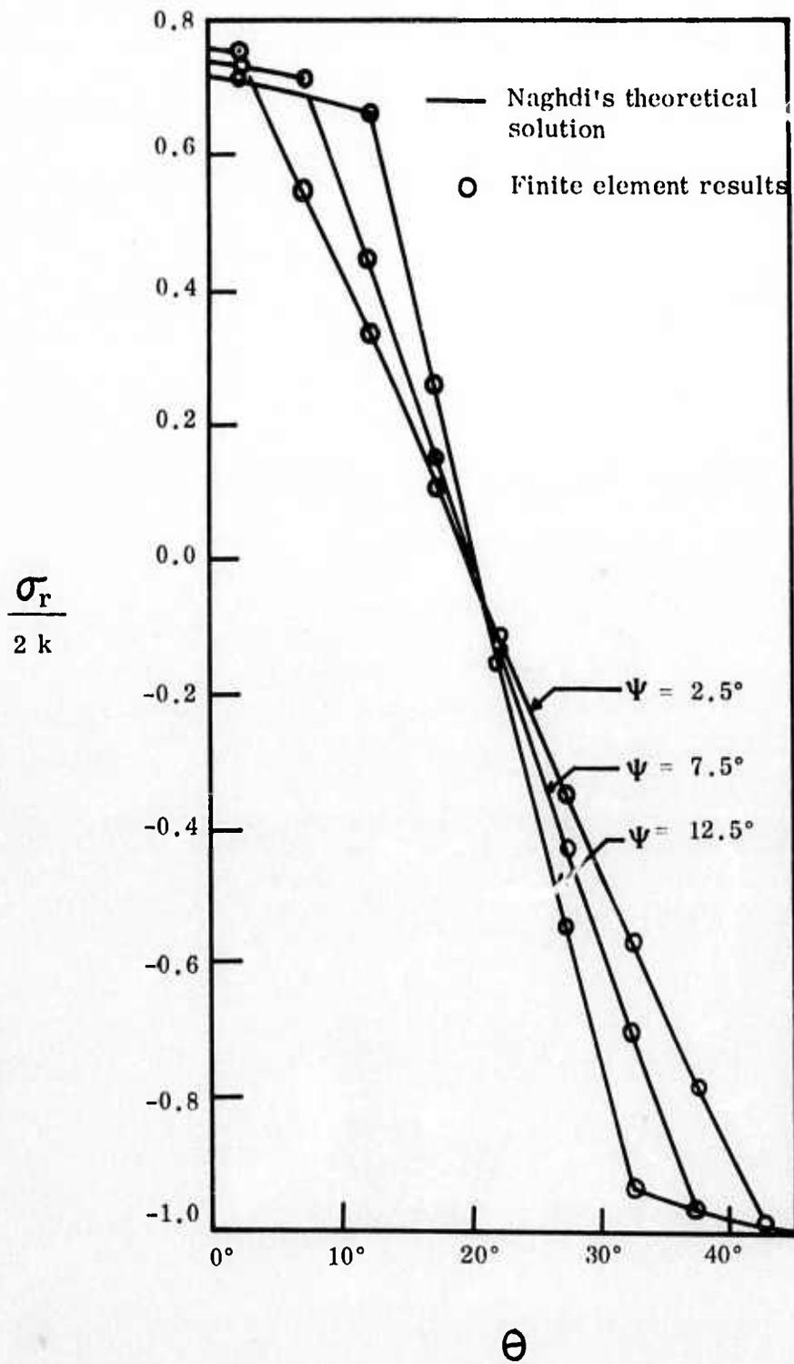
FIG. IV-5. Distribution of Radial Stress for Wedge at Various Load
