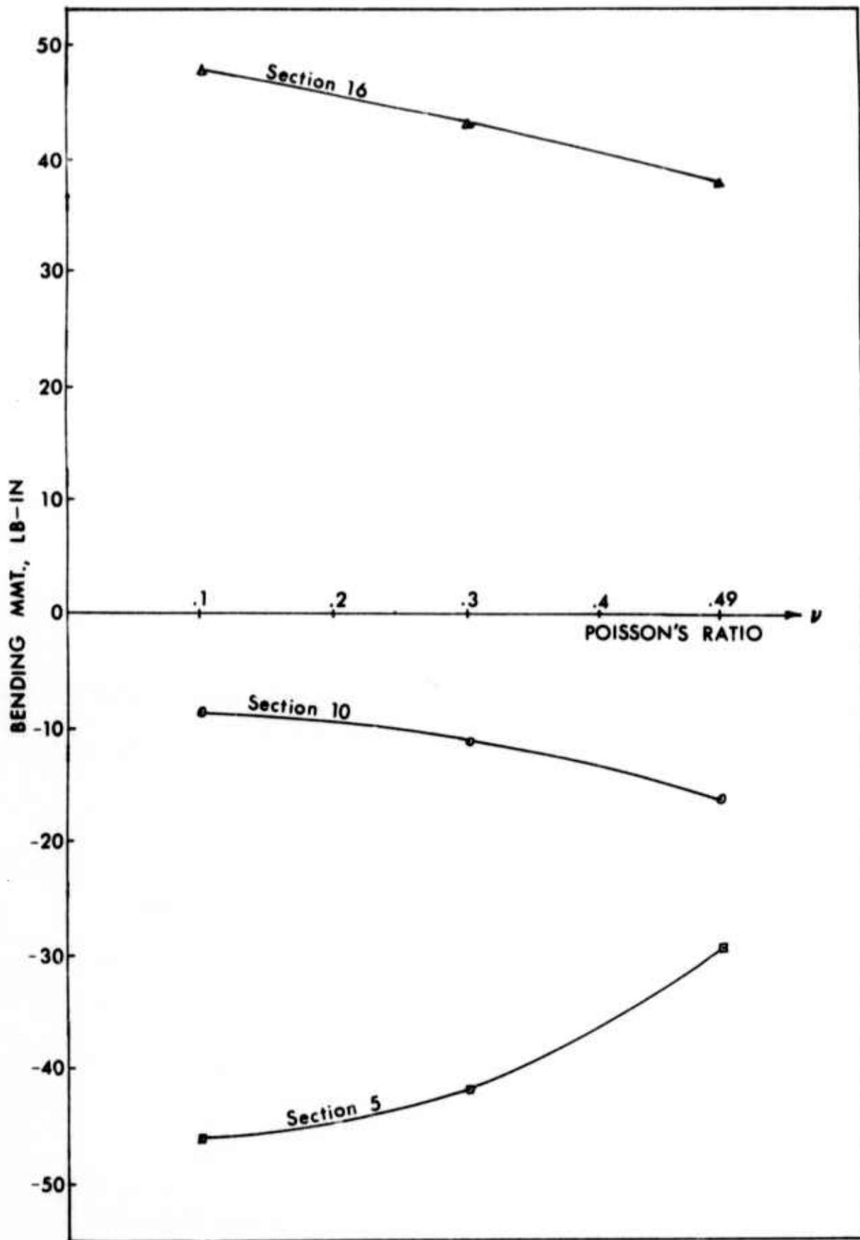
FIG. VI-19. Influence of Poisson's Ratio on Bending Moments
