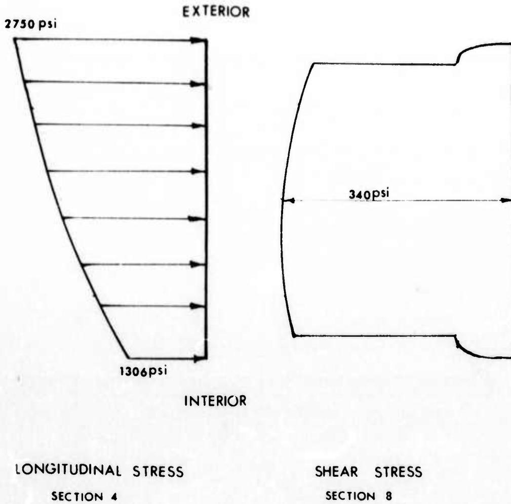
FIG. VI-32. Distribution of Longitudinal and Shearing Stresses on Critical Sections
