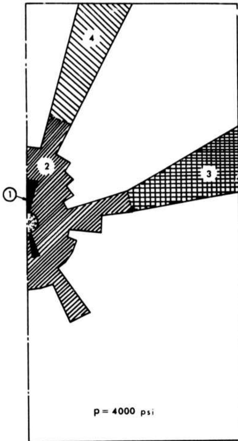
FIG. V-24 Sequential Cracking Due to Internal Pressure on Tunnel Surface - 4000 psi
