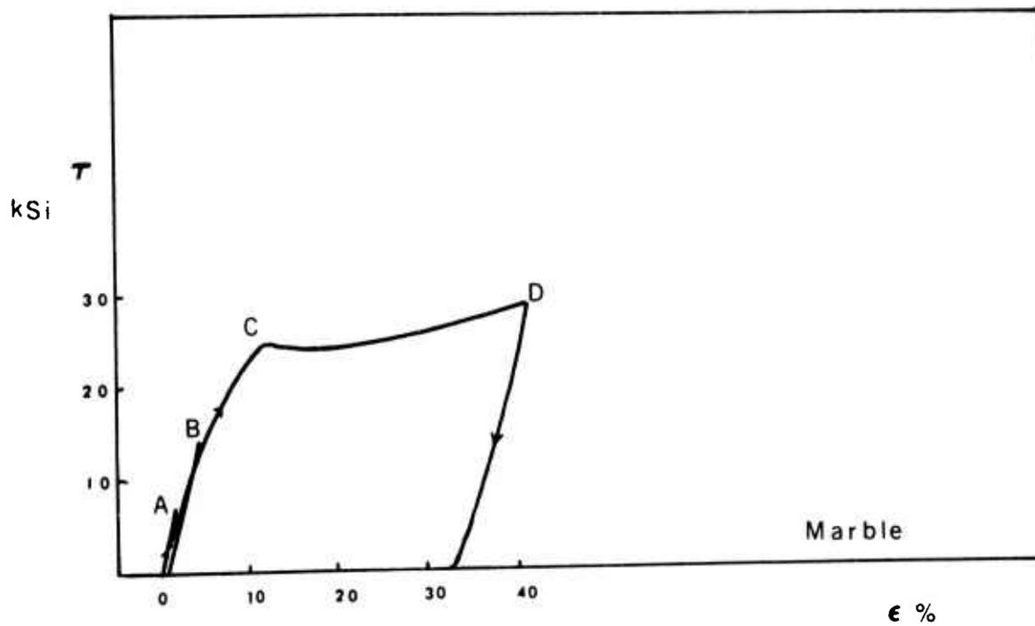
FIG. II-2. Stress-Strain Curves for Marble (Swanson, 1970)
