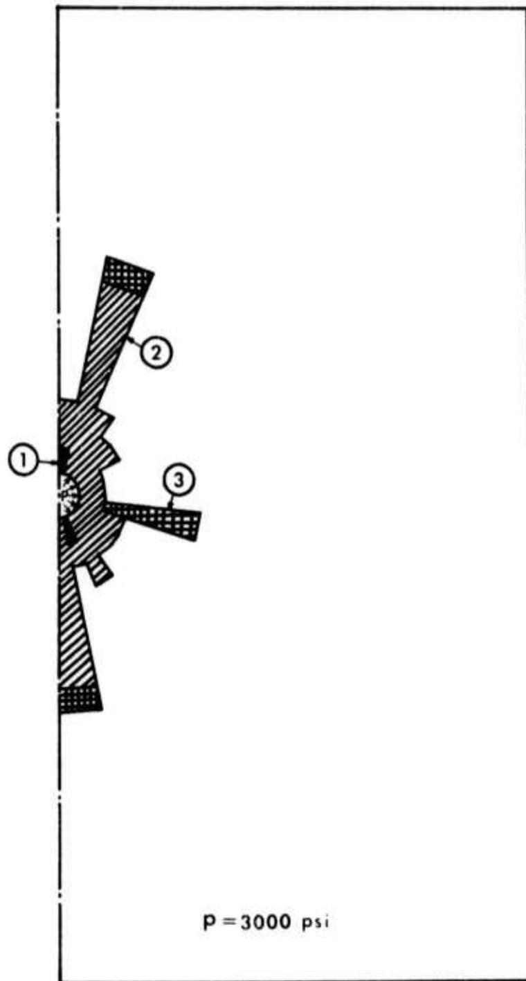
FIG. V-23 Sequential Cracking Due to Internal Pressure on Tunnel Surface - 3000 psi
