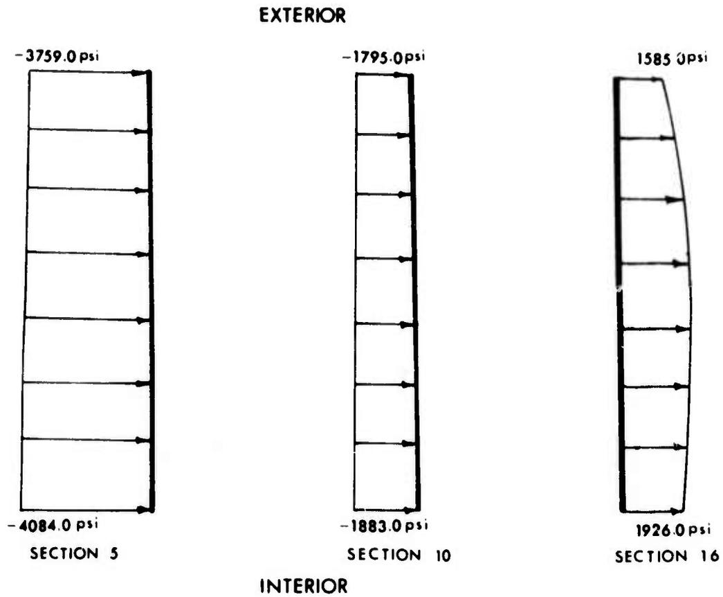
FIG. VI-22. Longitudinal Stress Distribution for Case (a) - Mean Values of E and  $\nu$
