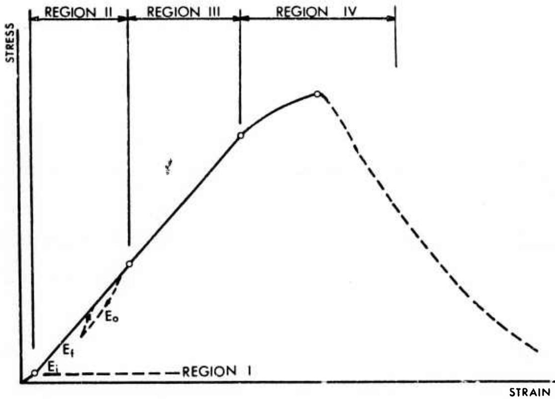
FIG. II-8. Typical Stress-Strain Curve for a Rock Specimen Under Multiple-Axial Loading (Walsh, 1965a)
