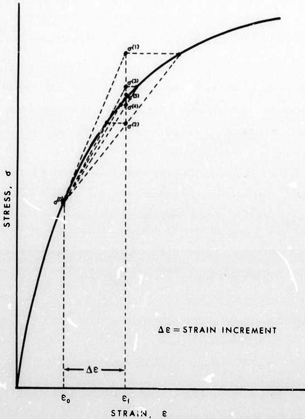
FIG. IV-3a. Calculation of Stress for a Strain Increment - Method 1
