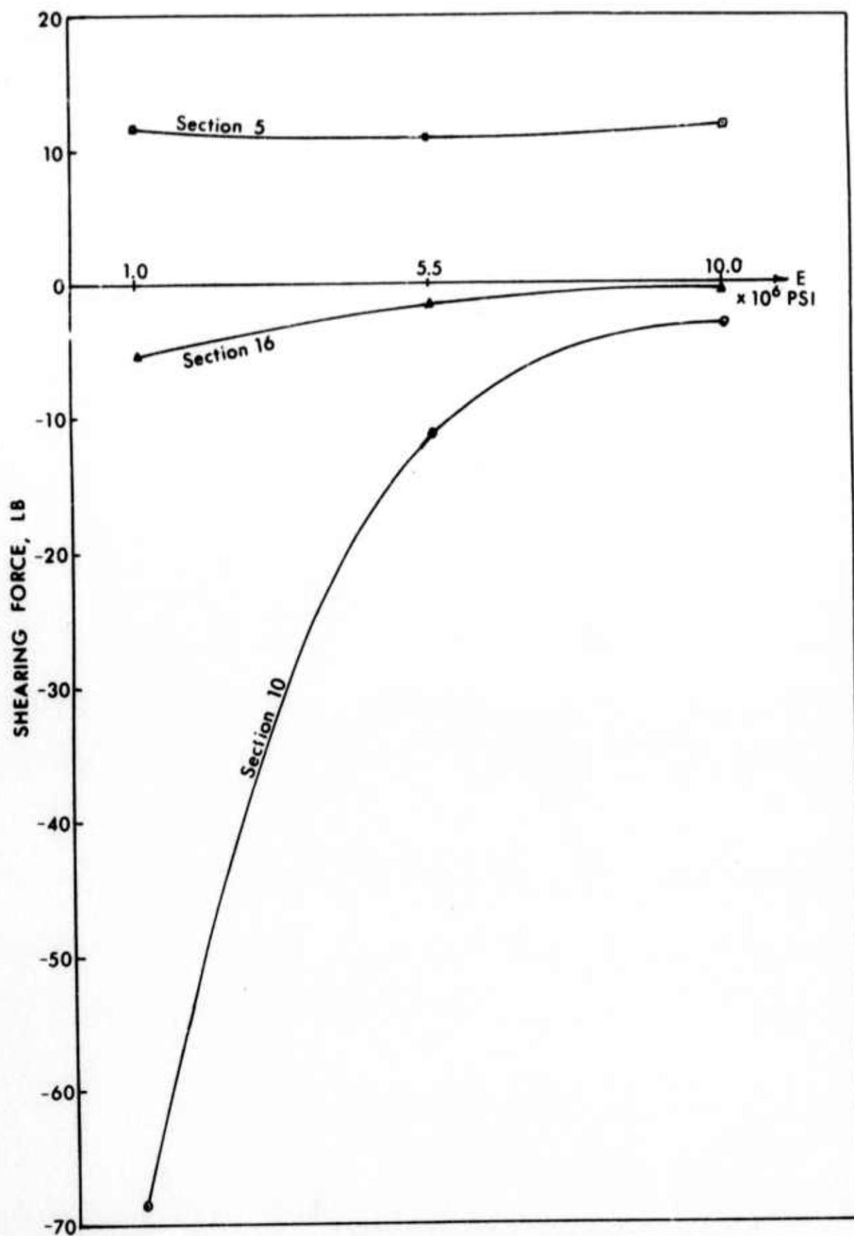
FIG. VI-18. Influence of Elastic Modulus on Shearing Force
