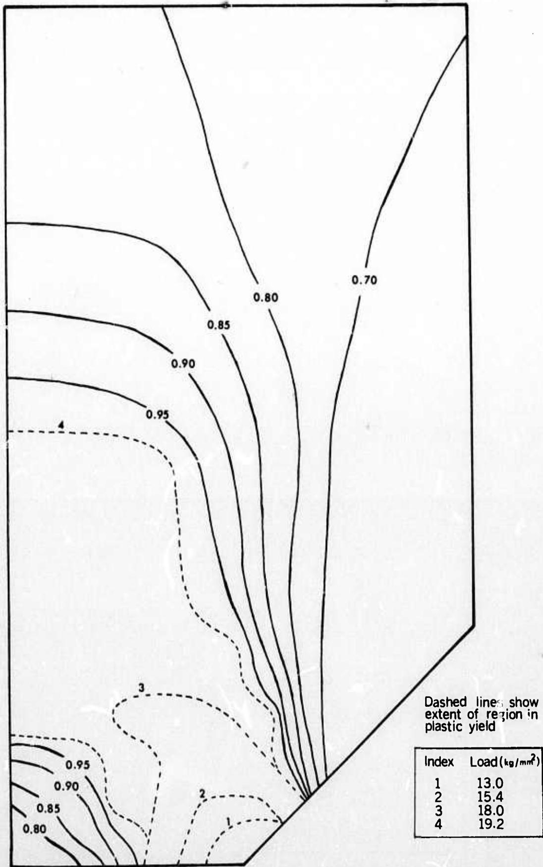
FIG. IV-10. Notched Specimen - Contours of Failure Ratio at Uniform Extensional Load of 19.2 kg./mm.<sup>2</sup> Applied at Ends
