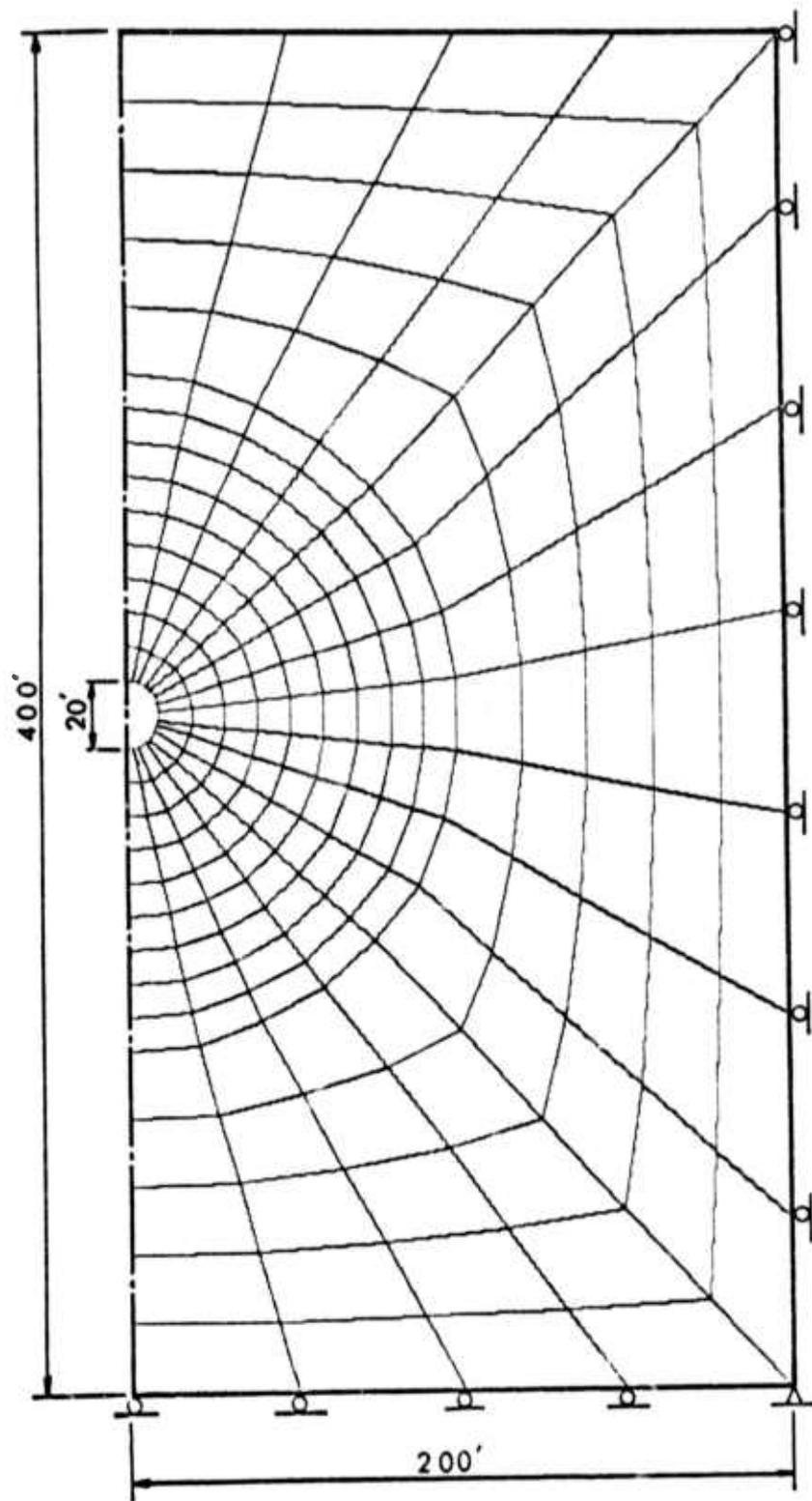
FIG. V-21. Finite Element Idealization of a Circular Tunnel
