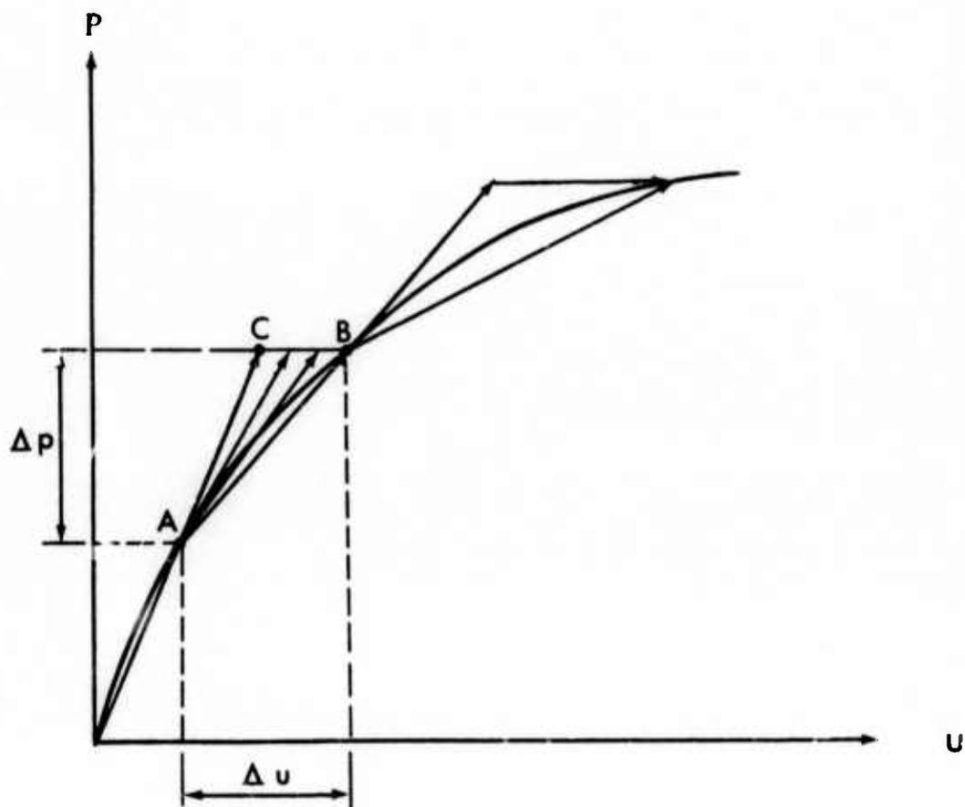
Fig. V-5. Incremental Loading Analysis
