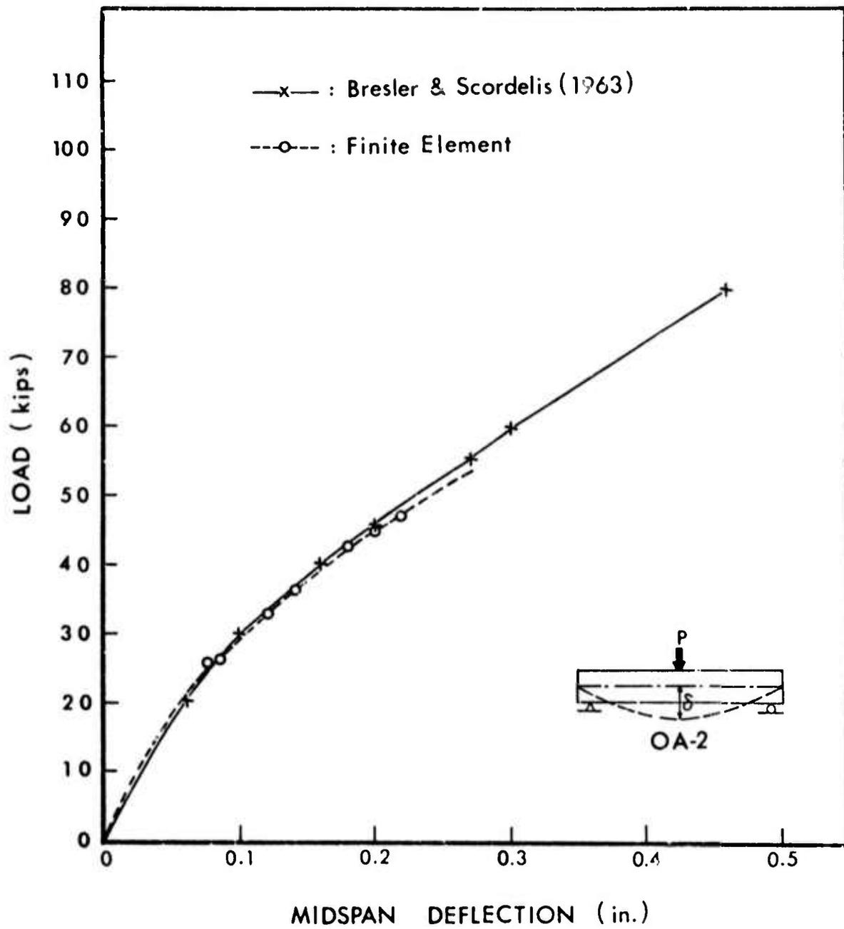
FIG. V-10. Load-Deflection Curve for Beam OA-2
