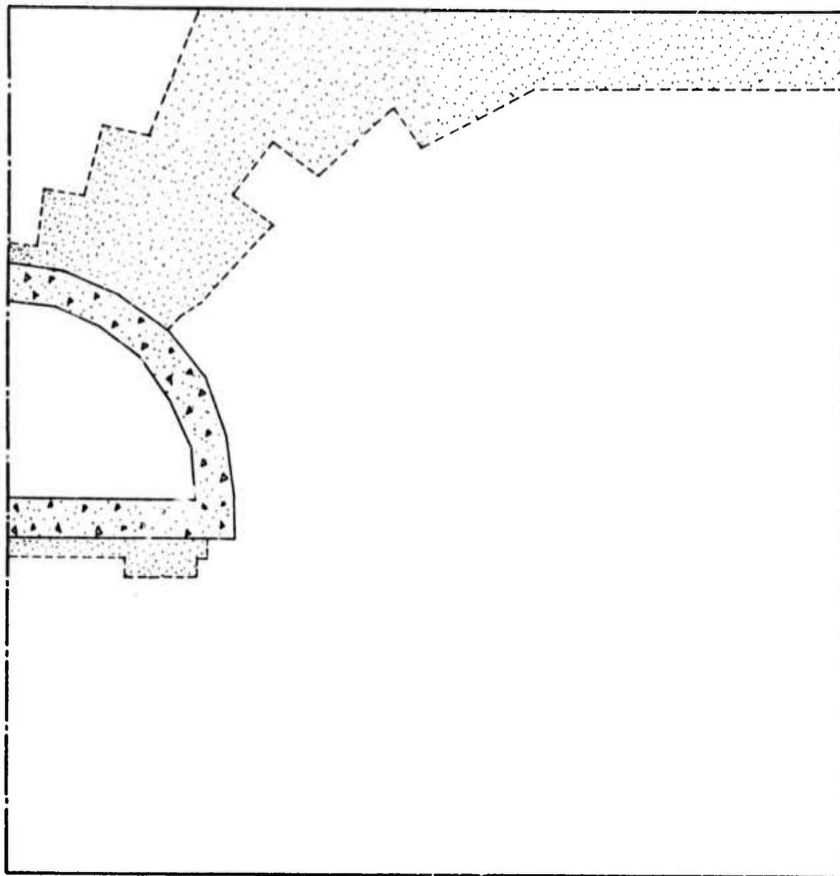
FIG. V-15 Initial Tensile Zones in Rock
