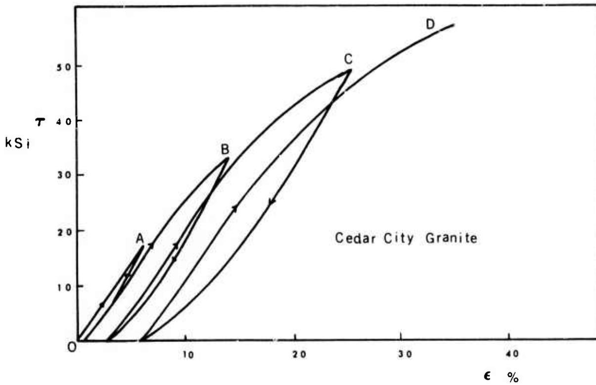
FIG. II-1. Stress-Strain Curves for Cedar City Granite (Swanson, 1970)
