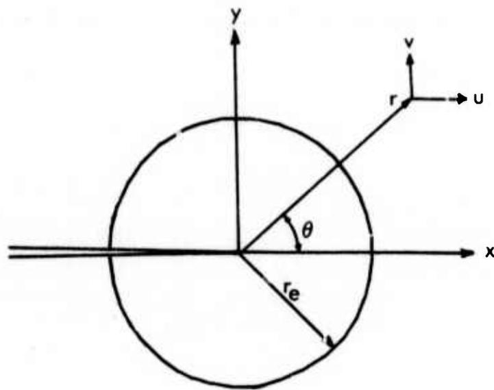
Fig. V-3. Cracked Element (Wilson, 1971)
