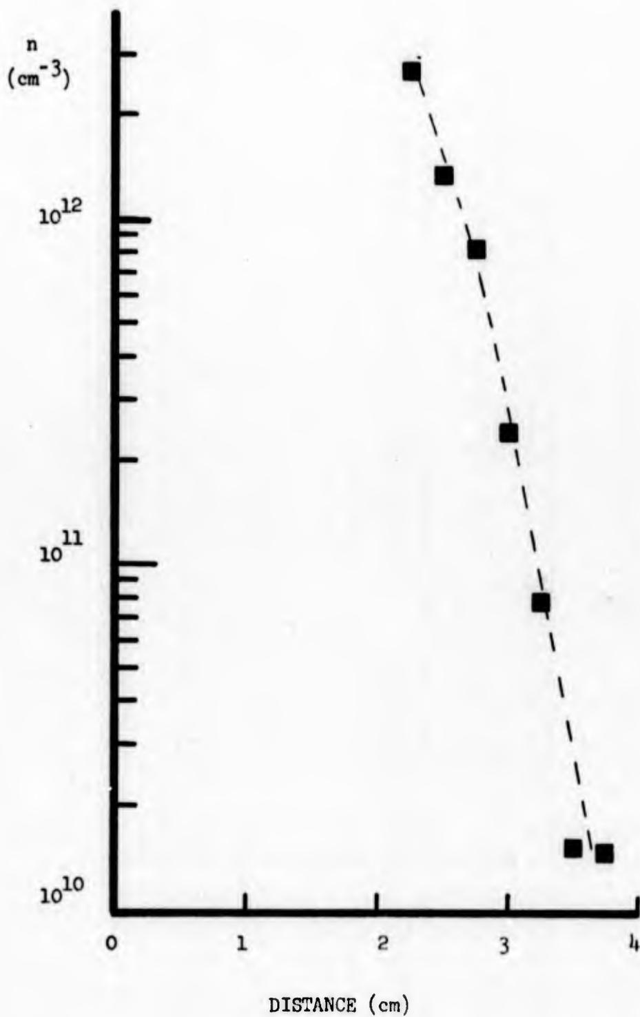
Figure 21 Langmuir Probe Number Density  $n$  Versus Distance From Arc Center. Arc is Helium
