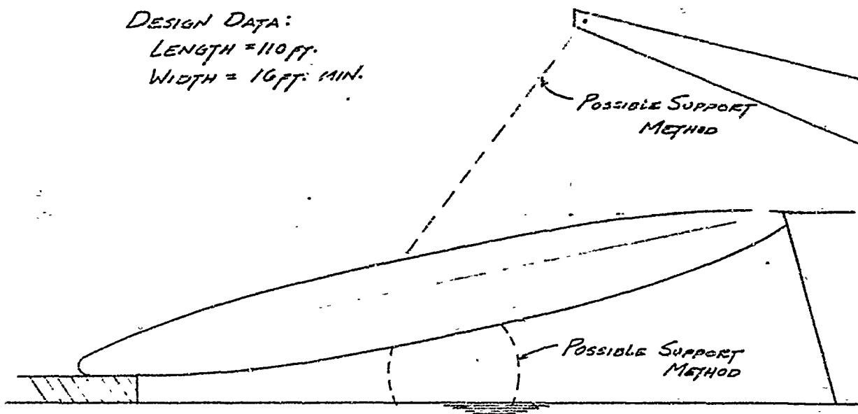
ANALYZE FIRST AS A FLAT PLATE WITH NO SUPPORT MECHANISM
