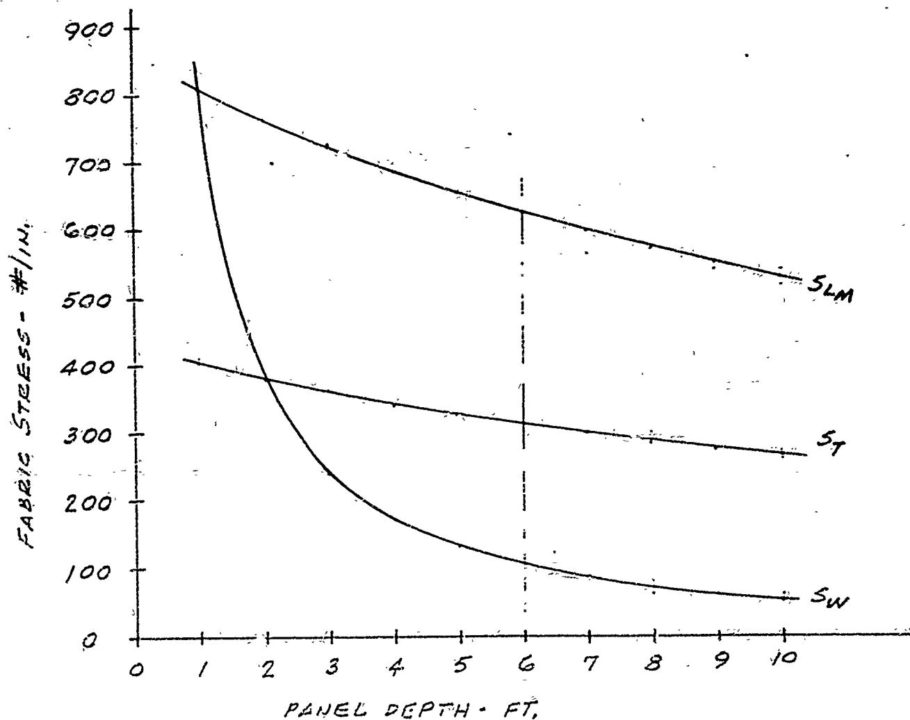
IN CONSIDERATION OF PRESSURE AND STRESSES, AN "OPTIMUM" CELL DEPTH WOULD APPEAR TO BE APPR. 6 FT.
