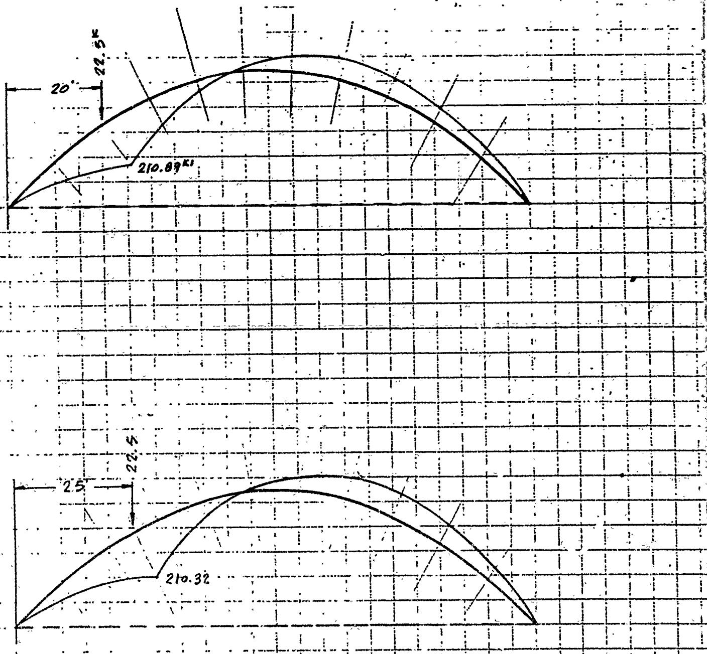
$$\text{Compute } M \text{ @ Load } M = \frac{(22.5)(85)(25)}{110} - (11.613)(19.5182) = 210.32 \text{ k}'$$
