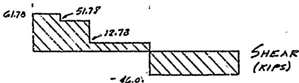
NOTE: MAX. SHEAR OCCURES WITH LARGEST WHEEL LOAD AT SUPPORT
