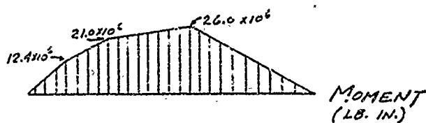
\* Note: If load is considered as a concentrated force at midspan, max. bending moment is:
