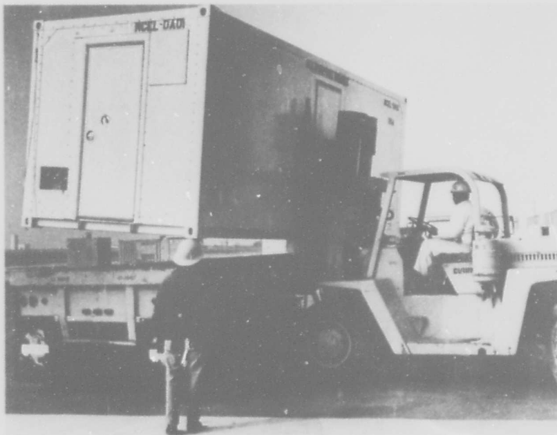
Figure 33. Forklift loading the all purpose module onto a flatbed semi-trailer.
