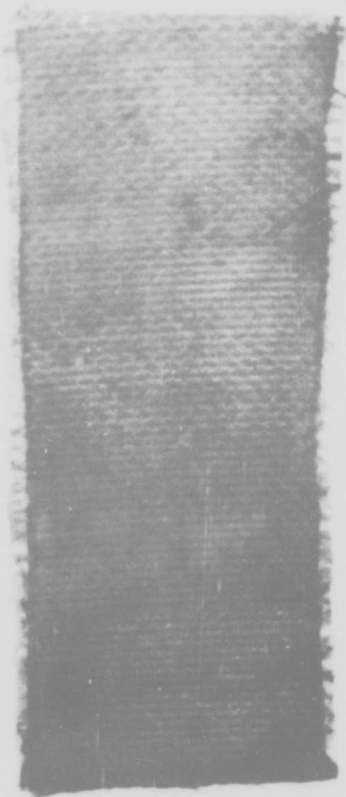
Figure 60. Radiograph of 5-D Astroquartz Omniweave/Ludox AS Plate 401-3
