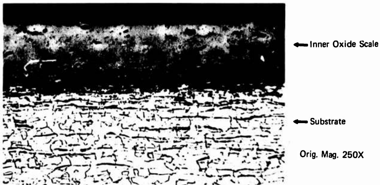
Figure 7. Cross section of oxides formed on FS-85 after 1 hr at 1600 F 19-066-1589/AMC-72
