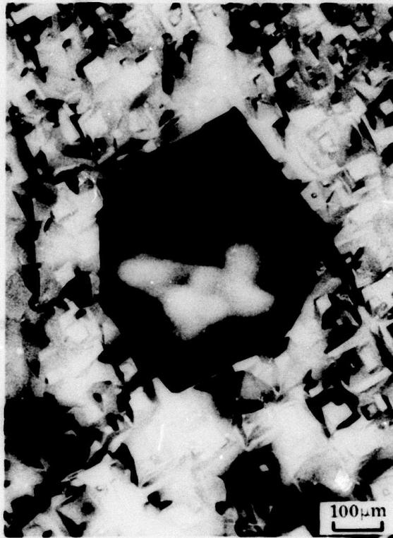
Figure 58. Surface of Verneuil-grown  $(10\bar{1}4)Al_2O_3$  after Etching with Freon at 1500C for ~3 hr at Nominal Rate of  $0.6\mu\text{m}/\text{min}$ .<sup>3</sup> (Several deep large etch pits (as in center) were randomly distributed on surface.)
