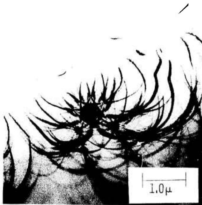
Figure 66. Electron Micrograph of (0001) $\text{Al}_2\text{O}_3$  Substrate
