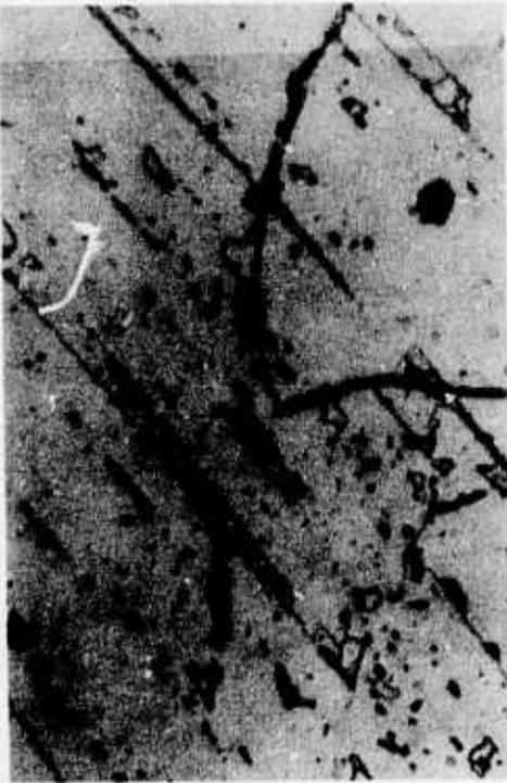
(a) Initial surface (200x) prepared by cleaving at (100) and followed by a heat treatment at 670°C for 20 hours under He. Cleavage steps almost gone and surface is decorated by vapor deposited material.
