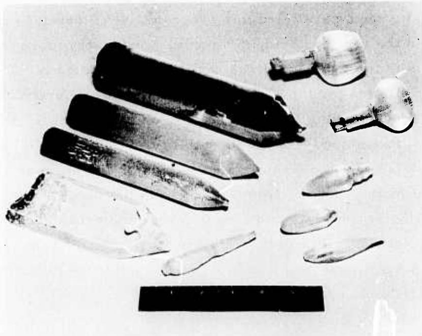
Fig. 4. Czochralski Boules and Bridgman Cylinders and Flat Ingots of Single-Crystal KCl.
