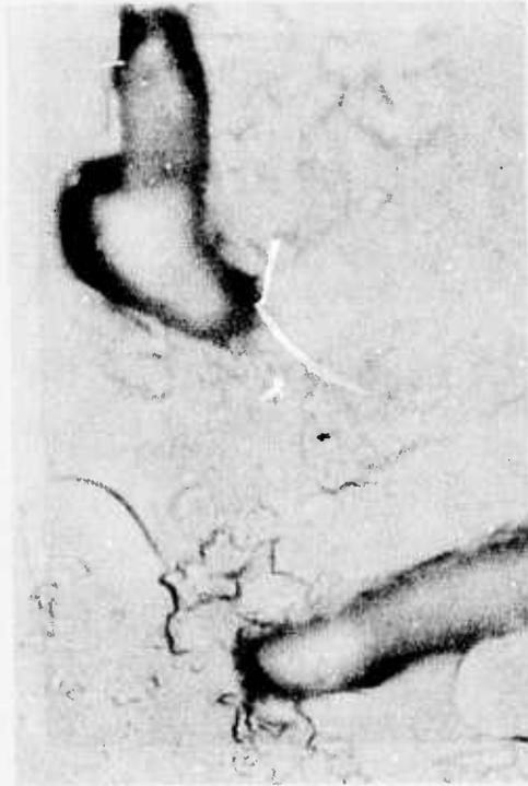
(c) The center of (b) at 1000x showing no etch pits.
