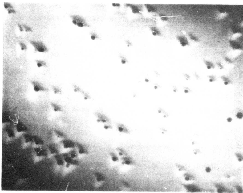
Figure 13. Same Area as Fig. 12, Dark Field Transmitted Illumination, Focused About 30 \mu\text{m} Below Surface of the Epitaxial Layer (200X).
