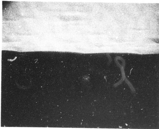
Figure 14. SEM Photograph of Fractured Section of the Epitaxial Layer Shown in Figs. 12 and 13. Substrate is at the Bottom and the Top Surface of the Layer is Visible at the Top. Incident Angle 80^\circ , 500X.
