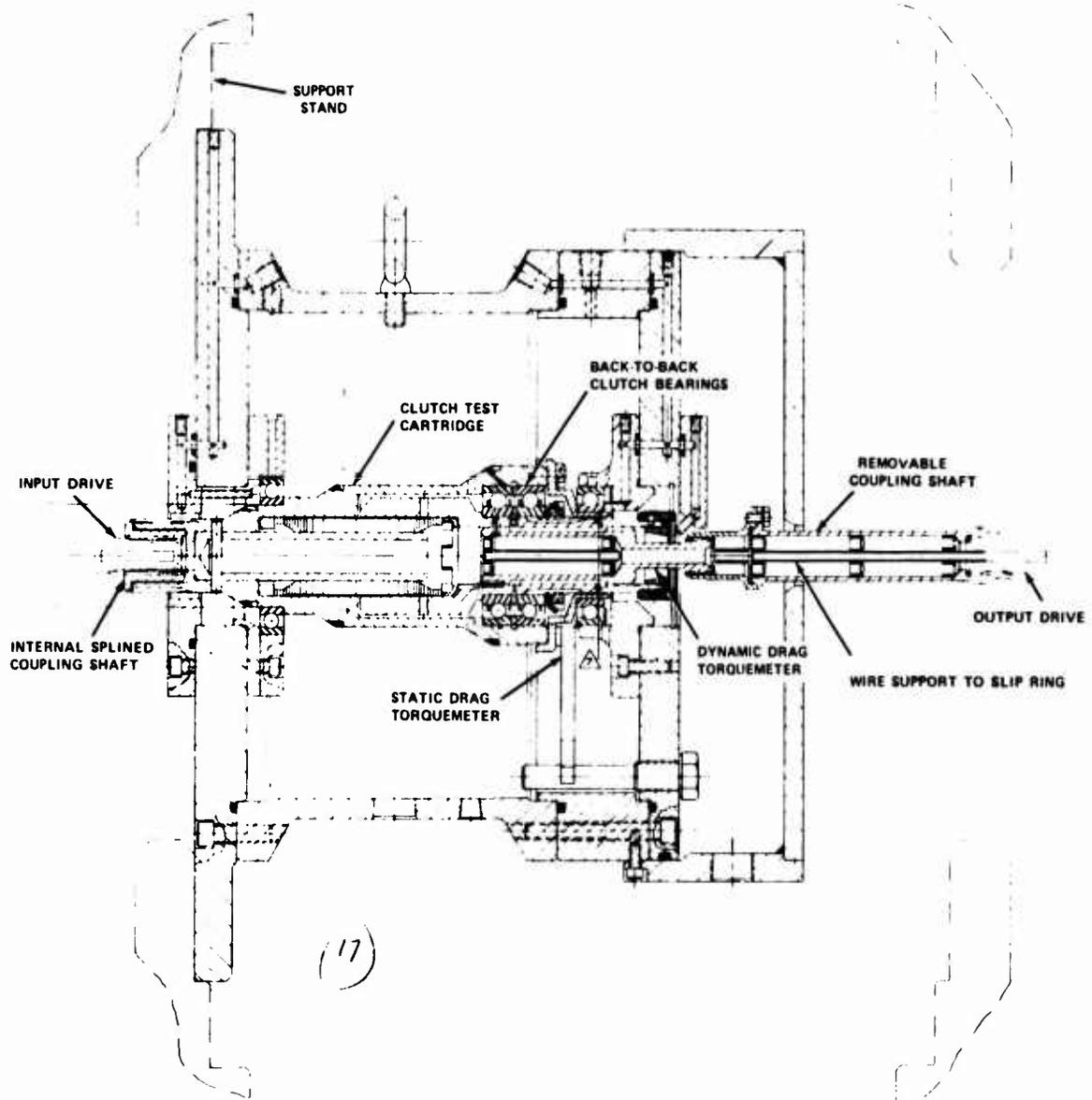
Figure 17. Design B, Test Cartridge Details.
