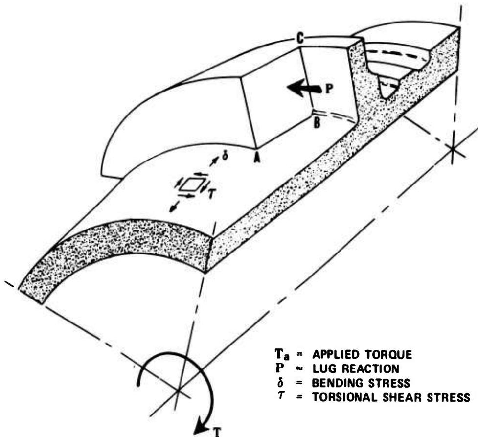
Figure 67. Inner Race, Spring Clutch Assembly.
