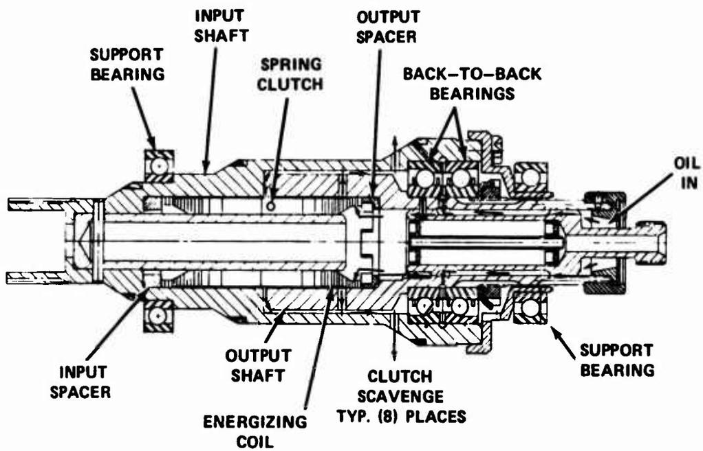
Figure 9. Lubrication and Scavenge Paths, Design B.
