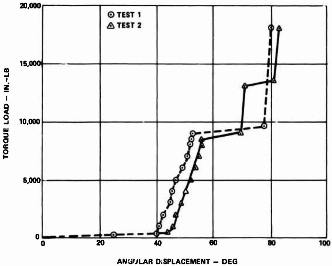
Figure 61. Angular Displacement of Output Shaft, Design B.
