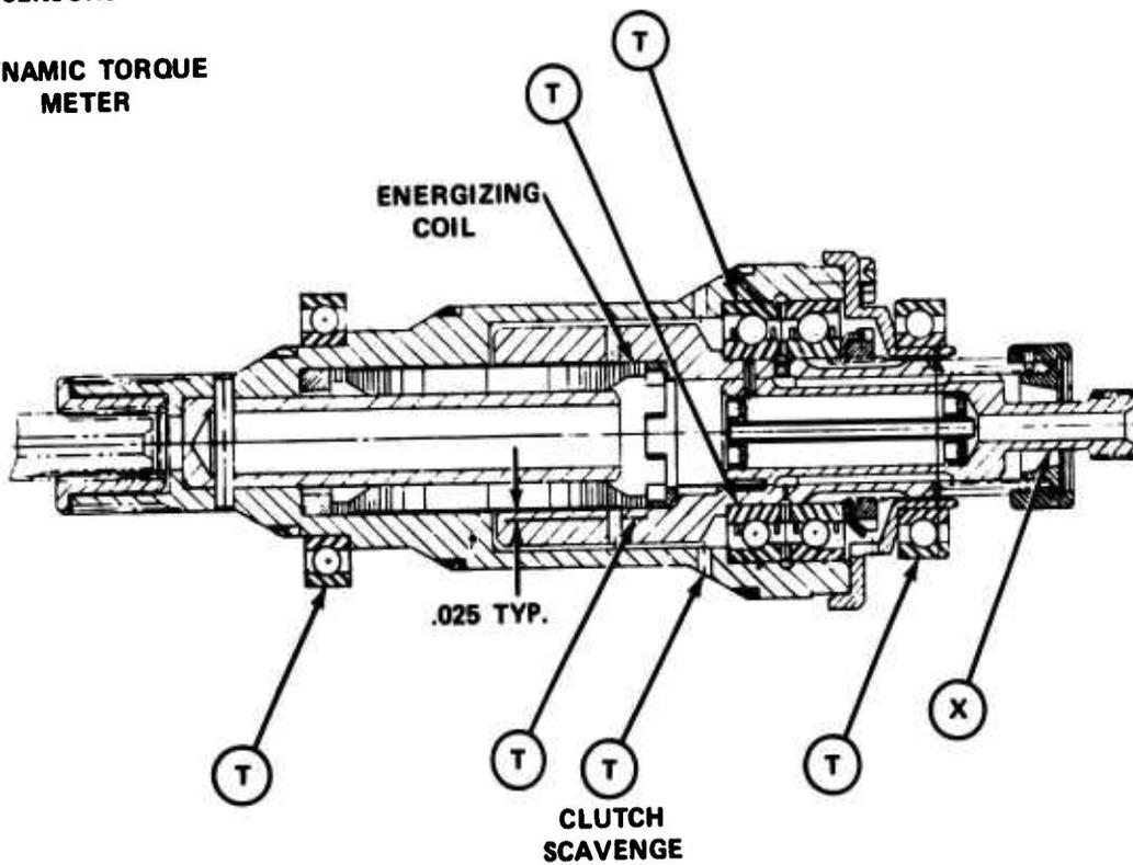
Figure 22. Design B, Instrumentation Schematic.
