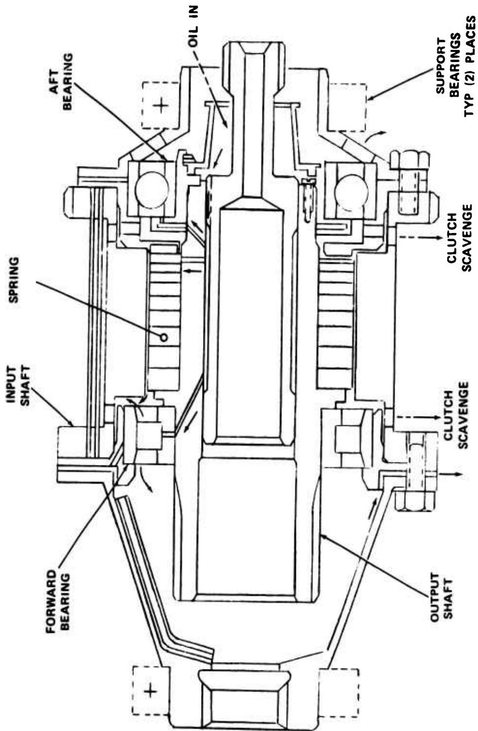
Figure 5. Lubrication and Scavenge Paths, Design A.
