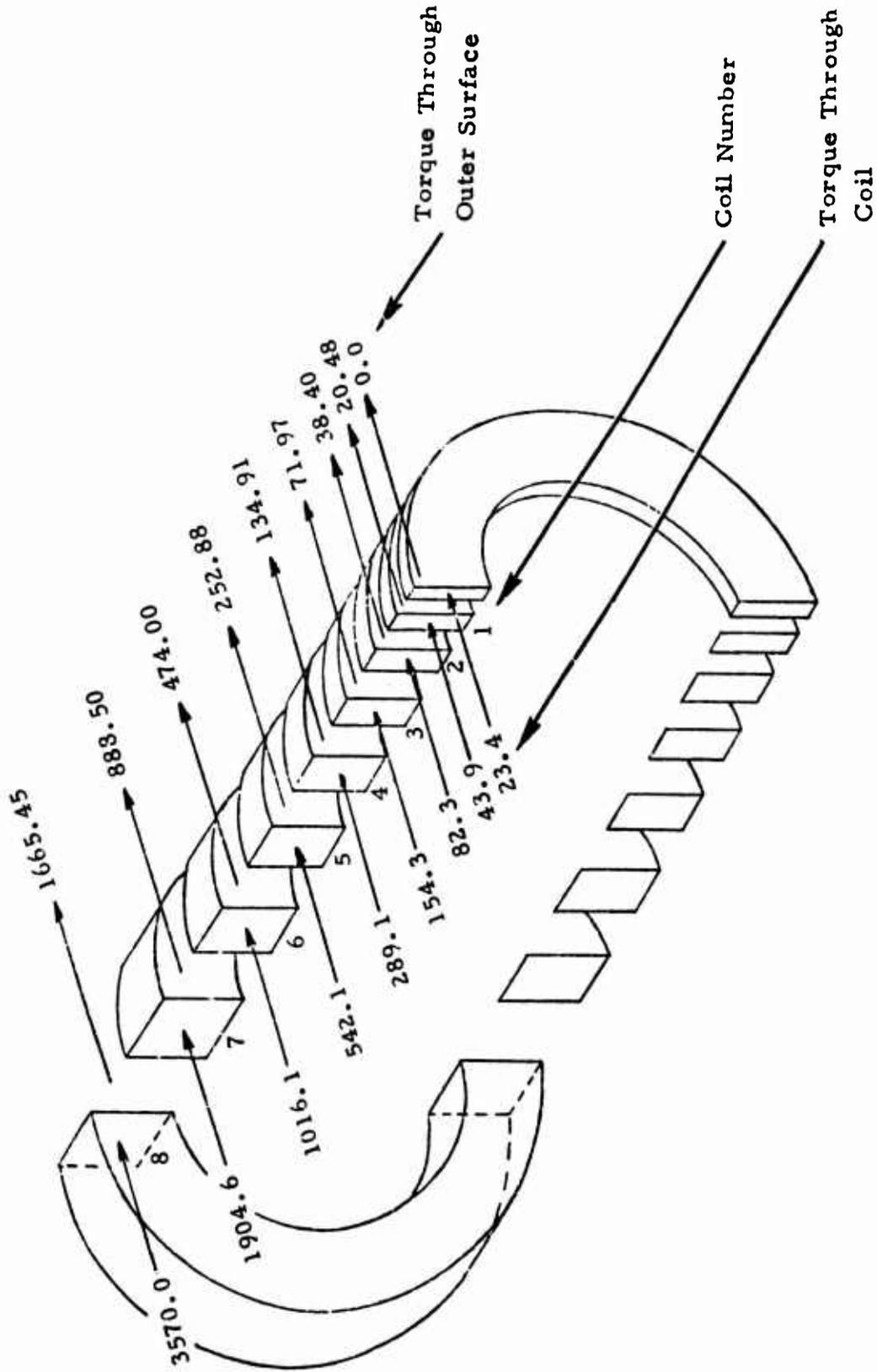
Figure 64. Torque Distribution Through Spring, Clutch Design A.
