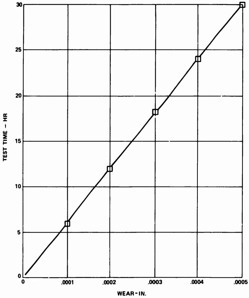
Figure 33. End Coil Wear Versus Test Hours, Design A.
