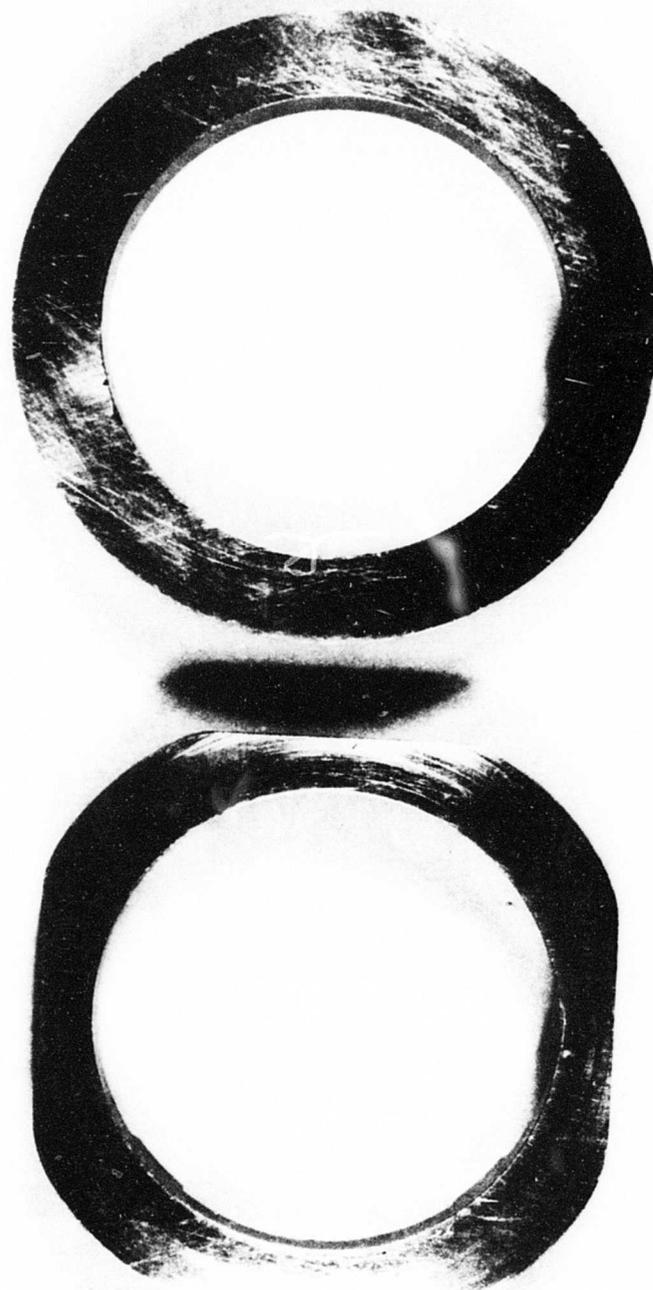
Figure 37. Design B Spacers Following Override Test.
