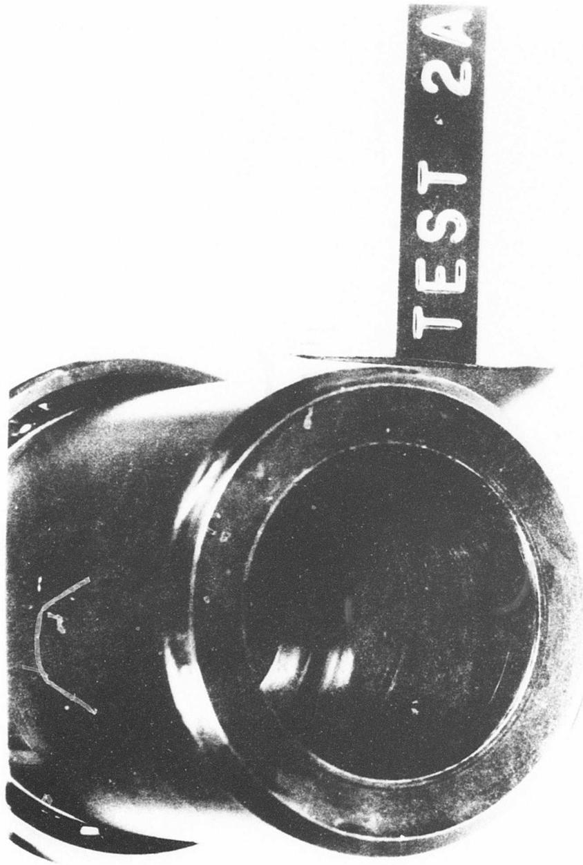
Figure 52. Design B Output Shaft Following Differential Speed Test.
