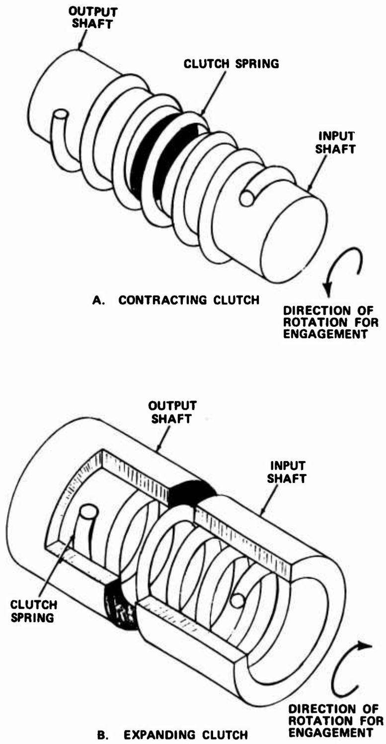
Figure 1. Principle of Spring Clutch Operation.
