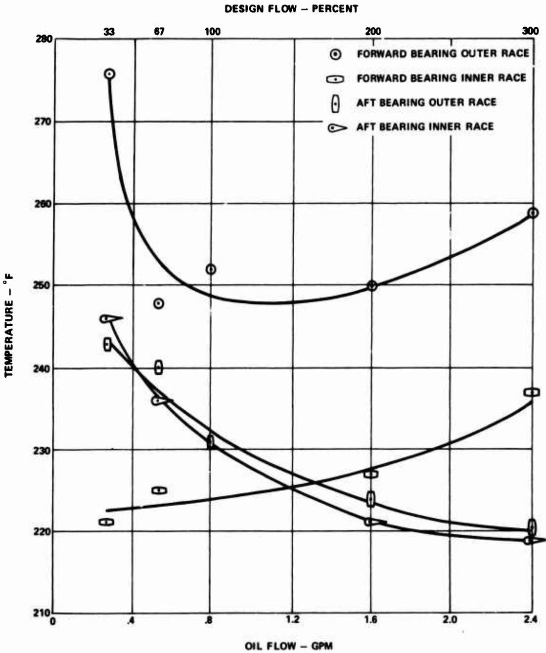
Figure 44. Bearing Race Temperatures Versus Flow, Design A.
