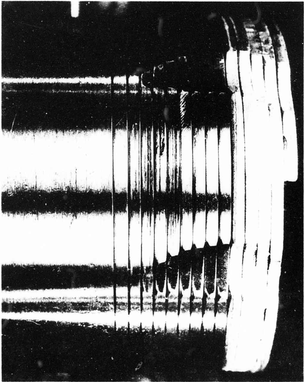
Figure 36. Design B Energizing Spring Following Override Test.
