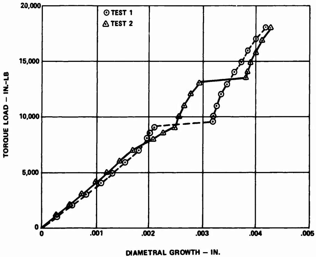
Figure 60. Diametral Growth of Output Shaft, Design B.
