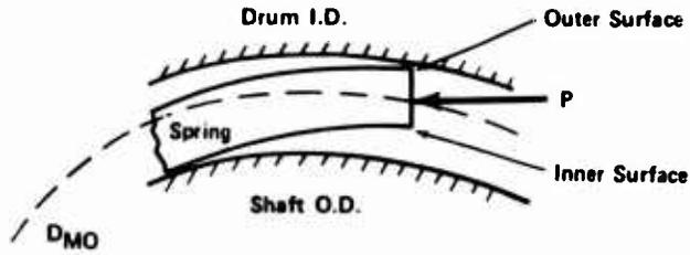
Spring stress due to load P consists of bending plus compressive stresses.
