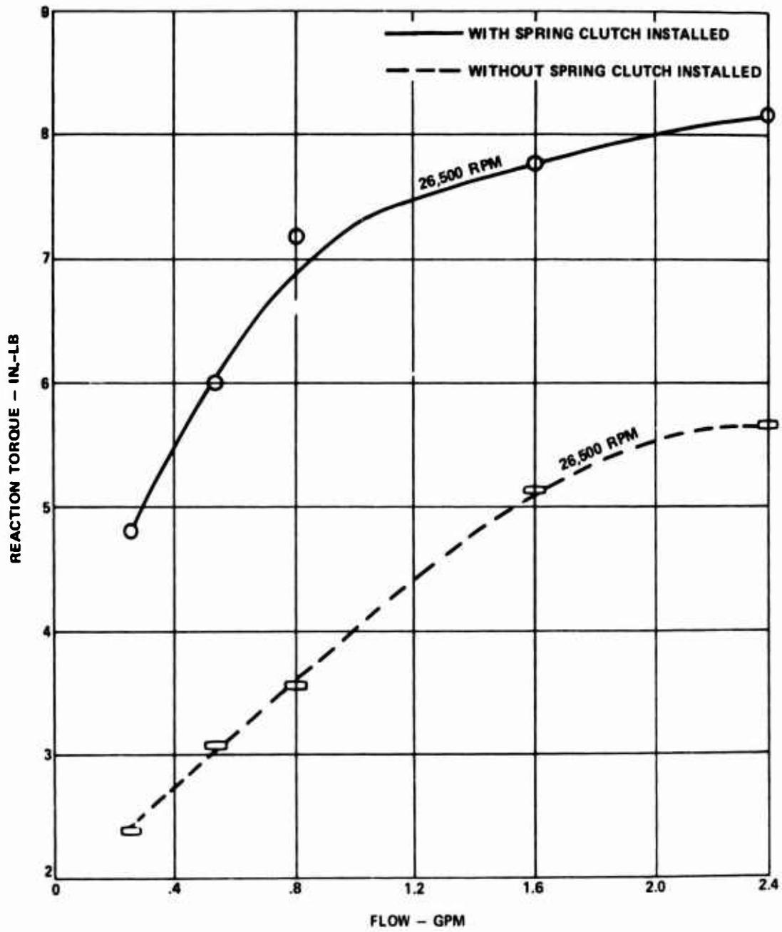
Figure 39. Reaction Torque Versus Oil Flow, Design B.
