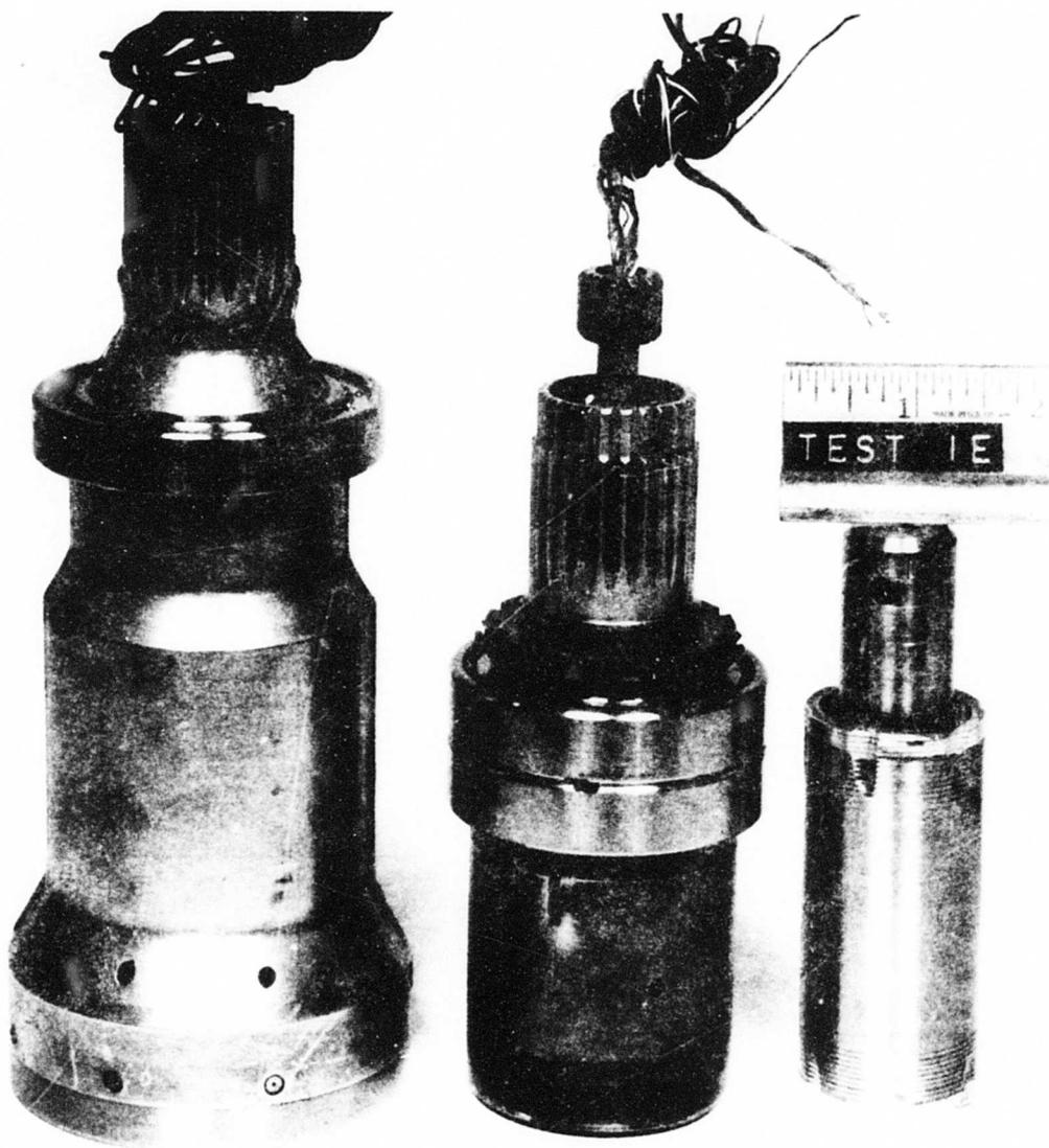
Figure 35. Design B Components Following Override Test.
