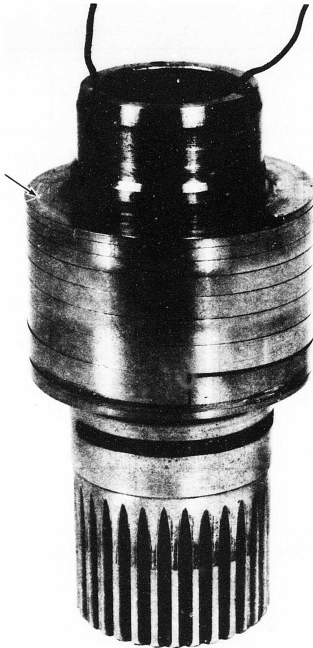
Figure 32. Spring Condition Following Override Test, Design A.
