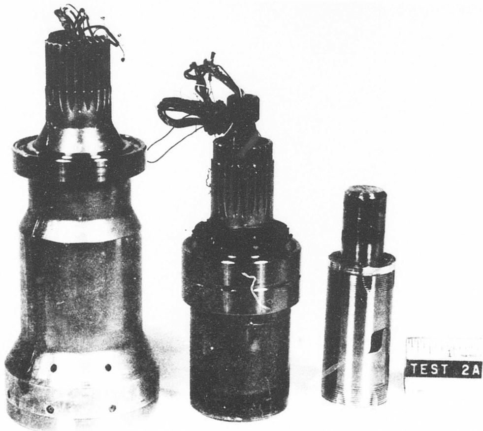
Figure 49. Design B Components Following Differential Speed Test.
