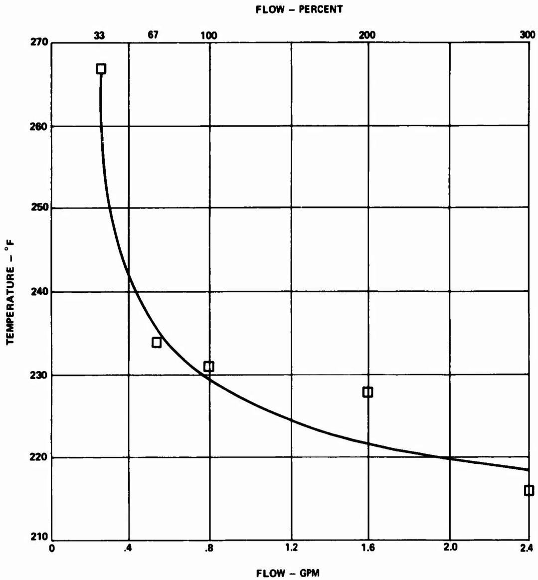
Figure 43. Energizing Coil Temperature Versus Flow, Design B.
