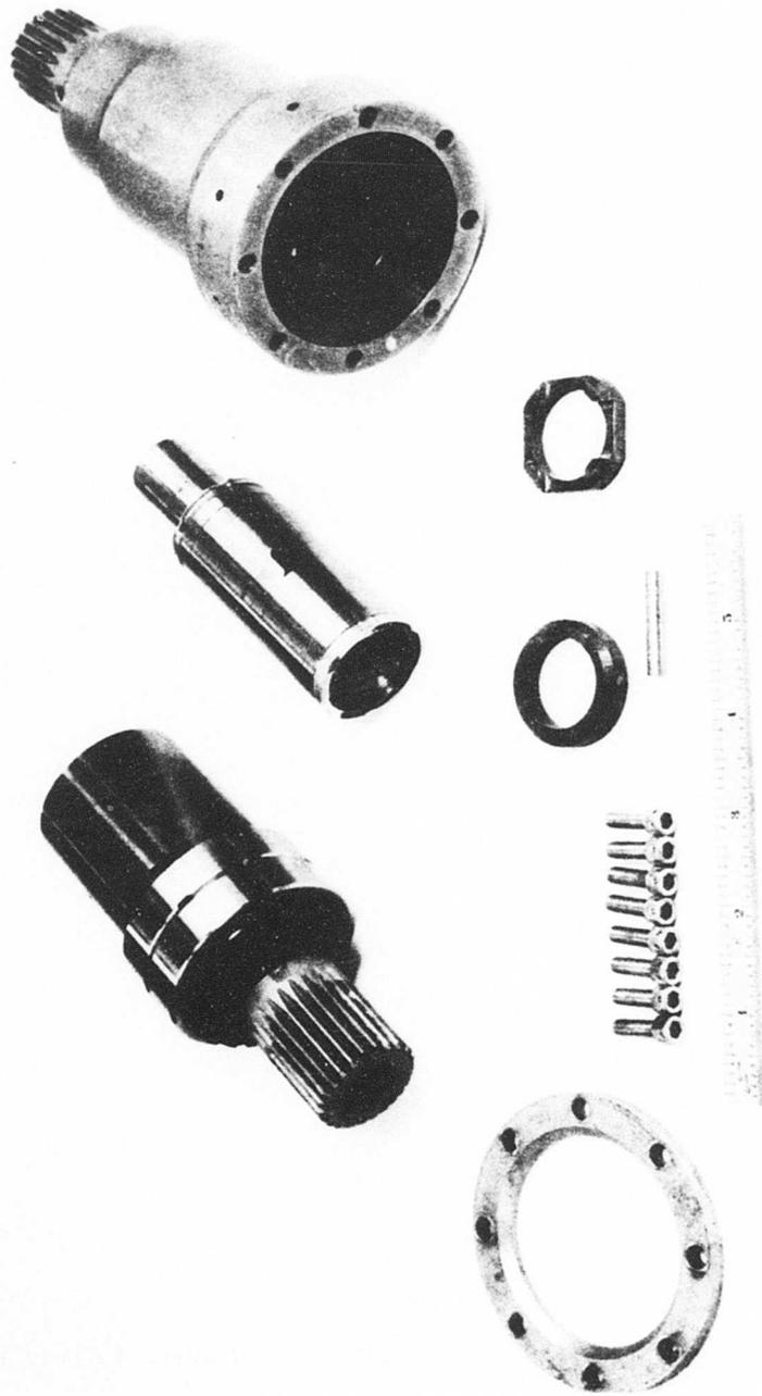
Figure 10. Clutch B Components.
