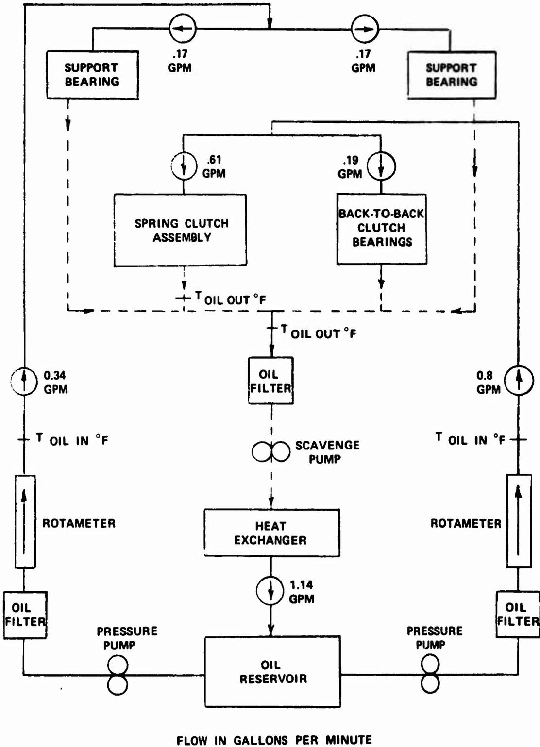
Figure 19. Design B, Lubrication Schematic.
