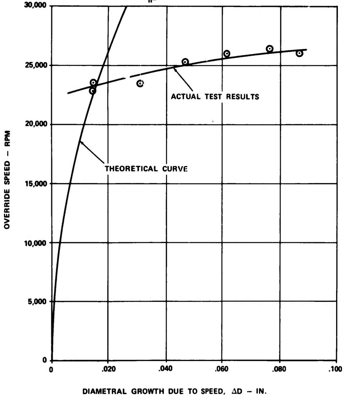
Figure 13. Override Speed Versus Diametral Growth, Design A.
