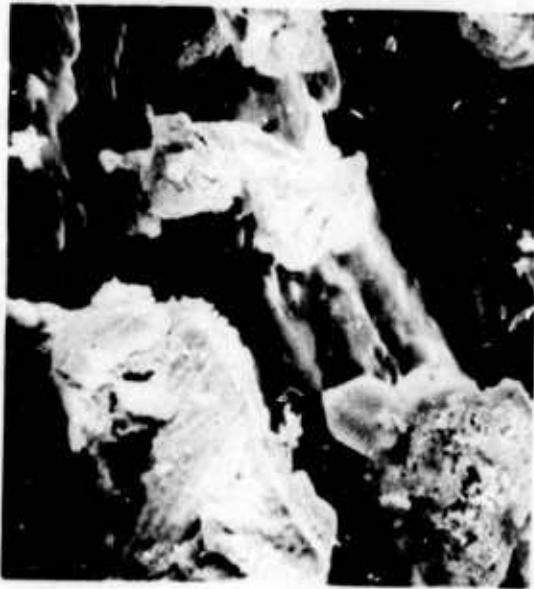
Figure 1 SEM photomicrograph of calcined powder prepared by the sulfate process. 4300X
