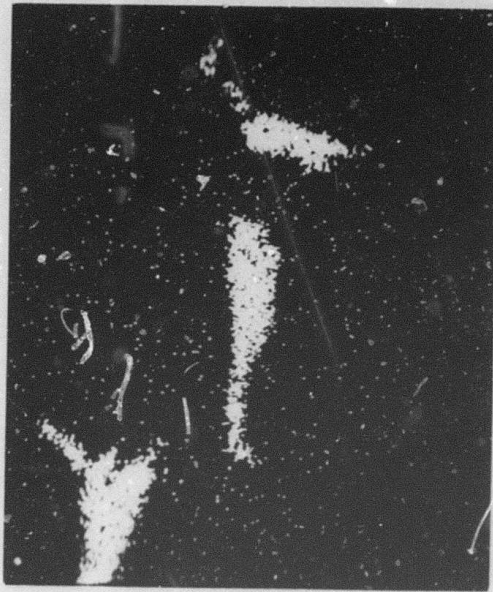
Figure 3 Electron probe, X-ray K_{\alpha} display of sulfur in the grain- boundary phase. 1088X
