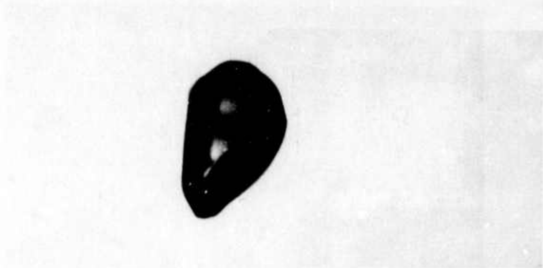
Figure 12 Large pore in sintered material prepared from ball-milled powder. Sintered 60 hours at 2170°C. Transmitted light. 270X
