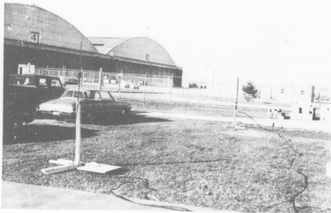
FIGURE 11: Photograph of the One Inch and Five Foot Monopoles - Mounted on Wooden Stands
