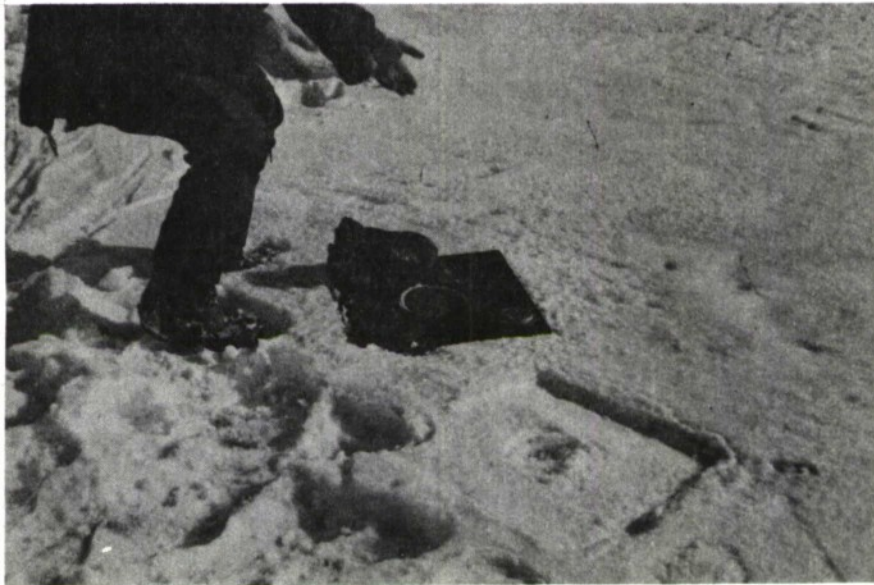
Figure 2-3. Load Bearing Test
