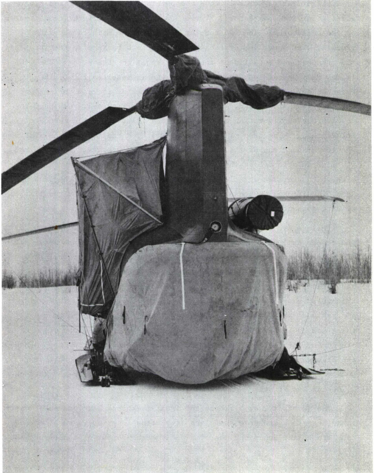
Figure 3.2 Engine and Cargo Ramp Shelters on Aircraft
